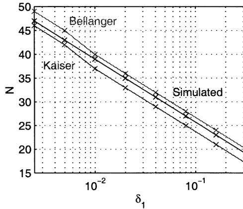
**Figure 4:** Order  $N$  as a function of ripple  $\delta_1$  ( $R_s=40$  dB and  $tr=0.05f_s$ ).
