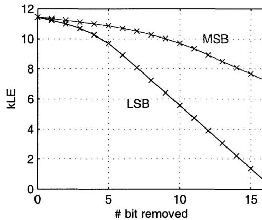
**Figure 8:** Number of Logic Elements (LE) as function of removed bits for Most Significant Bits and Least Significant Bits ( $kLE=1000 \cdot LE$ ).
