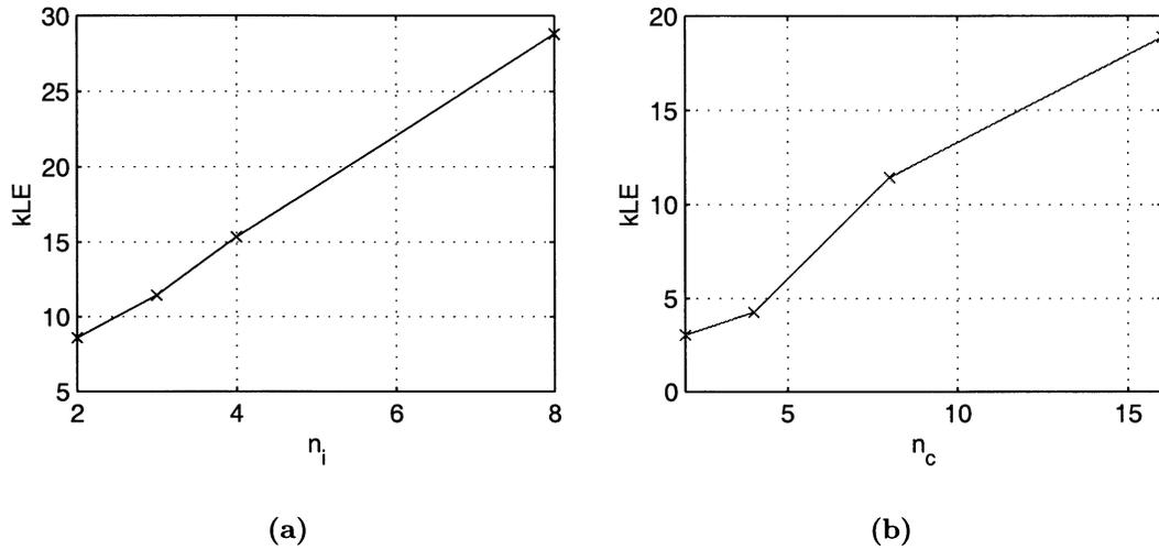
**Figure 9:** *Logic Elements as function of (a) input bits  $n_i$  and (b) coefficient bits  $n_c$  ( $kLE=1000 \cdot LE$ ).*
