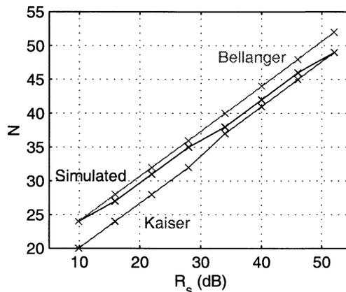
**Figure 5:** Order  $N$  as a function of attenuation  $R_s$  in dB ( $R_p=0.1$  dB and  $tr=0.05f_s$ ).
