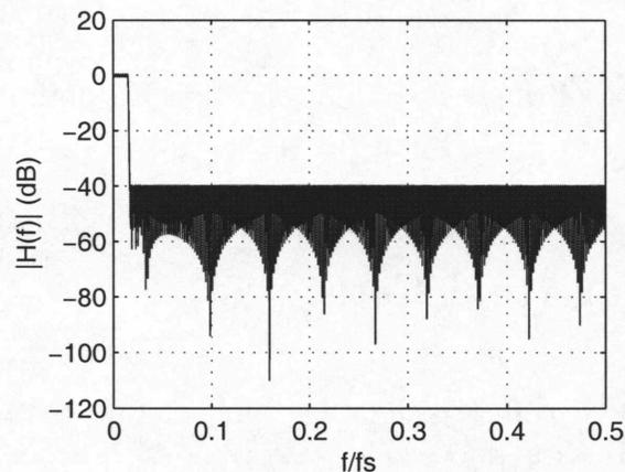
**Figure 7:** Frequency characteristic of small low pass filter with 10 percent transition region, 40 dB suppression and 1 dB ripple.
