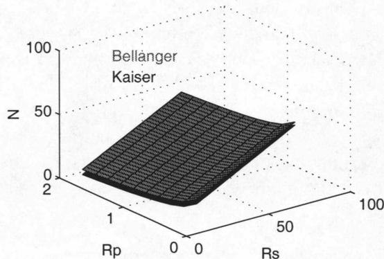
**Figure 6:** Order  $N$  as a function of ripple  $R_p$  and attenuation  $R_s$ , both in dB, for a transition region of  $0.05f_s$ .
