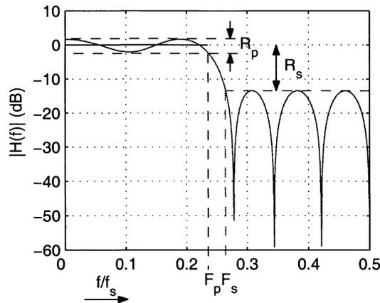
**Figure 1:** Definition of FIR filter quantities, with  $f_s$  the sample frequency.
