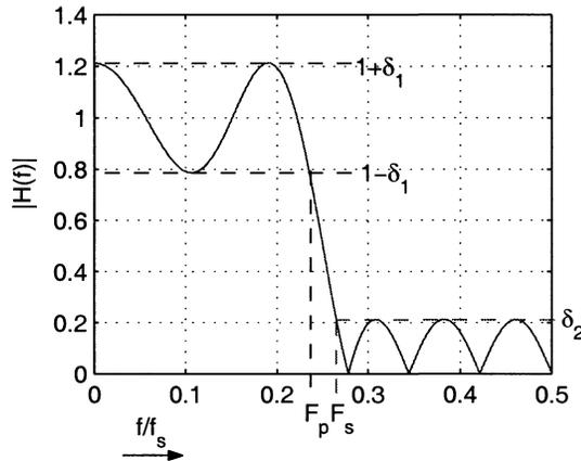
**Figure 2:** Definition of additional FIR filter quantities, with  $f_s$  the sample frequency.
