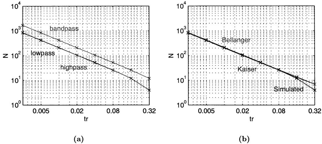
**Figure 3:** Logarithmic plot of order as a function of transition region (expressed in  $f_s$ ) for (a) lowpass, highpass and bandpass filter and (b) for lowpass filter obtained via simulation, Kaiser's approximation and Bellanger's approximation ( $R_p=0.1$  dB and  $R_s=40$  dB).
