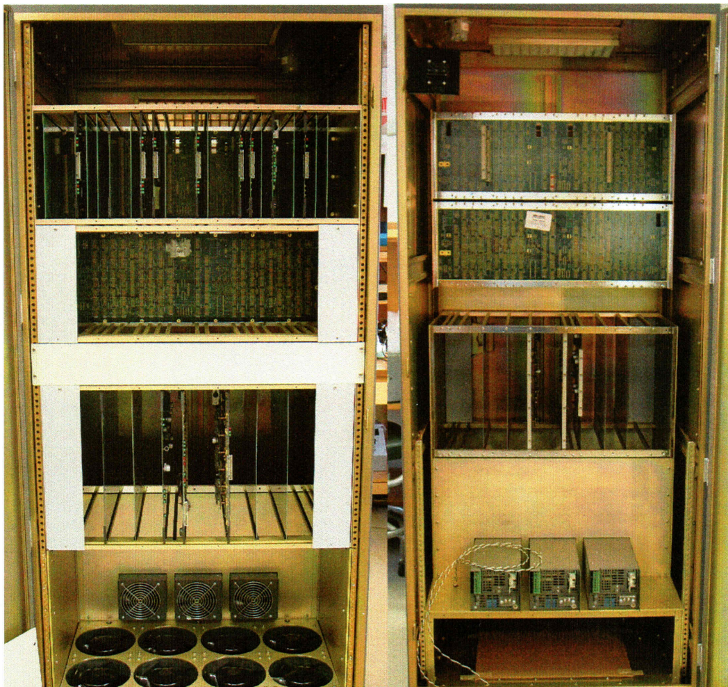
Front (left) and rear of prototype 2-antenna correlator rack showing card cages, cards, backplanes, fans, and power supplies mounted.
