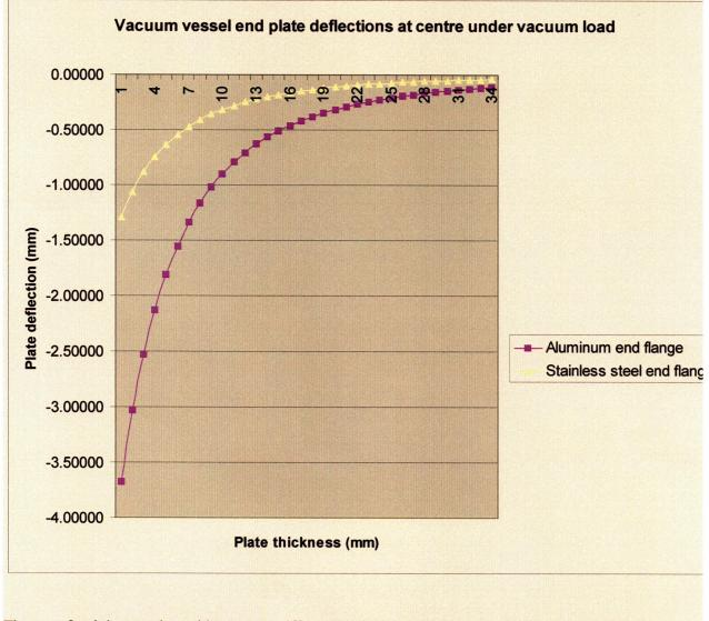
The use of stainless steel provides greater stiffness but there is a mass penalty using this material. I will calculate some revised mass estimates to quantify this.
