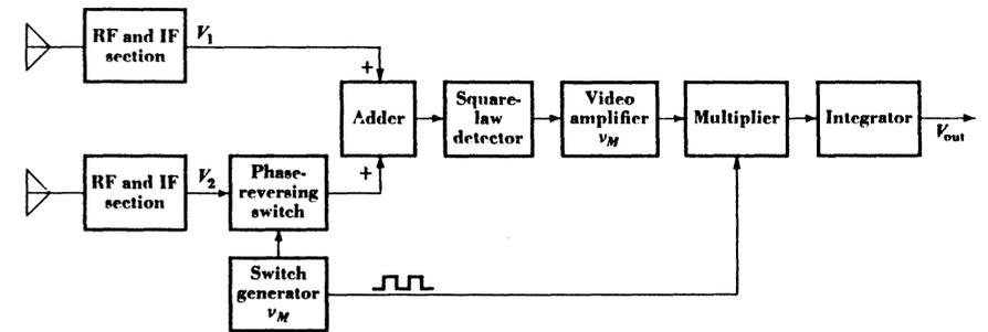
Fig. 7-20. Phase-switched receiver
