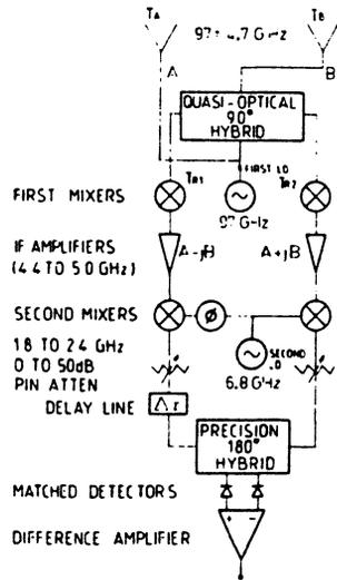
Fig. 1. Radiometer block diagram. The two inputs at temperatures of  $T_A$  and  $T_B$  are split and combined in a quasi-optical hybrid. After mixing at 97 GHz, they are amplified and phase shifted to optimize the response. A precision  $180^\circ$  hybrid and matched detectors are used to "multiply" the two IF signals.
