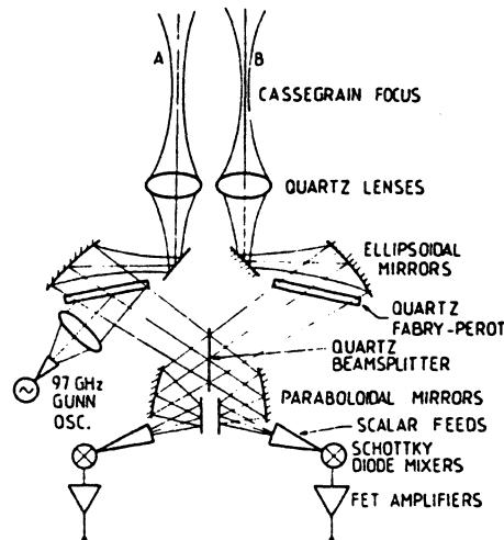
Fig. 2. Radiometer optics diagram. The symmetrical system uses fused-silica lenses to focus the inputs from the Cassegrain focus into the cryogenic Dewar. A thin sheet of fused-silica acts as a  $90^\circ$  hybrid. Then the 97-GHz LO is injected via a dielectric Fabry-Perot and the beams are refocused into the millimeter mixers.
