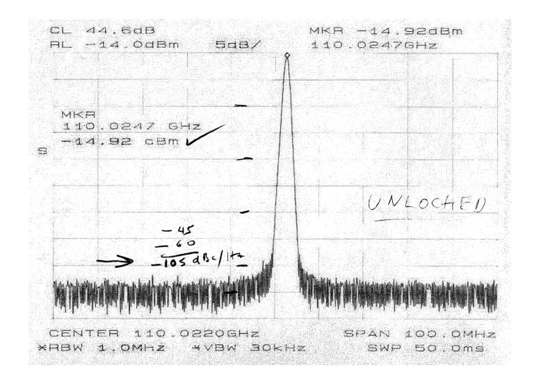
Figure 4: Output spectrum from laser heterodyne and u2t photomixer at 110 GHz
