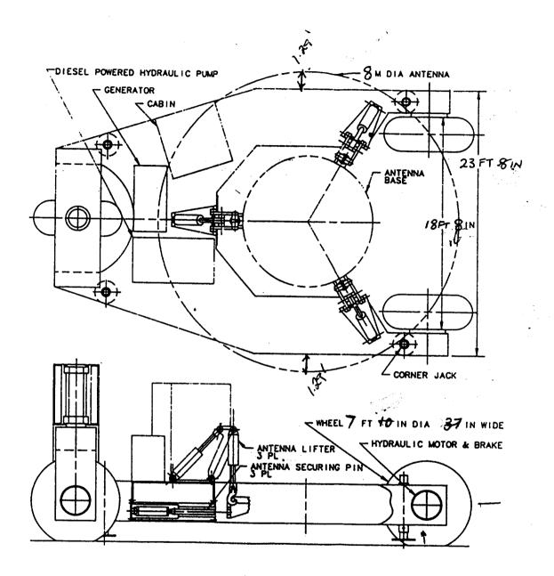
Mechanical interface between the antenna and the transporter.
