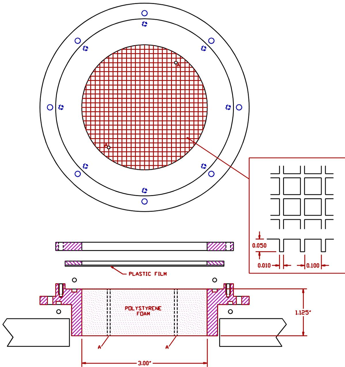
Fig. 6. Construction of the broadband vacuum window. The plastic film vacuum barrier is supported by the polystyrene foam plug. The small through holes "A" (1/16" dia.), connected to the grid of grooves in the upper surface of the foam, ensure that any gas molecules permeating the vacuum barrier are pumped away and do not condense at a cold region inside the foam.
