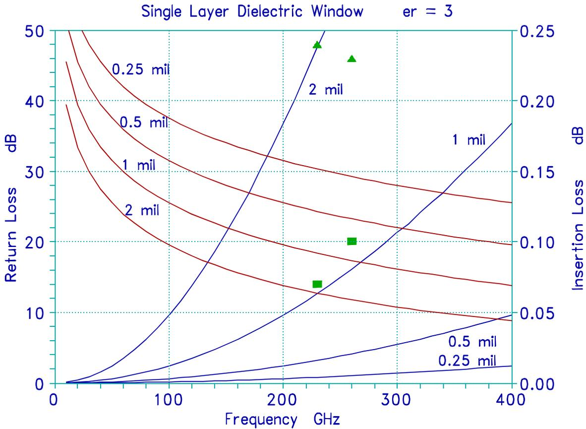
Fig. 1. Theoretical return loss and insertion loss vs. frequency for dielectric sheets with  $\epsilon_r = 3$  and thickness 0.00025", 0.005", 0.01", and 0.002". The points  $\square$  and  $\triangle$  are the measured insertion loss for 0.001" and 0.002" mylar.
