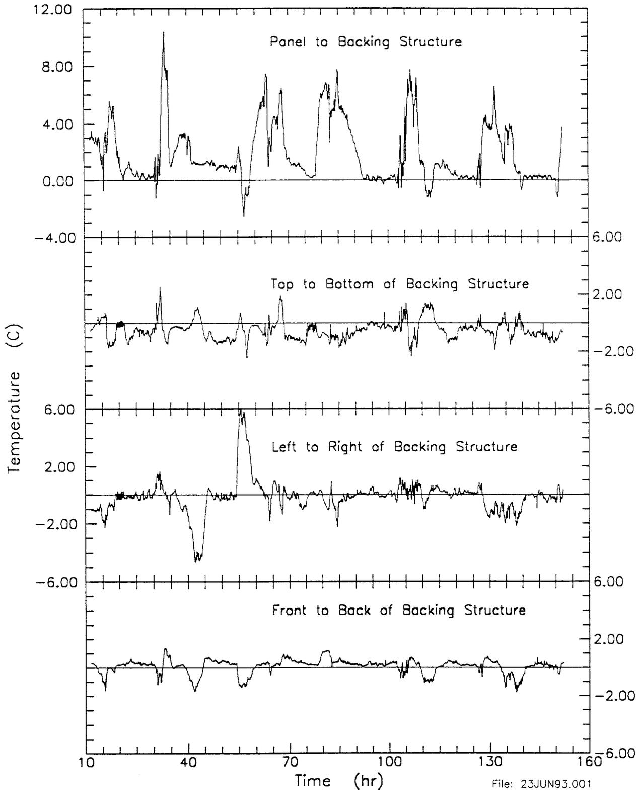
Figure 5. Differences between parts of the BS for 23<sup>rd</sup> June 1993 data, fans and sunshades off.
