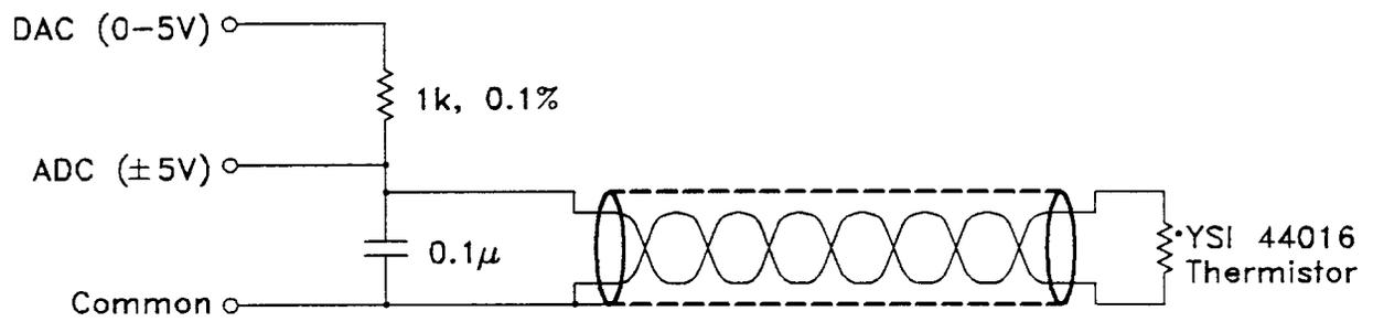
Figure 2. Circuit used to supply current to thermistors and read voltages.
