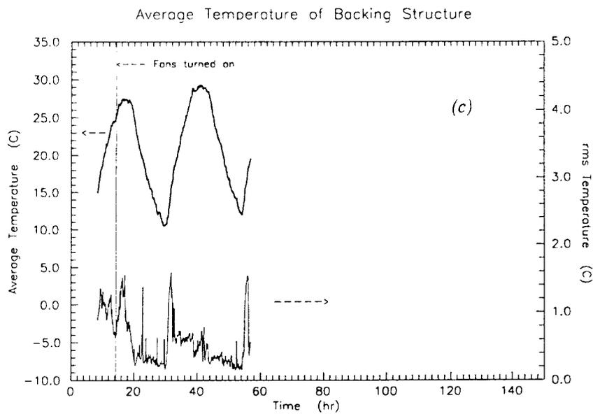
Figure 3. Average temperature in the backing structure, and rms variation of sensor readings from the mean.
