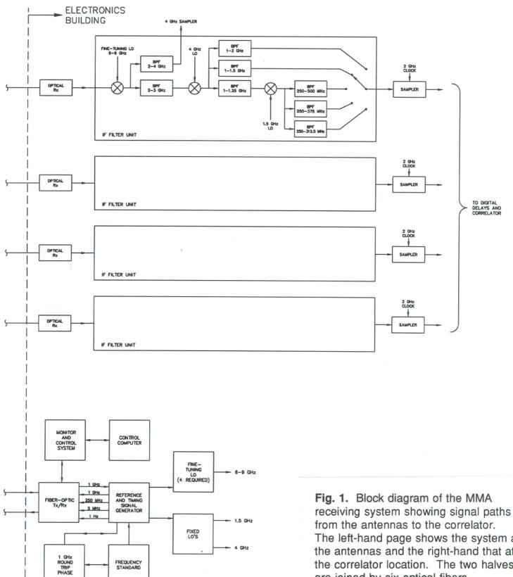
receiving system showing signal paths The left-hand page shows the system at the antennas and the right-hand that at the correlator location. The two halves are joined by six optical fibers.
