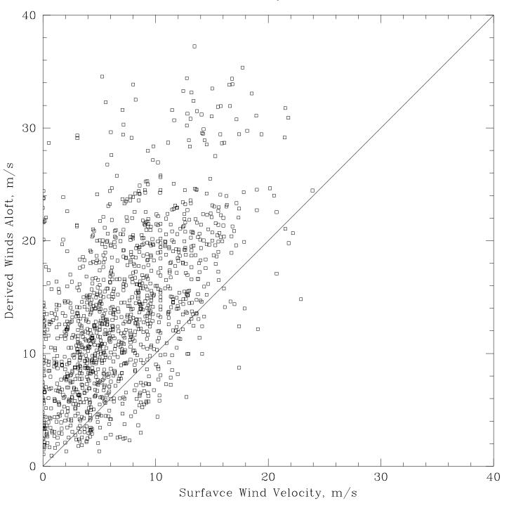
Figure 2: Derived velocity of the winds aloft as calculated from the scaling between the spatial and temporal structure functions, plotted against the surface wind velocity measured at our weather station.
