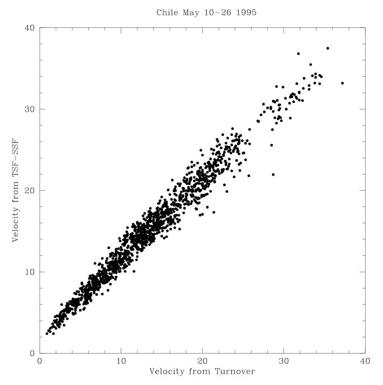
Figure 1: Derived velocity of the winds aloft as calculated from the scaling between the spatial and temporal structure functions, plotted against the velocity calculated from the temporal structure function turnover and simulations.
