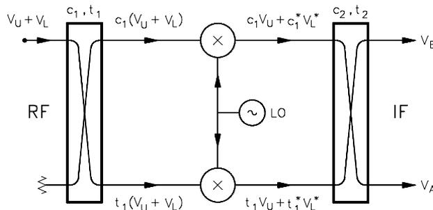
**Fig. 7. Signal flow through the image separating mixer. For simplicity, the mixers are assumed to have unit conversion gain.  $V_U$  and  $V_L$  are the complex amplitudes of the incident USB and LSB signals.**
