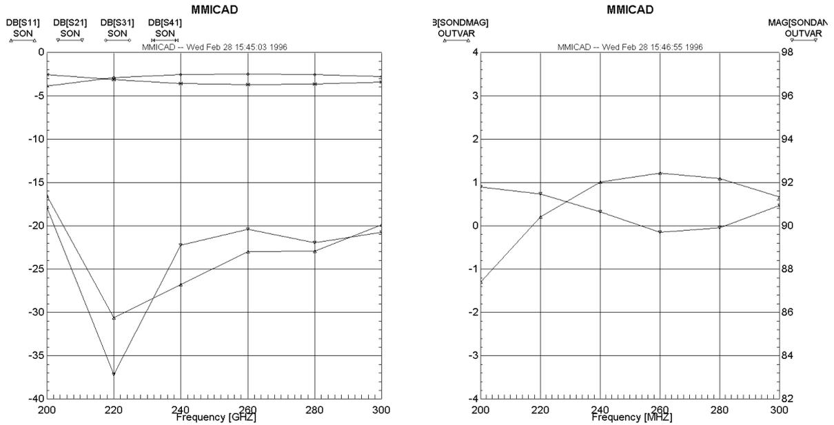
Fig. 11. S-parameters of the quadrature hybrid from Sonnet *em* simulation.
