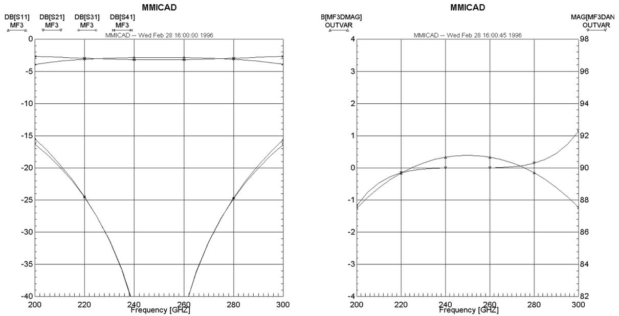
Fig. 10. S-parameters of the quadrature hybrid after optimization of the circuit model.
