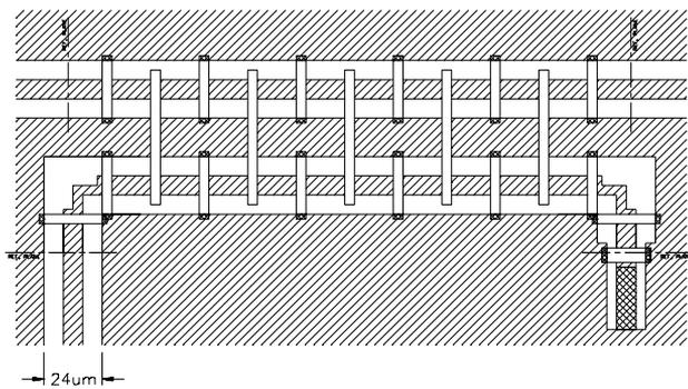
Fig. 13. The LO coupler. The five long vertical strips couple capacitively between the two CLCPW's.
