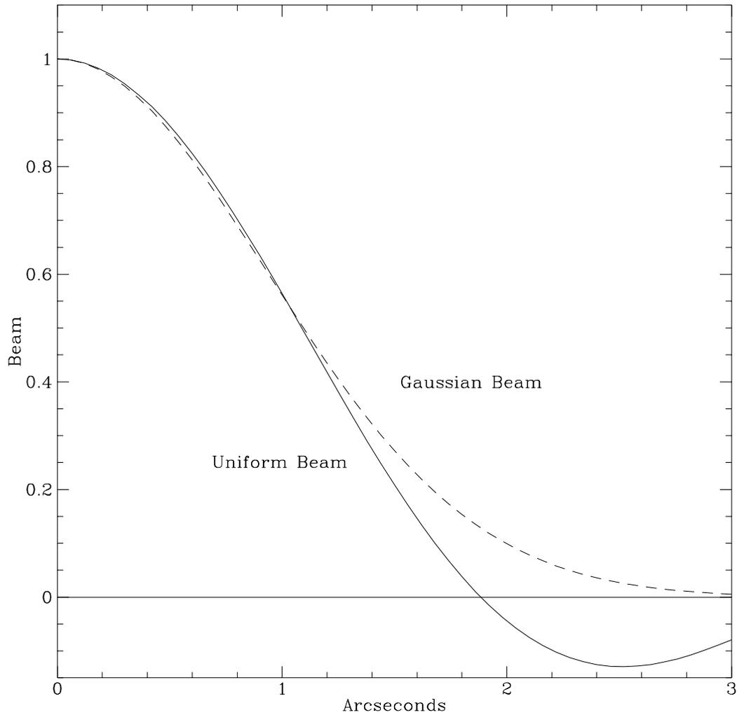
Figure 5: What's wrong with the uniform distribution's beam? Here are the radial profiles of the naturally weighted uniform Fourier distribution's beam and its best fit Gaussian. The uniform Fourier distribution has much too many long baselines to yield a good Gaussian beam. Conversely, in order to get a good Gaussian beam, the long baselines need to be tapered down, resulting in a loss of about 30% of the sensitivity.
