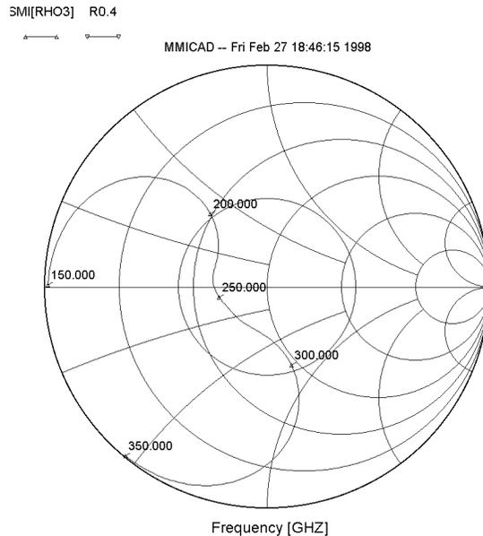
**Fig. 4. RF embedding impedance seen by the array. The junction capacitance is taken as part of the embedding circuit. The circle is at  $|\rho| = 0.4$ . (The Smith chart is normalized to the optimum source impedance.)**
