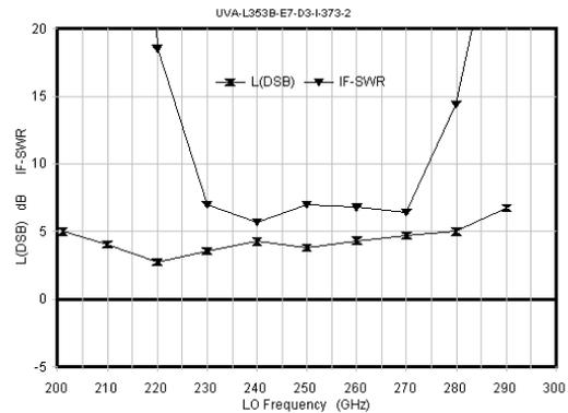
**Fig. 8. DSB conversion loss (lower curve) and IF port VSWR.**
