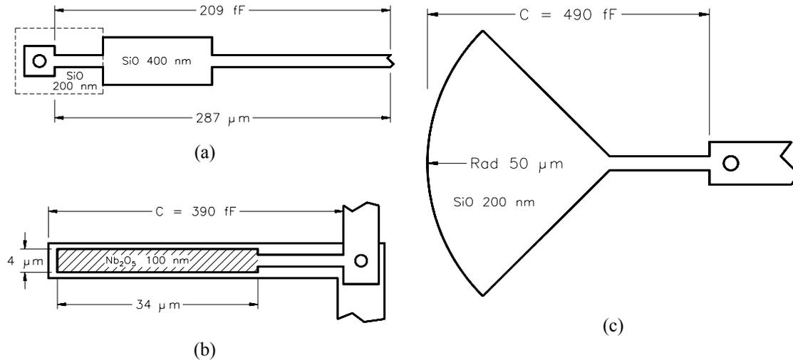
**Fig. 1. Three RF tuning circuits used in SIS mixers. Dimensions and capacitances indicated are for a center frequency of ~230 GHz. (a) End loaded matching circuit. (b) Tuning inductor with  $\lambda/4$  microstrip stub. (c) Tuning inductor with radial microstrip stub. (Diagrams not to scale.)**
