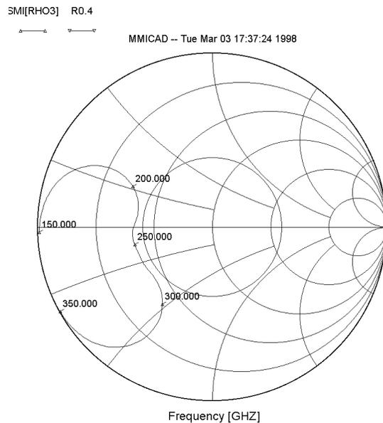
Fig. 6. RF embedding impedance seen by the array. The junction capacitance is taken as part of the embedding network. The circle is at  $|\rho| = 0.4$ . The Smith chart is normalized to the optimum source impedance (74 ohms).
