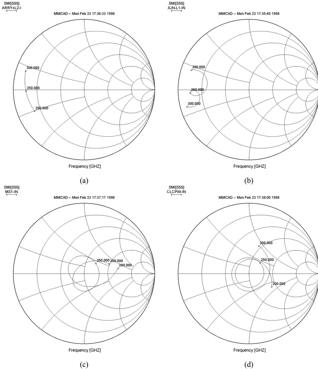
**Fig. 3. RF impedance transformation through the broadband matching network. (a) Impedance of the array of junctions and capacitor  $C_A$ , (b) including the two stubs, (c) including MS1 and CPW1, and (d) including the CLCPW input line. All Smith charts are normalized to 50 ohms.**
