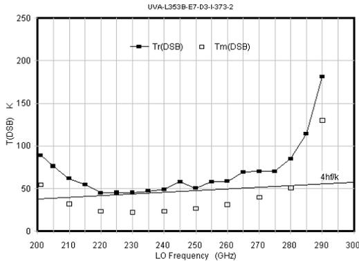
**Fig. 7. DSB receiver noise temperature (solid line) and mixer noise temperature (open squares). Shown for reference is the line  $4hf/k$ .**
