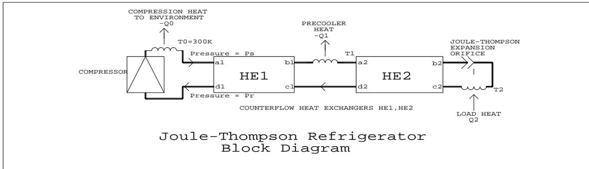
Figure 1. Block diagram of J-T refrigerator, showing the notation used in the text.
