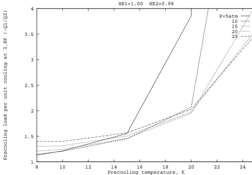
Figure 6. Precooling power per unit cooling at 3.8K, vs.  $T_1$  and  $P_s$ , with ideal heat exchangers.
