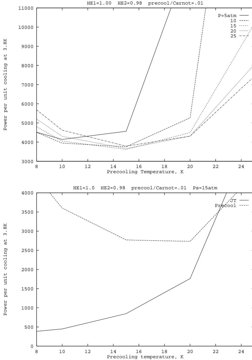
Figure 3. Like Fig. 2, but with HE2 efficiency reduced to 98%.
