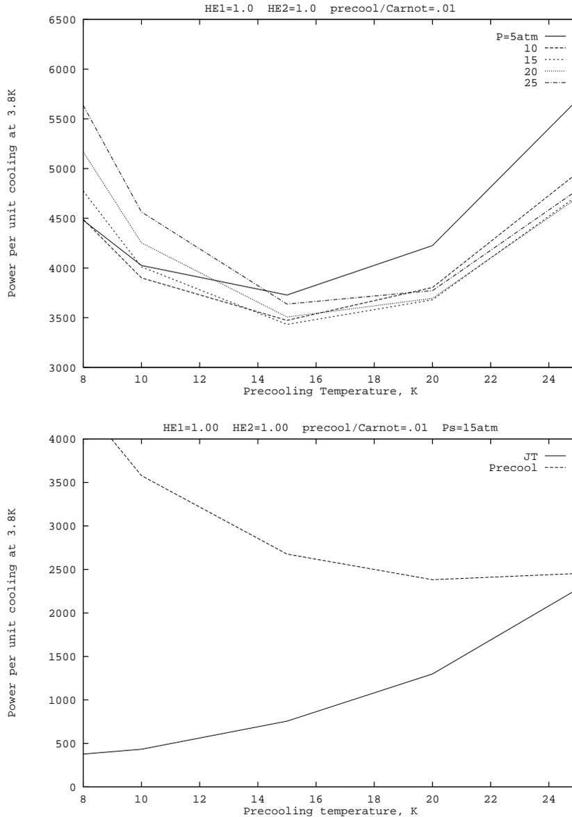
Figure 2. (a): Top. Total work per unit cooling at 3.8K, vs. precooling temperature and supply pressure, with ideal heat exchangers and with precooling efficiency typical of a small Gifford-McMahon refrigerator. (b): Bottom. Work per unit cooling for precooler and J-T compressor separately, at fixed supply pressure.
