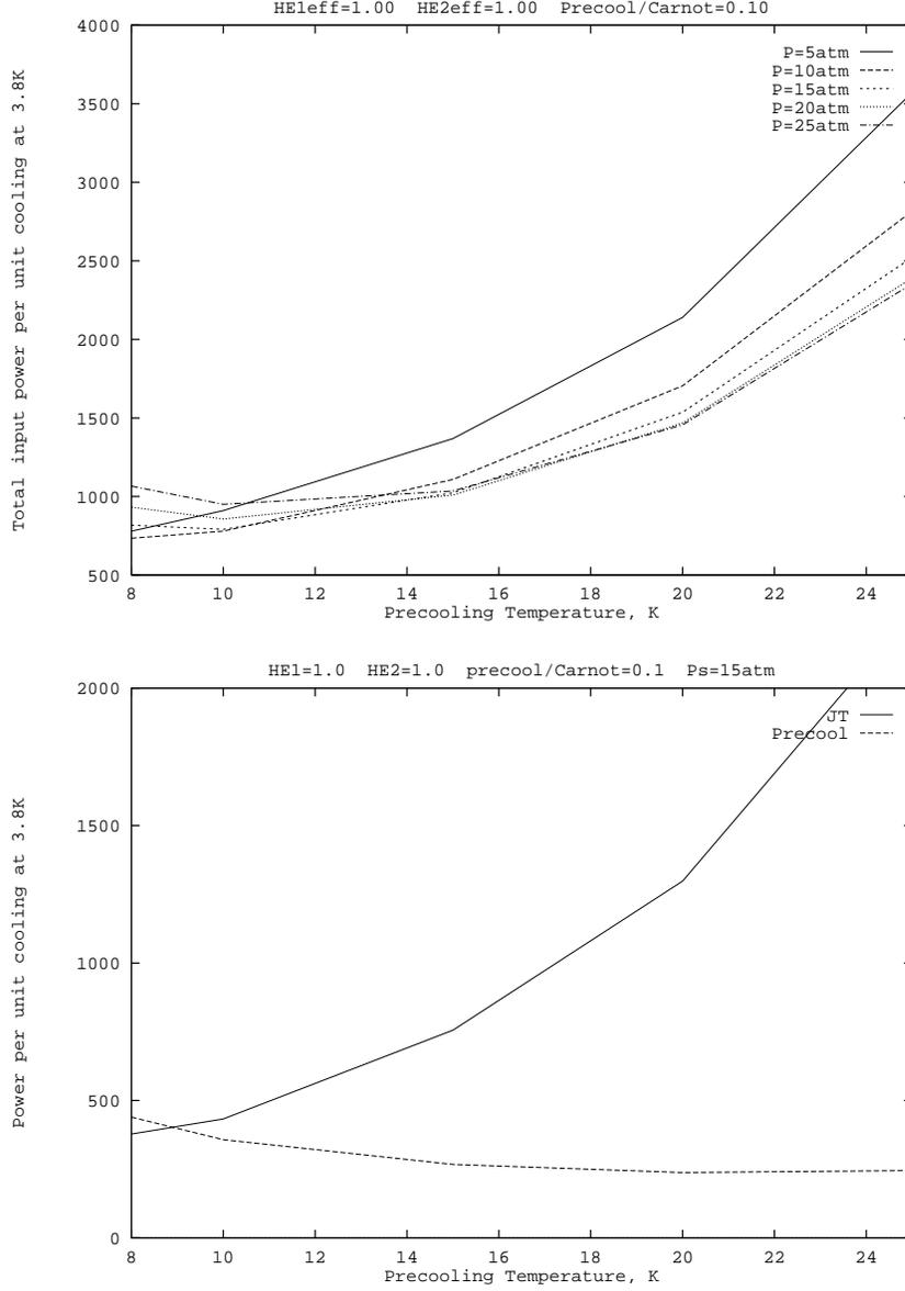
Figure 5. Like Fig. 2, but with a substantially more efficient precooler, typical of a small Sterling refrigerator.
