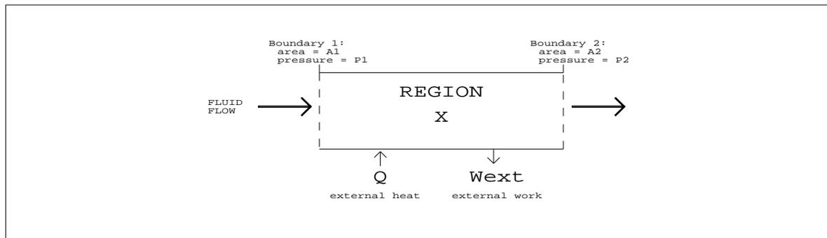
Figure A1. Illustration of the notation used to explain the concepts of enthalpy and flow work.
