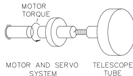
Figure 1. Simple model of antenna structure.
