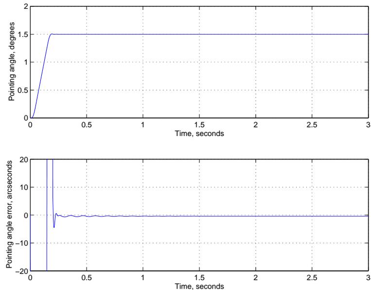
Figure 13. Responses for a system with tachometer loop only. The velocity profile of Figure 12 has been applied as input. The upper curve is load position, and the lower curve is load position from which the position profile of the lower curve of Figure 12 has been subtracted and appropriately scaled. No ringing occurs in spite of the short transition time.
