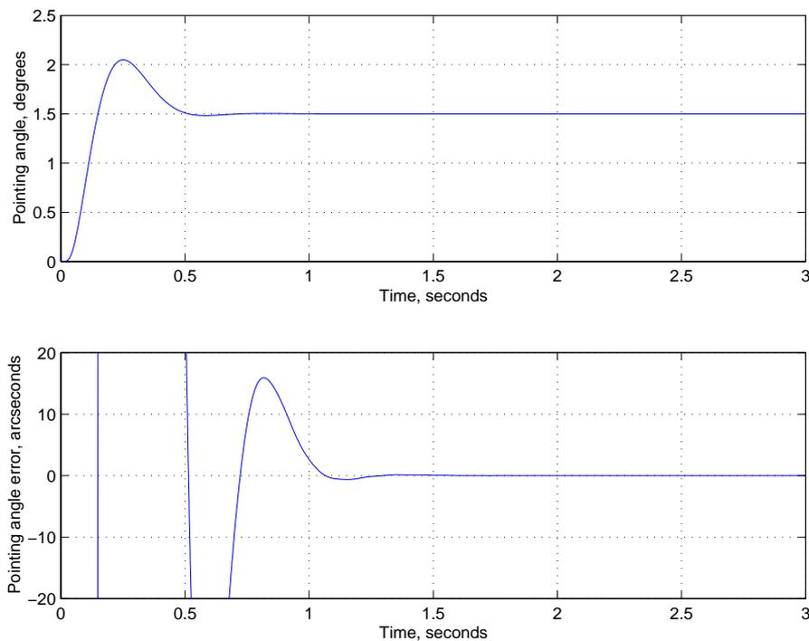
Figure 10. Step responses for a system with position feedback from the motor. The curves above show the movement of the load. The input curve is shown in Figure 11. Ringing is completely avoided.
