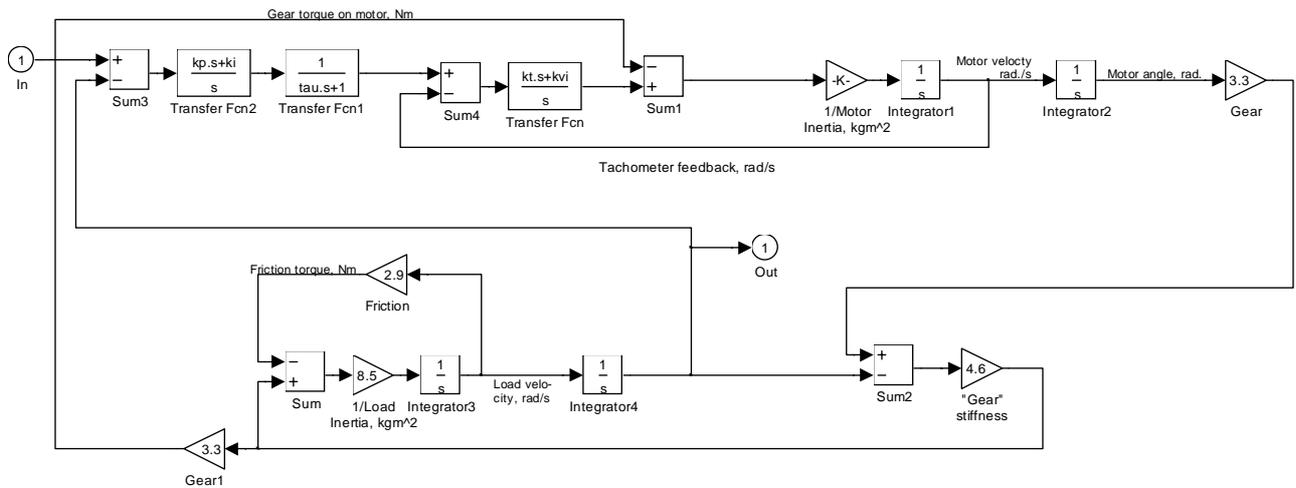
Figure 7. Block diagram of complete, linear model applied for this study. The diagram is shown with position feedback from the load. Alternatively, the feedback can be taken from the motor shaft.
