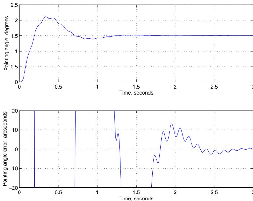
Figure 8. Step response of complete system. Encoder feedback is here taken from the load. It can be seen that the system is inherently too slow and that ringing is not critical.
