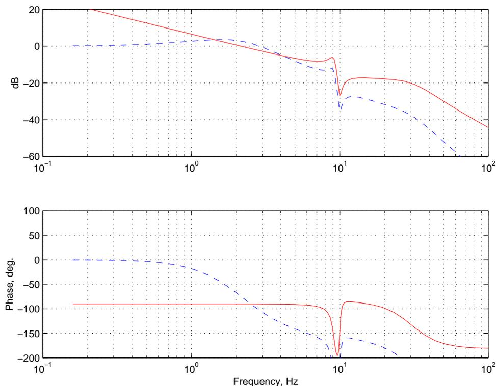
Figure 6. Open and closed loop frequency responses for the position loop. Encoder feedback is taken from the motor shaft. The open loop responses are solid and the closed loop plots dashed.
