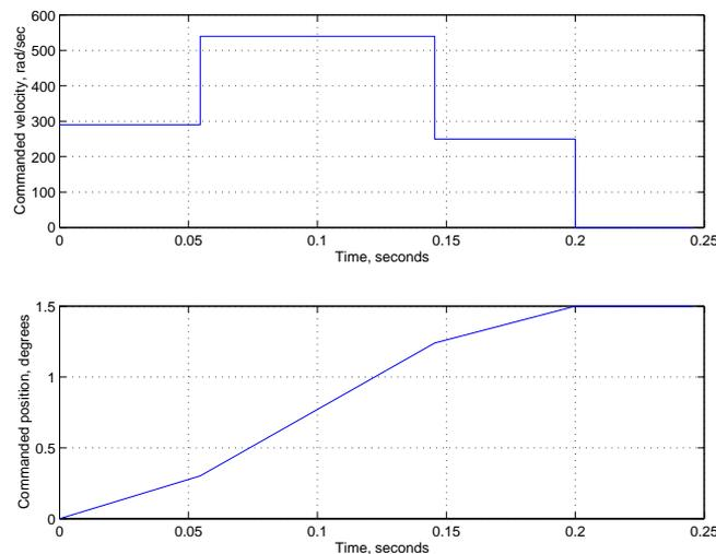
Figure 12. Shaped input curves for velocity (top) and position (bottom).
