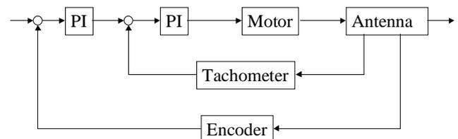
Figure 3. Overview of a conventional servo system for radio and optical telescopes. Compensation networks and current loop are not shown.
