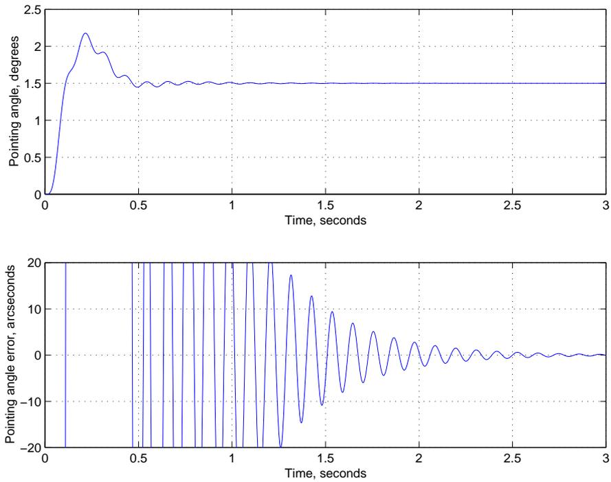
Figure 9. Step responses for a system with position feedback from the motor. The curves above show the movement of the load. Intense ringing occurs.
