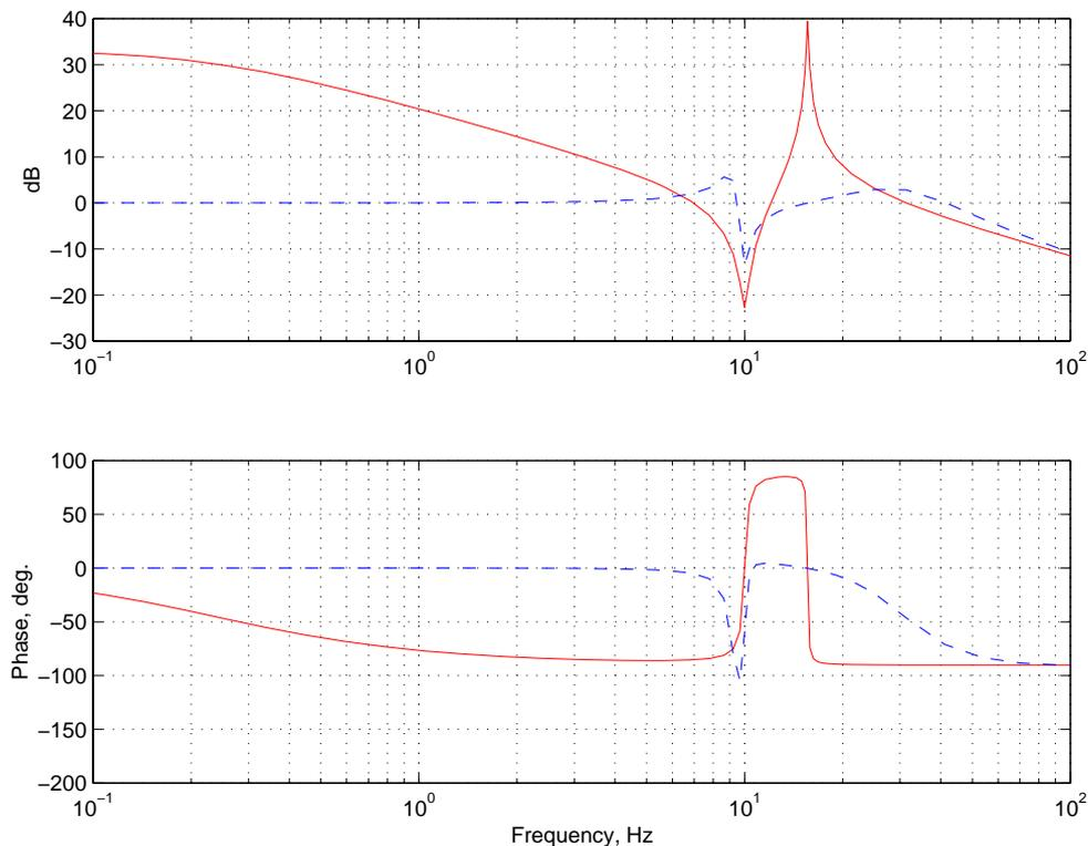
Figure 4. Bode plots for open and closed tacho loops, respectively. The open loop curves are solid, and the closed loop dashed.
