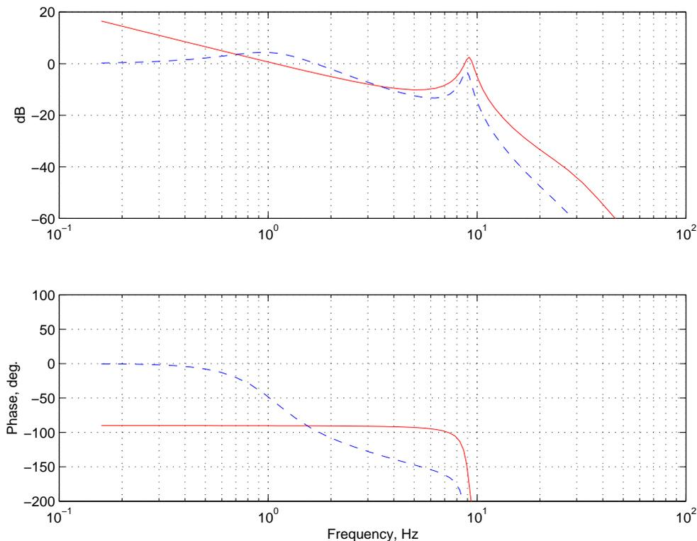
Figure 5. Open and closed loop frequency responses for the position loop. Encoder feedback is taken from the load. The open loop responses are solid and the closed loop plots dashed.
