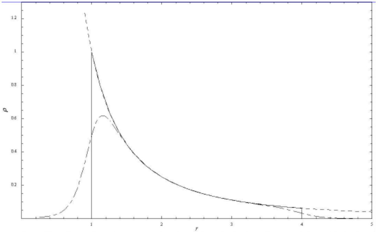
Figure 2: The beam profiles of hybrids consisting of two concentric rings of antennas, the outer with 4 times the diameter of the inner. The top curve is the profile when all the antennas are on the inner ring, the next when 20% of the antennas are on the outer, then 40, 60 80 and finally 100 %. Successive curves are displaced vertically for clarity.
