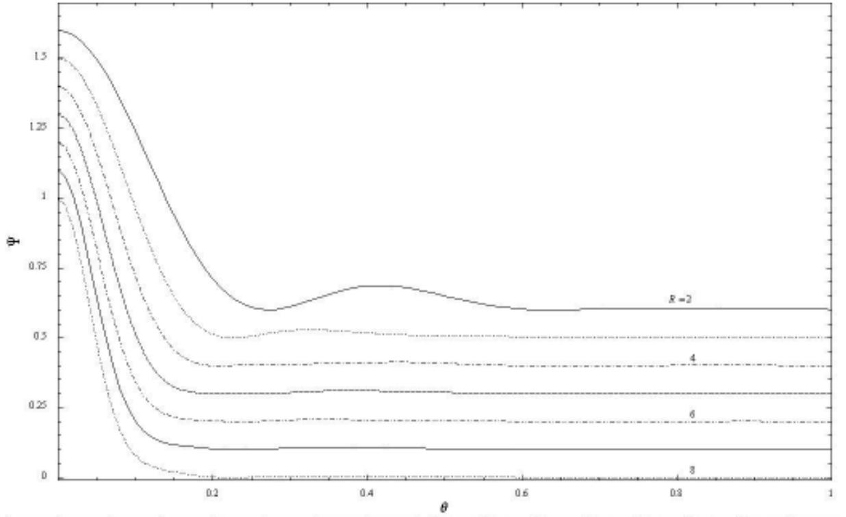
Figure 4: Beam profiles for solid annuli.
