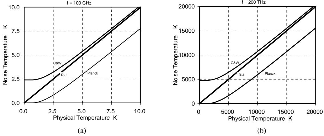
**Fig. 2.** Noise temperature vs physical temperature for a resistor, computed at (a) 100 GHz and (b) 200 THz ( $\lambda = 1.5 \mu\text{m}$ ) according to the Rayleigh-Jeans, Planck, and Callen & Welton laws.
