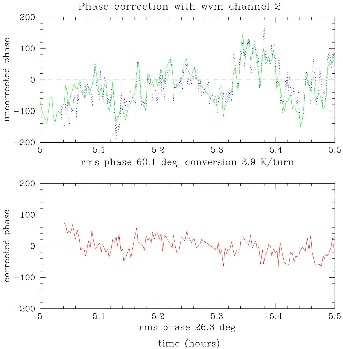
Figure 4: The radiometric phase correction for the Channel 2 is shown in detail. The lines shown are the same as in Figure 2. The radiometric phase correction closely track the astronomical data, and the significant improvement is obvious in the lower panel.
