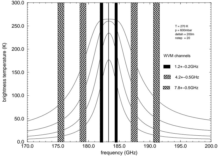
Figure 1: The three double-sideband frequency channels of the water vapor radiometer are shown superposed on the spectrum of the 183.31 GHz water line for 0.5, 1, 2, and 4 mm of PWV.
