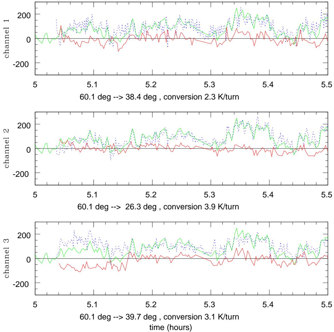
Figure 2: The raw astronomical interferometer phase (green solid line), the phase correction predicted from the radiometer measurement (blue dashed line), and the corrected interferometer phase (red solid line) are shown for each of the three radiometer channels. After subtracting a linear phase drift due to the interferometer baseline error, the rms phase fluctuations are computed as listed above.
