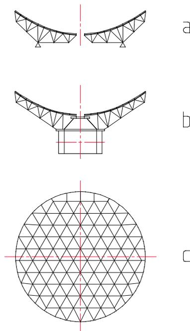
*Figure 6. Different layouts of antenna dishes. Solution a) has a polar truss pattern with circular support, b) a polar truss pattern with central hub support, and c) a 120 degree truss pattern. a) and b) are side sections whereas c) is a top view of the truss geometry.*
