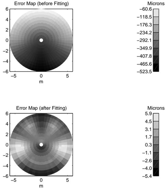
Figure 15. Example of gravity computation based on a finite element model. The elevation angle is  $60^\circ$ . The upper contour plot shows the raw surface deflection (normal to the surface) with respect to a weightless telescope. The lower plot shows the same surface after rigging angle corrections are introduced, and after the paraboloid part has been removed by postprocessing.
