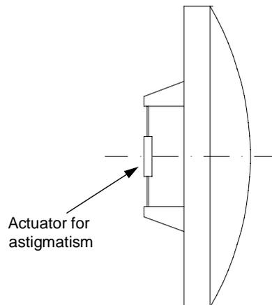
*Figure 18. Correction for astigmatism using a single actuator behind the subreflector.*
