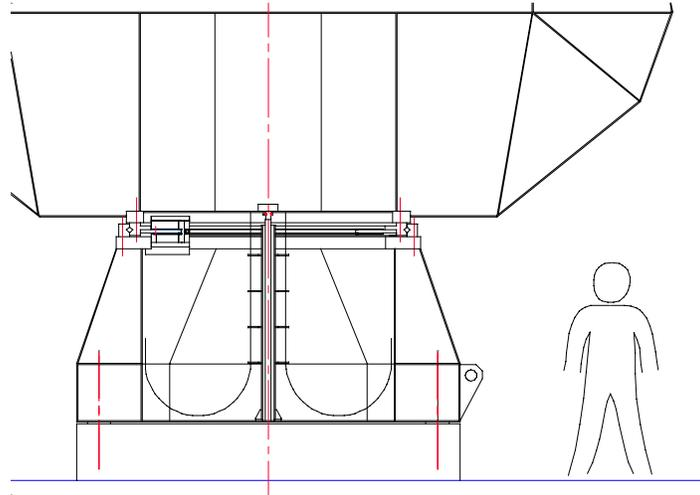
*Figure 10. Section through the lower part of the yoke and the base.*
