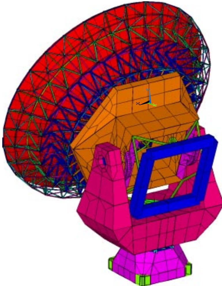
*Figure 14. Finite element model of the radio telescope.*
