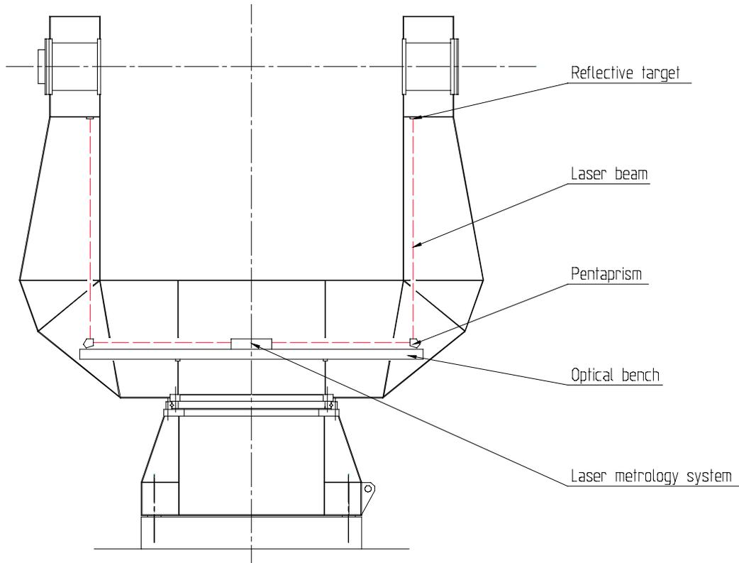
*Figure 19. A possible layout of a simple active optics system for pointing corrections. Structural deformations below elevation axis are measured.*
