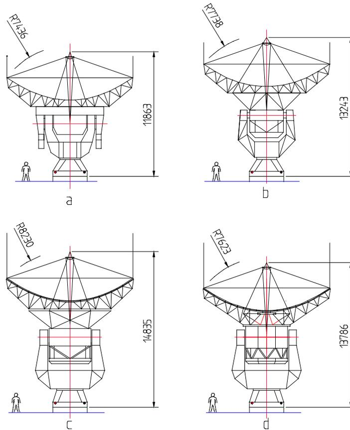
*Figure 7. Some antenna design alternatives. Design a) has elevation shafts outside the yoke. This design is best for small receiver cabins. b) is a design with a yoke having a truss structure, and with a truss structure below the BUS. c) has a yoke of plate boxes and a truss structure connecting center section and BUS. d) shows a design with a central hub in the dish. The a) and b) designs have been drawn with smaller receiver cabins.*
