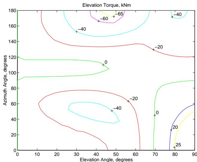
Figure 11. Total elevation motor torque for different pointing angles. Wind velocity 24 m/s.
