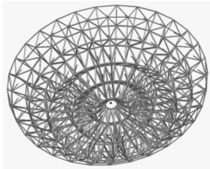
*Figure 5. Back-Up Structure (BUS) without panels. Rear view.*
