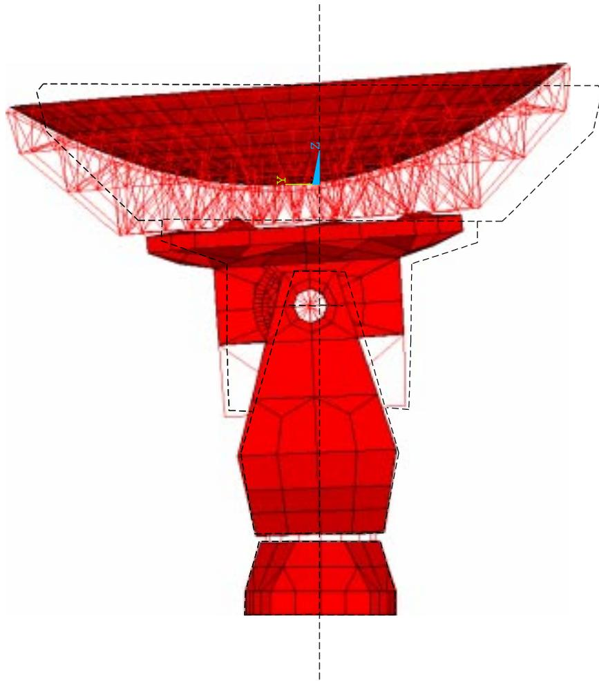
*Figure 16. Shape of the eigenmode corresponding to the lowest eigenfrequency.*
