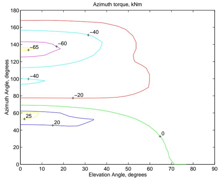
Figure 12. Azimuth motor torque for different pointing angles. Wind velocity 24 m/s.
