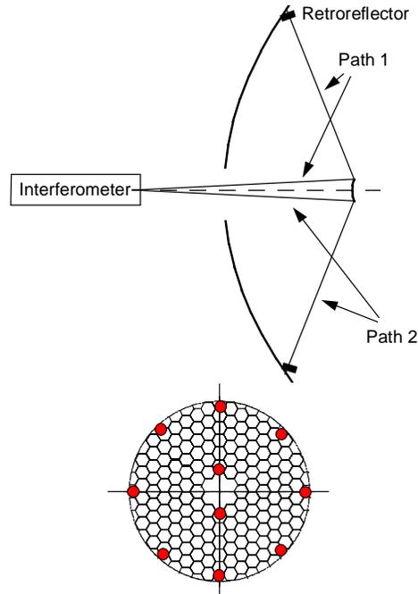
*Figure 17. Possible implementation of active optics for low spatial frequency corrections. The upper drawing shows possible laser paths. The lower sketch (here shown with hexagonal panels) illustrates that the form of the antenna dish is measured only at a few carefully selected points. This system could correct for changes in focus, astigmatism, triangular coma and quadratic astigmatism.*
