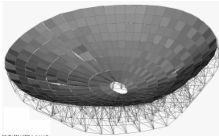
*Figure 8. Eigenmode corresponding to the lowest eigenfrequency of the dish with thermal expansion devices included.*
