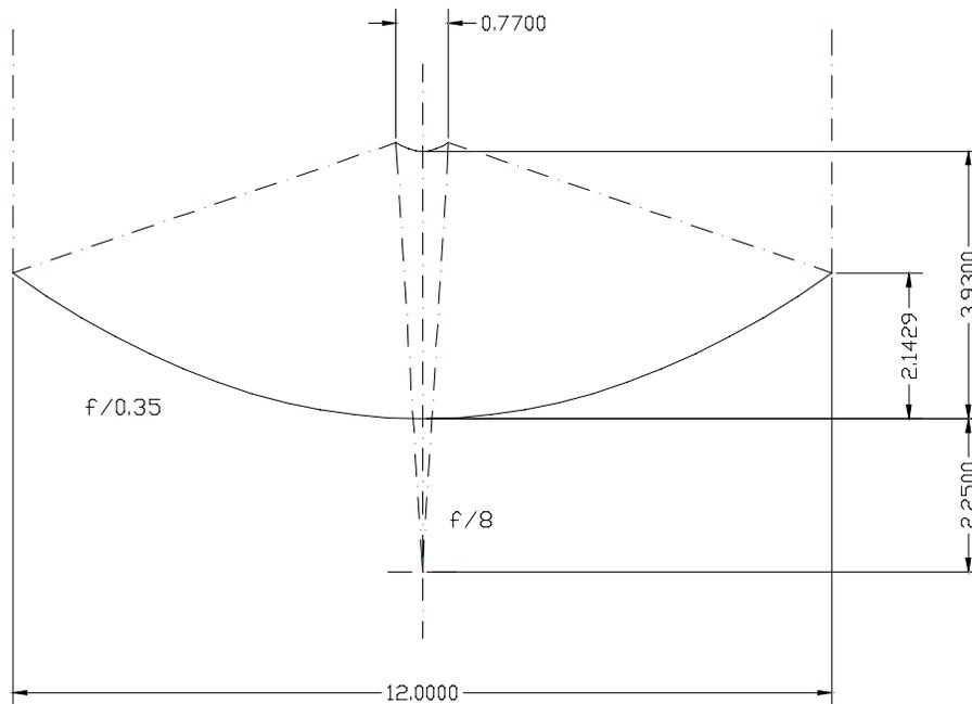
*Figure 1. Optical Layout of antenna.*
