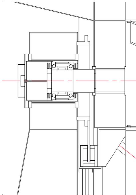
*Figure 9. Section through one of the yoke arms. The spherical ball bearing and the direct drive torque motor can be seen.*
