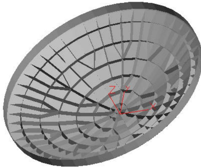
Fig. 4.1.2: subreflector structure in aluminium
