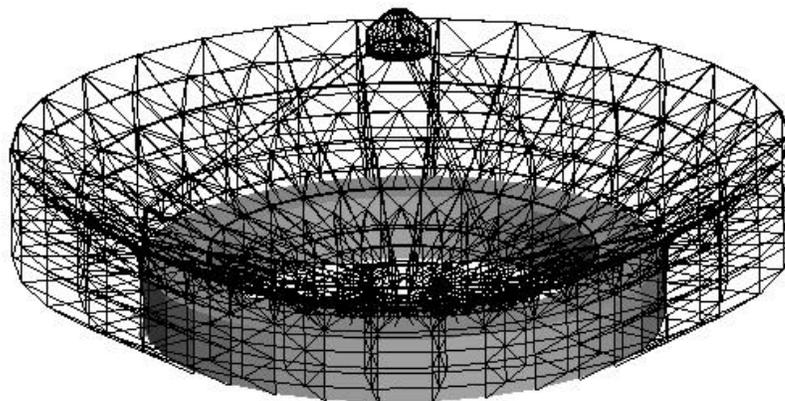
Fig. 4.2.3: toroidal box structure inside the reflector backup structure
