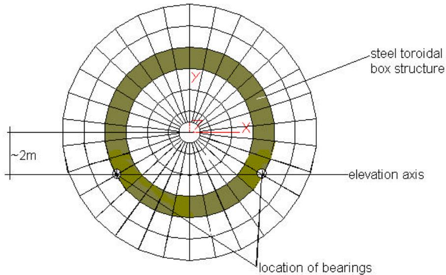
Fig. 4.2.4: position of elevation bearings with respect to the reflector geometry
