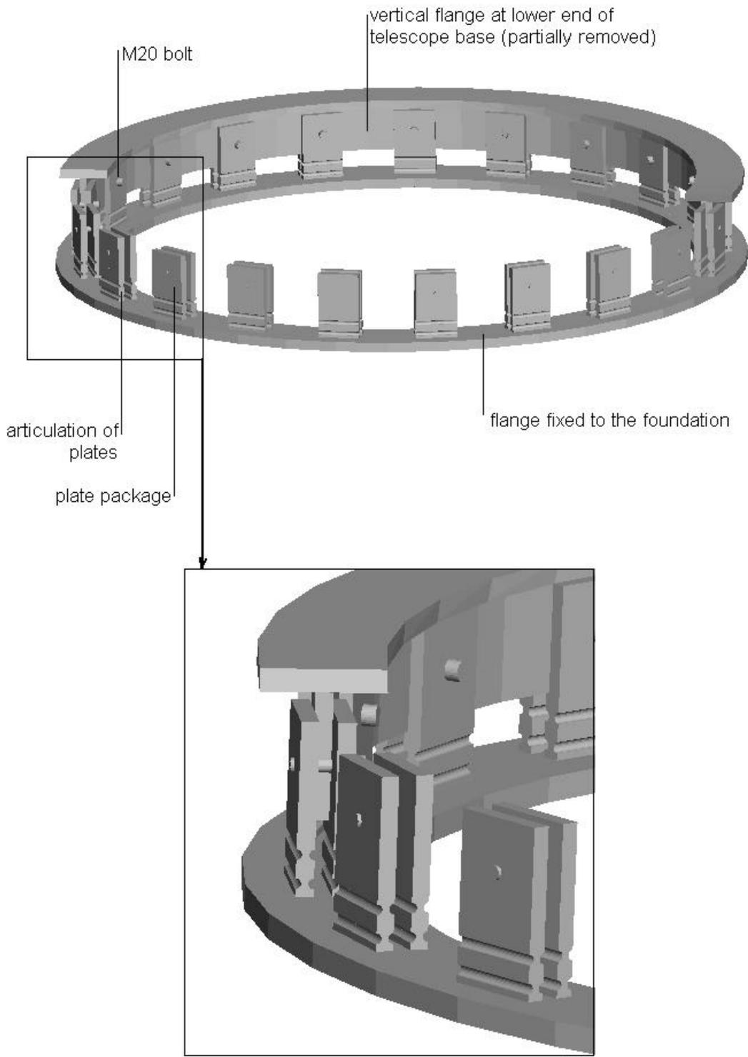
Fig. 4.5.1: clamping of the telescope base to the plate packages on the foundation
