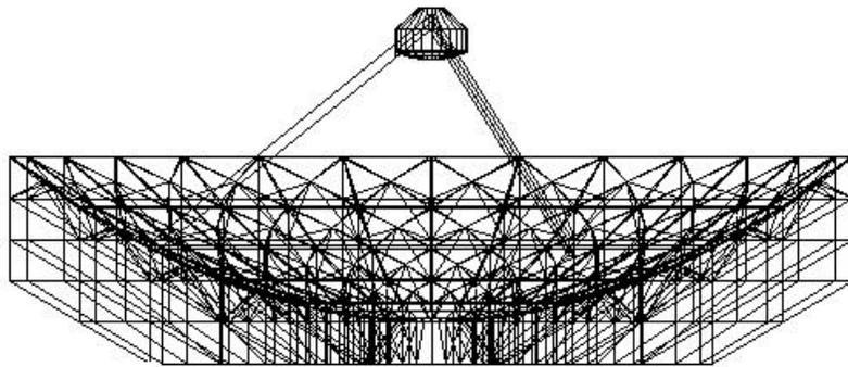
Fig. 4.2.1: main reflector and secondary mirror truss structures
