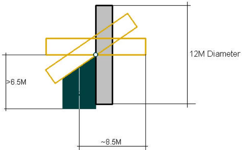
b) elevation axis displaced relative to the azimuth axis
