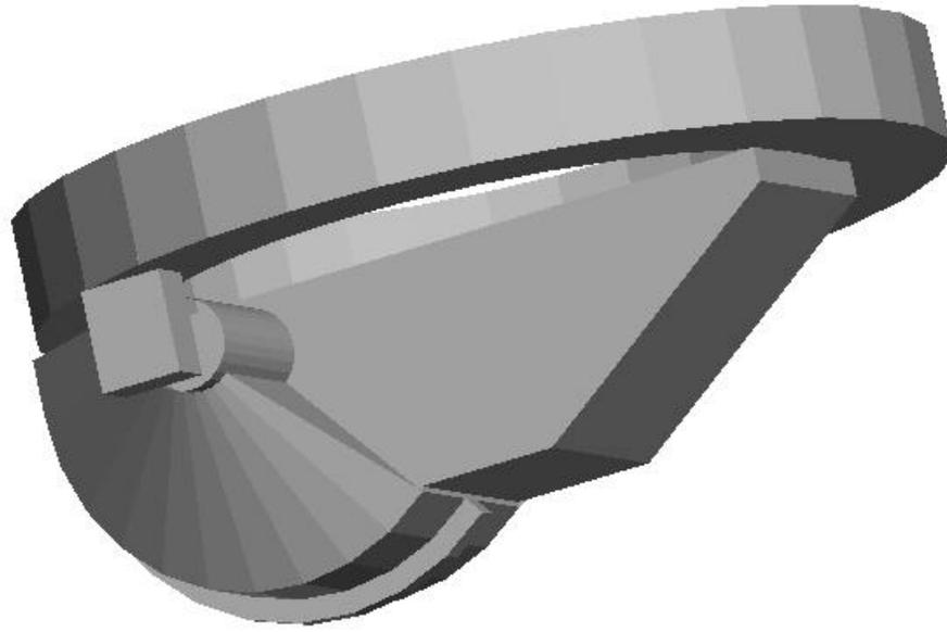
Fig. 4.3.2: shaded view on the assembly of receiver cabin, hub and ring box
