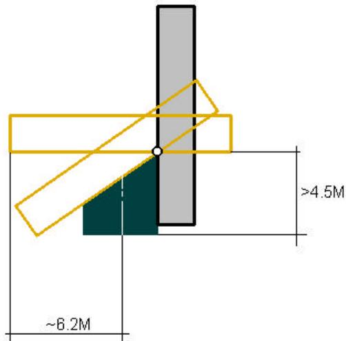
c) elevation axis displaced relative to azimuth and optical axis
