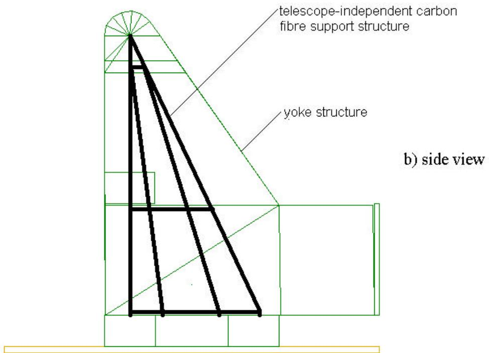
Fig. 5.2.1: sketch of telescope-independent reference support structure in carbon fibre
