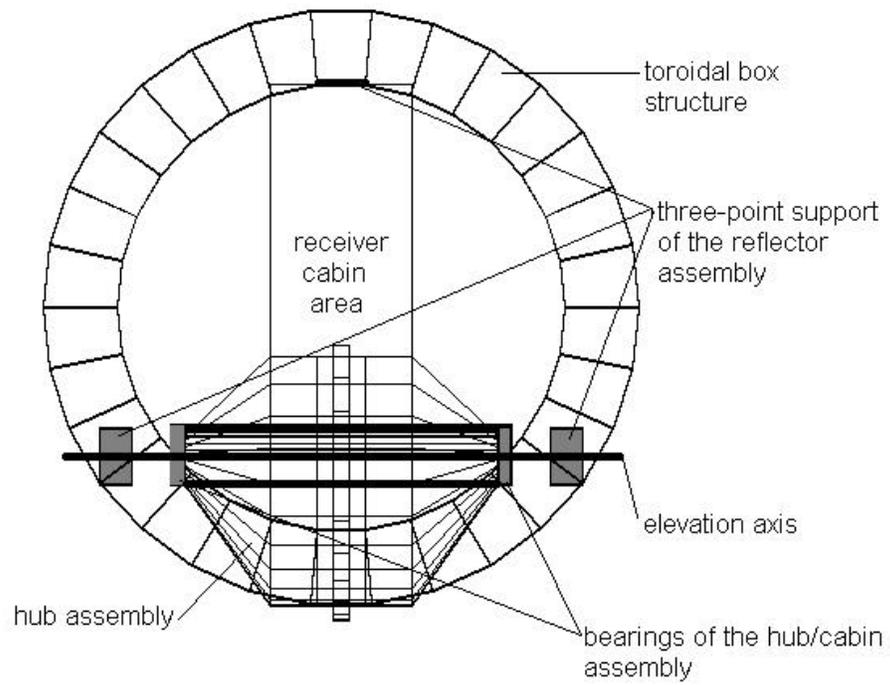
Fig. 4.3.3: three-point support of the reflector ring box structure
