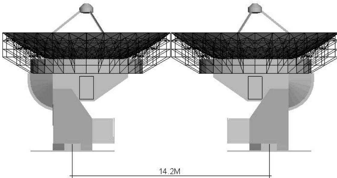
Fig. 4.1.3: two telescopes in a closest packing position
