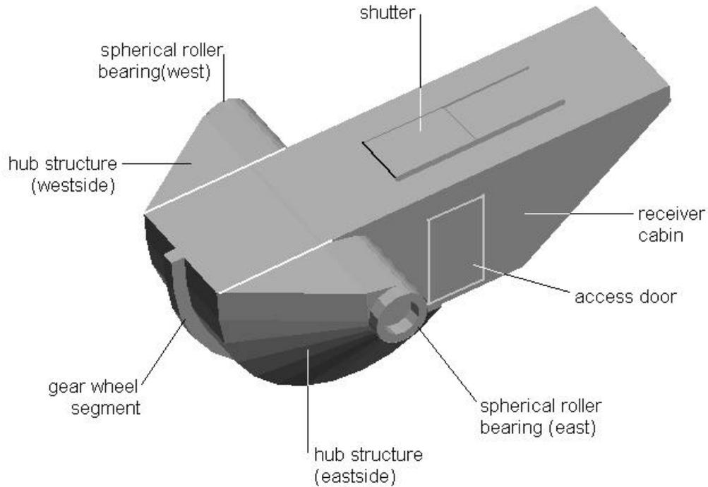
**Fig. 4.3.1: computer vision of the hub and cabin assembly**
