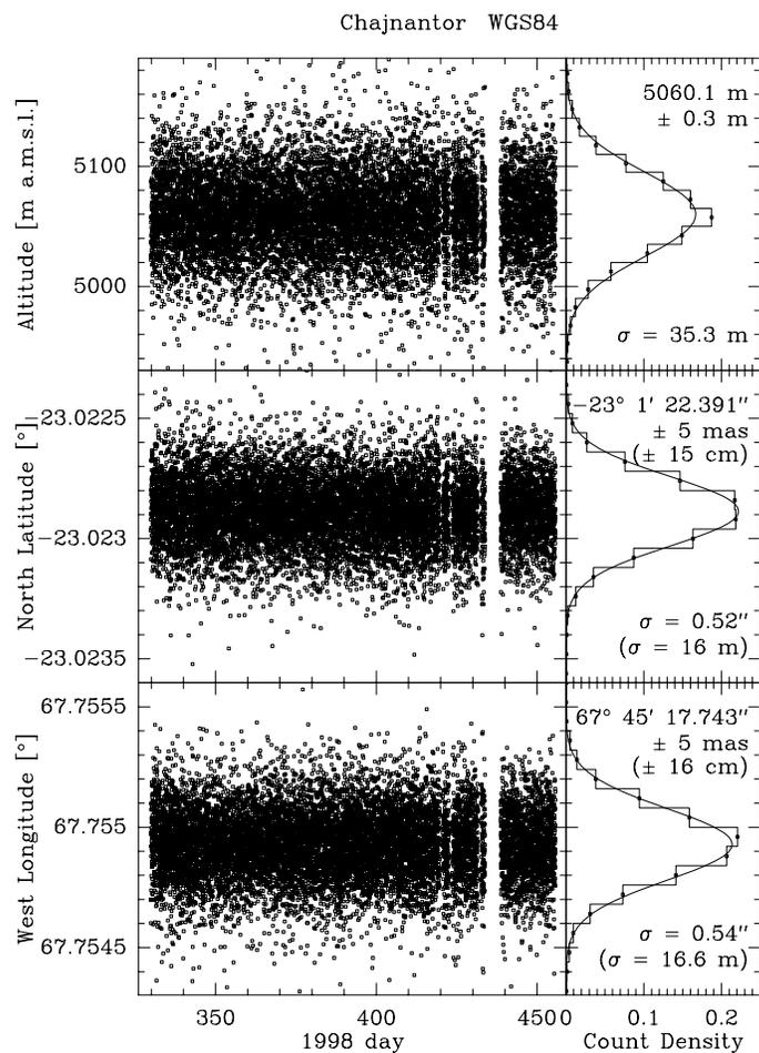
Figure 1: Measured positions of MMA equipment container on Chajnantor, Chile. In the right panels, the histograms show the actual distribution of the measured positions and the curves are normal (Gaussian) distributions for the parameters derived from the data. Note scale difference between latitude-longitude and altitude.
