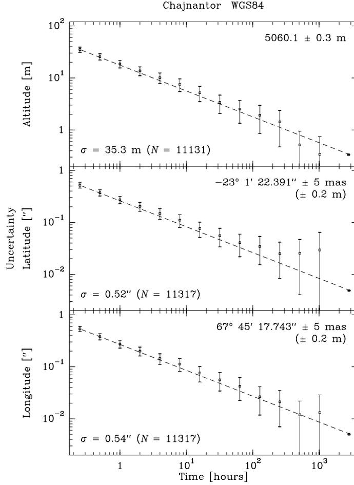
Figure 3: Measurement uncertainty for different averaging times. The error bars illustrate the sampling uncertainty for a normal distribution,  $\sigma_\sigma/\sigma = (2/(N-1))^{1/4}$  (Bailey 1971). The dashed lines show the decrease with time<sup>0.5</sup> expected for sequentially uncorrelated data.
