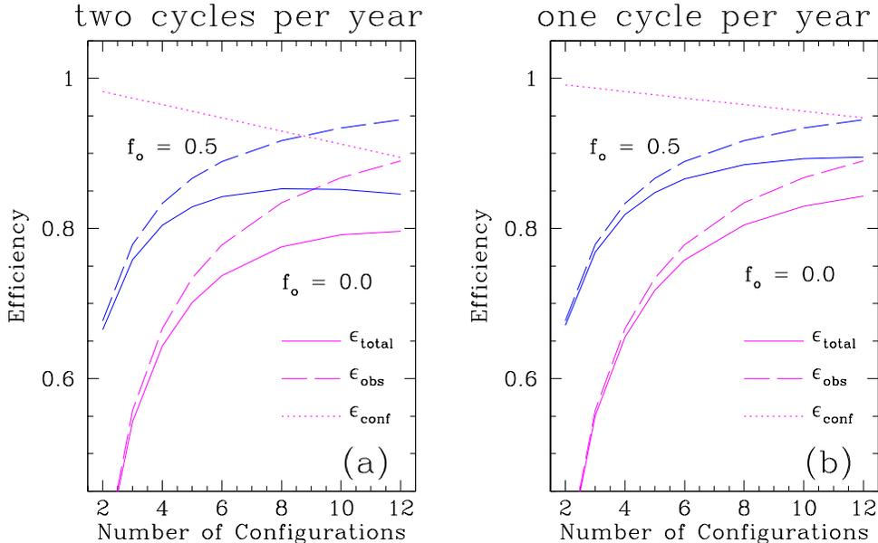
Figure 1: A comparison of the array efficiency between one full configuration cycle per year and two configuration cycles per year. The cases considered here are essentially the same as in Figures 1&2 of Holdaway (1998). The main difference is in the reconfiguration efficiency (dotted line), and the monetary cost comparison is given in Table 1.
