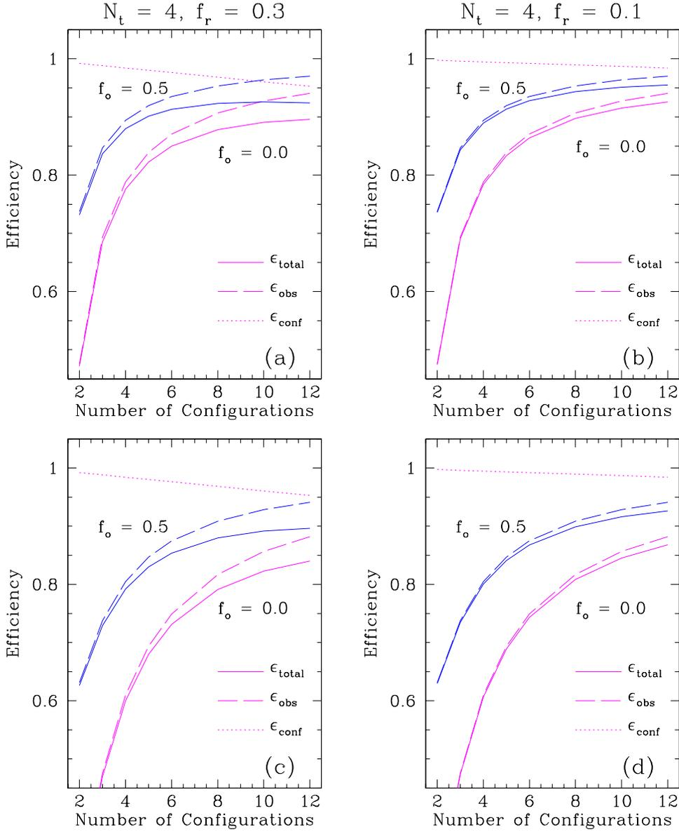
Figure 5: The array efficiencies are computed for (a) assuming science projects can be carried out during 70% of reconfiguration time ( $f_r = 0.3$ ); and (b) during 90% of time ( $f_r = 0.1$ ) assuming  $N_t = 4$  and  $p = 0.5$ . These calculations can be compared with the  $f_r = 0.5$  case previously considered by Holdaway (e.g. Fig. 4a). The corresponding calculations for  $p = 1$  cases are shown in (c)&(d).
