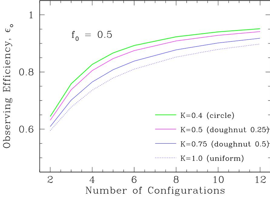
Figure 3: Observing efficiency  $\epsilon_{obs}$  for various configuration designs considered in Figure 2. The observing efficiency for the more concentrated circle and thin doughnut arrays are higher because they are more robust against tapering and offer up to 10% gain in observing efficiency over a uniform array.
