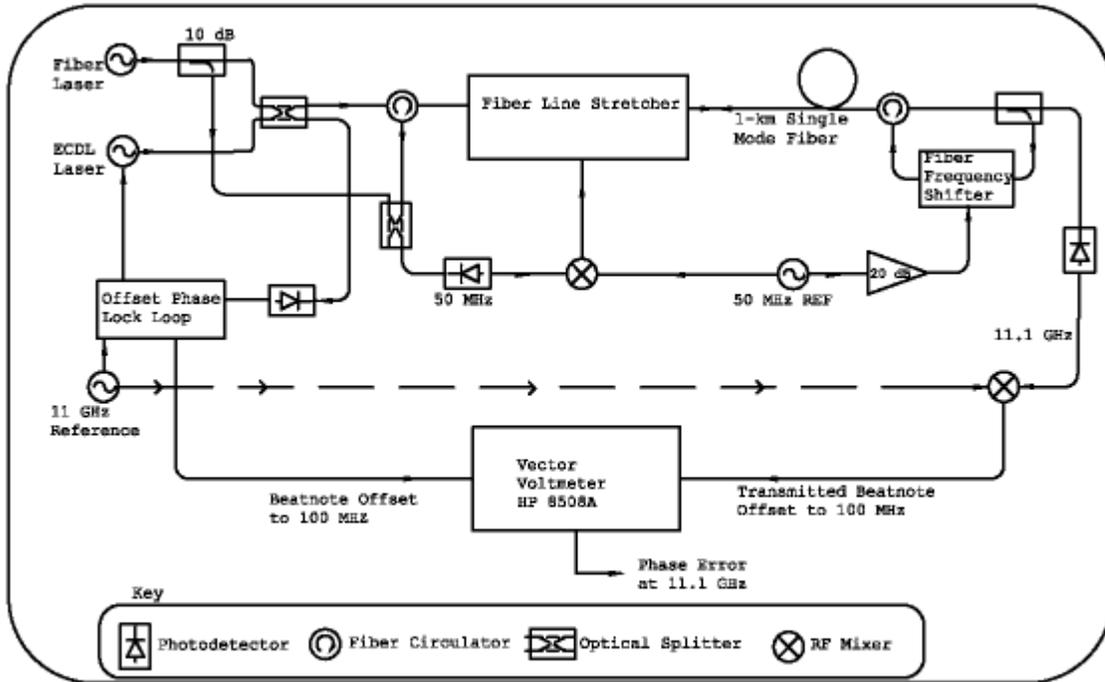
Figure 1: Simultaneous demonstration of round-trip phase correction and transmission of photonic LO.
