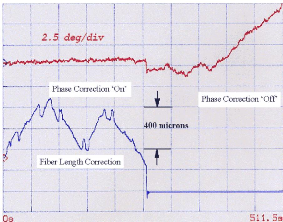
Figure 4: Comparison of Phase Difference between 11.1 GHz phase-locked beatnote before and after being transmitted through a 1-km single mode fiber: with correction 'on' and 'off'. Bottom trace is the movement of the slow fiber length corrector
