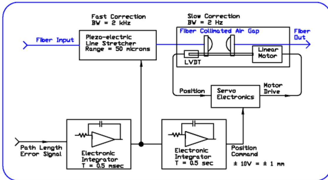
Figure 3: Fiber Line Stretcher
