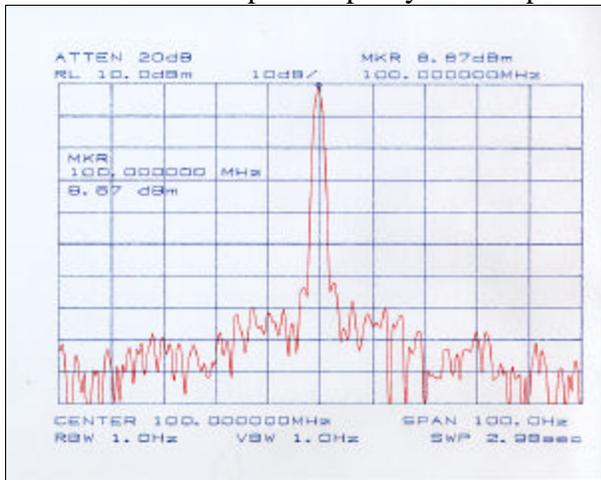
**Figure 2: 100 MHz beatnote derived from offset in the phase lock loop**
