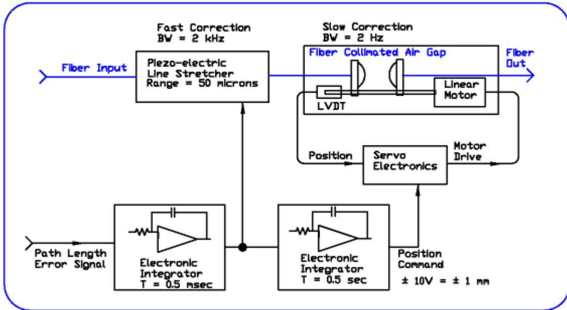
Figure 3: Fiber Line Stretcher
