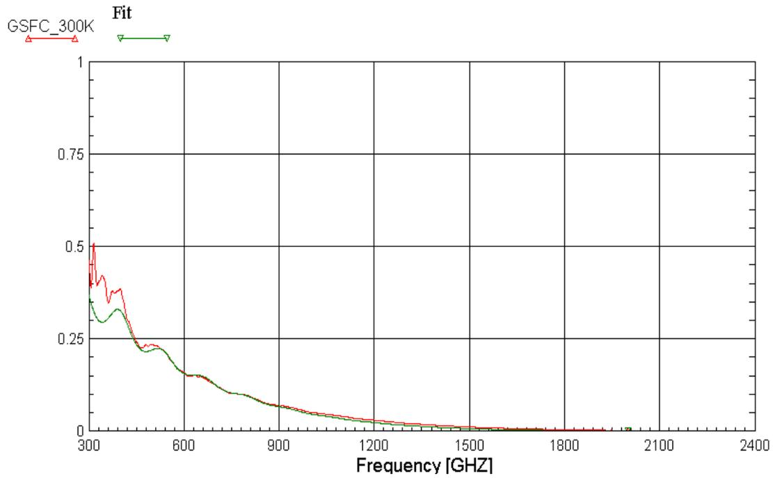
**Figure 3** MMICAD fit to 300 K transmittance data.
