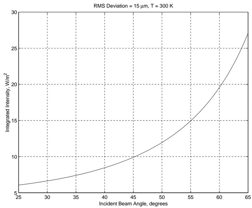
Figure 5: Output Intensity (into feed) vs.  $\alpha$ , Fixed RMS Deviation
