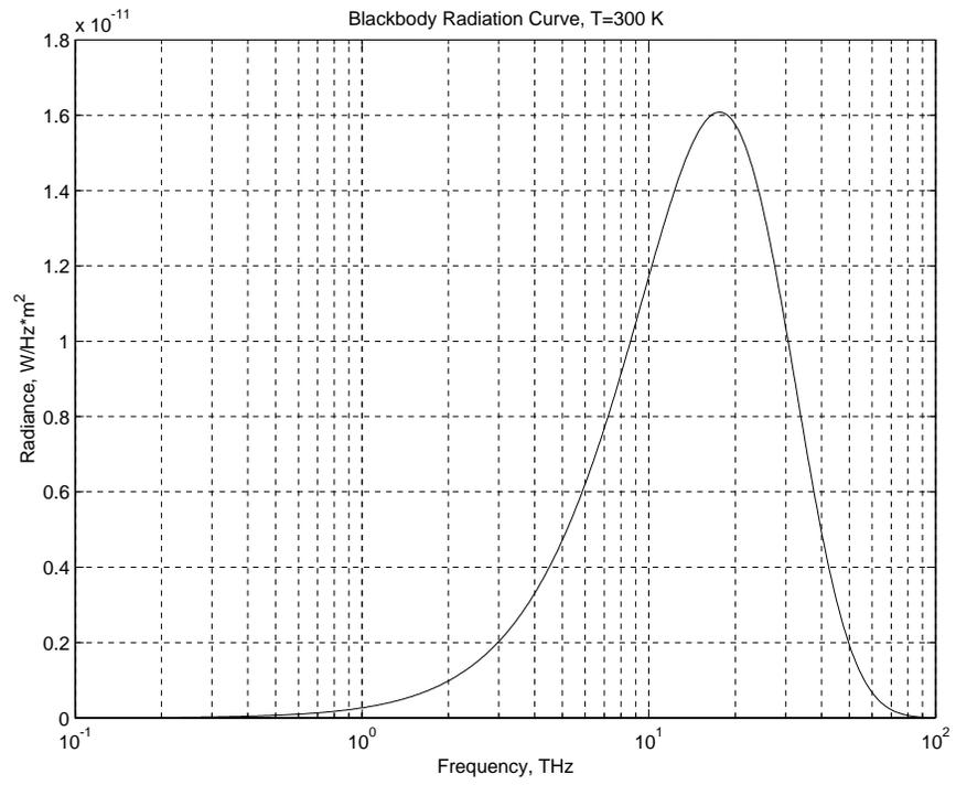
Figure 2: Room Temperature Blackbody Radiation Curve vs. Frequency
