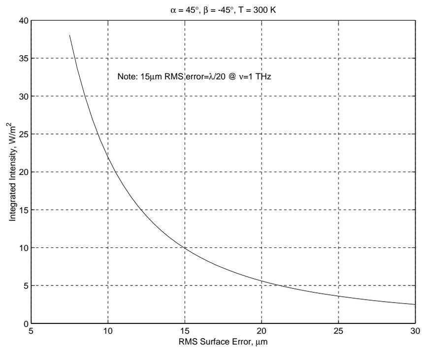
Figure 4: Output Intensity (into feed) vs. RMS Deviation,  $45^\circ$  Incidence
