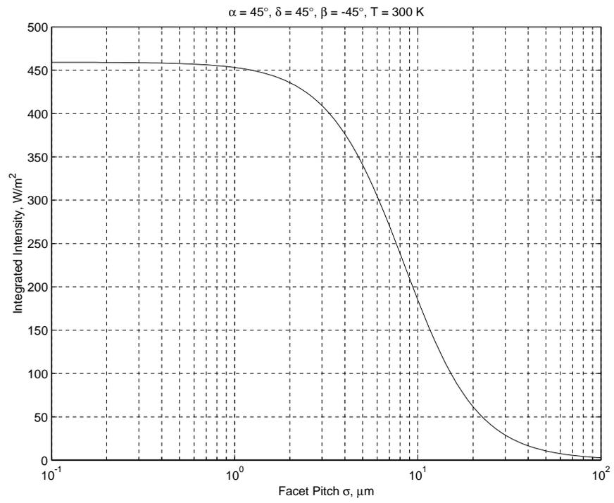
Figure 3: Grating Filter Output Intensity (into feed) vs. Facet Spacing
