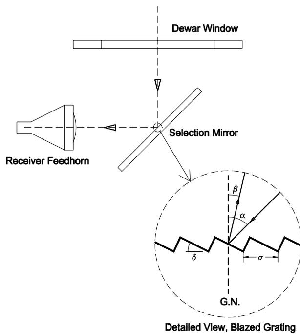
Figure 1: Receiver Selection Mirror/Diffraction Grating Filter
