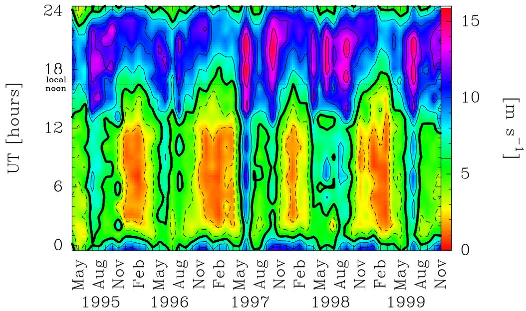
Figure 1: Hourly-monthly median wind speed at Chajnantor. Heavy contour is overall median,  $6 \text{ m s}^{-1}$ , and contour interval is  $2 \text{ m s}^{-1}$ . Local Solar time is  $\text{UT} - 4.5 \text{ h}$ .
