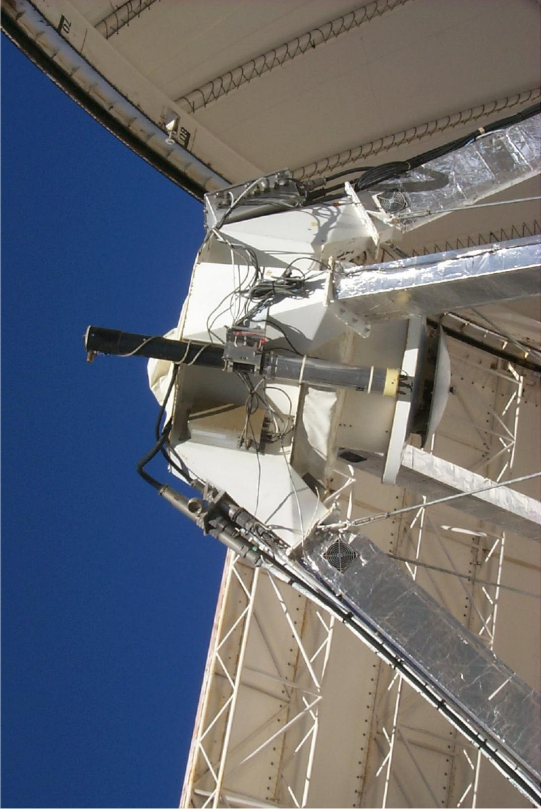
Figure 1: The 12 Meter Telescope optical pointing telescope. This system has been used to diagnose and characterize the pointing behavior of the 12 Meter Telescope for over 10 years.
