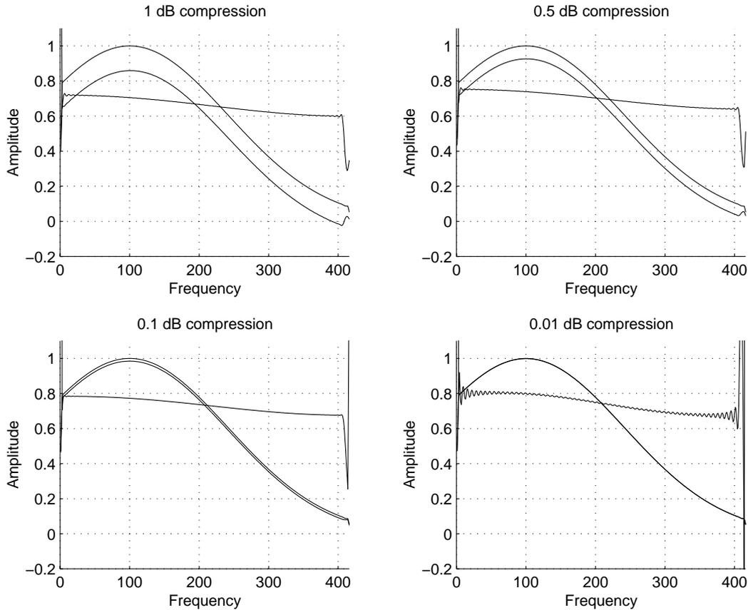
Figure 5: Compression in correlator multipliers for an input signal with a smooth bandpass. The upper curve in each frame is the input spectrum, the similar curve slightly below is the spectrum with a  $\tanh(x)$  compression, and the slightly tilted line below is the difference between the two magnified by factors of 5, 10, 50, and 500 in panels with decreasing compression.
