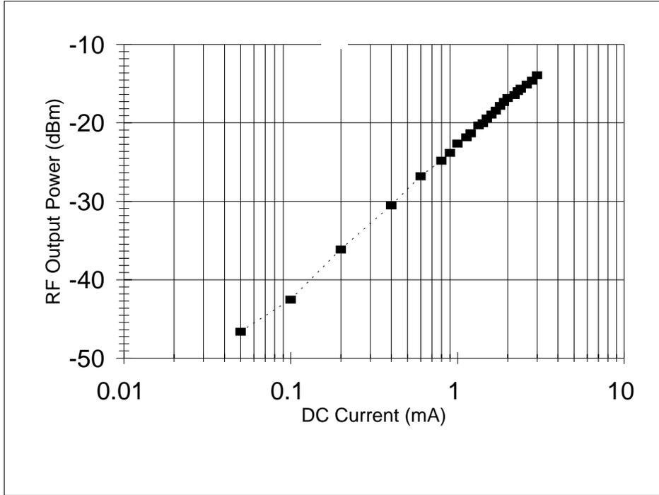
Figure 3: Output power vs. input level at 109 GHz. Responsivity is approximately 0.24 mA/mW after coupling loss.
