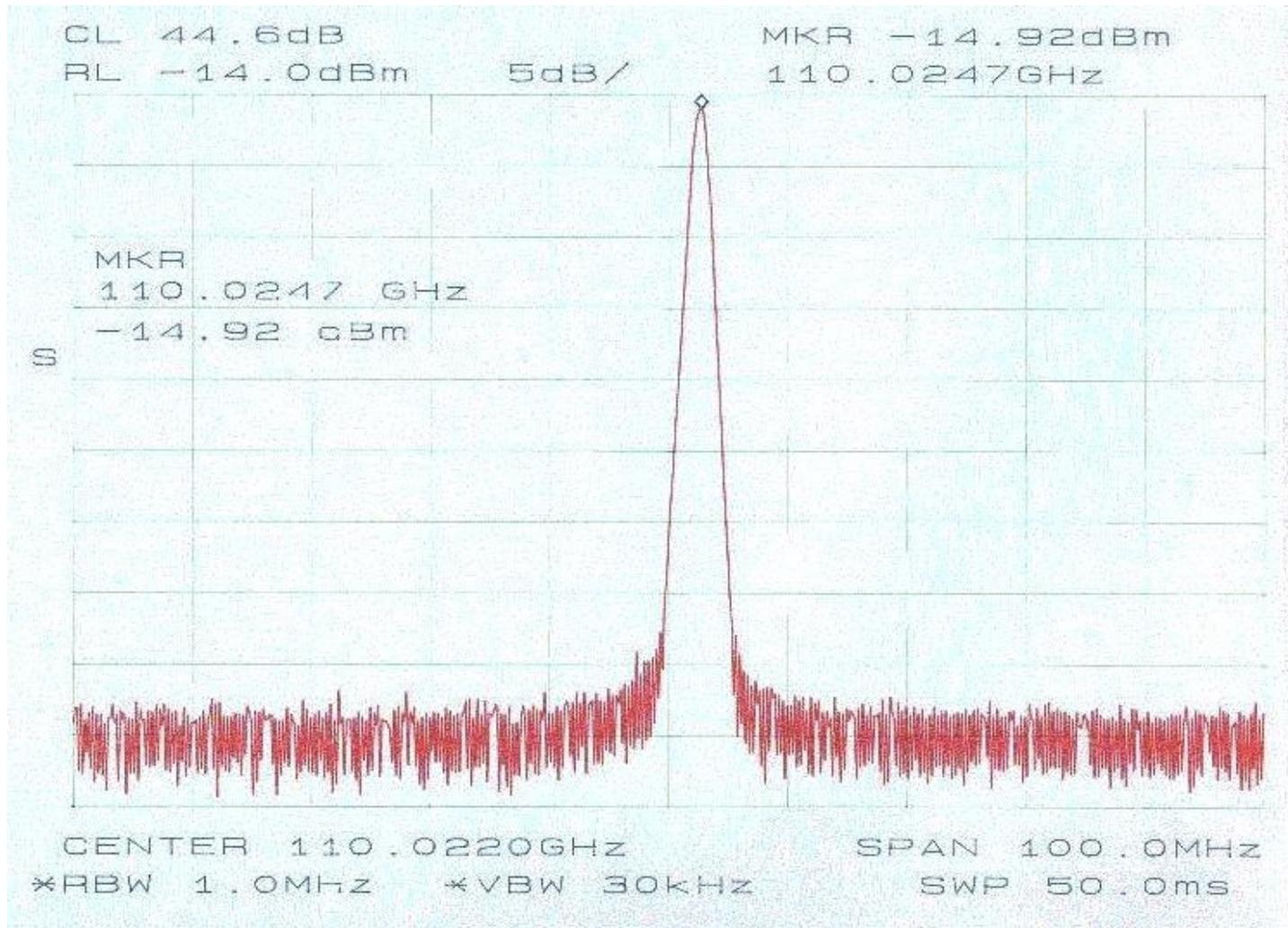
Figure 4: Output spectrum from laser heterodyne and u2t photomixer at 110 GHz
