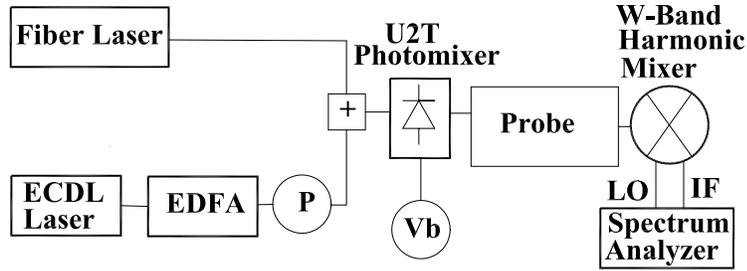
Figure 1: Test Setup for Heterodyne Measurement of U2T photomixer. EC DL: external cavity diode laser; EDFA: erbium doped fiber amplifier; P: polarization controller; +: power combiner; Vb: bias to photomixer; Probe: coplanar waveguide to WR-10 adapter probe.
