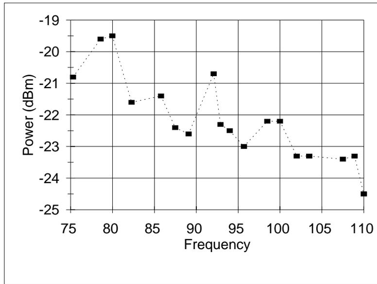
Figure 2: Power output vs. frequency for u2t photomixer across full WR-10 waveguide band. Input optical power is 4.6 mW, photomixer DC bias is -2.0 volts, 1.1 mA. The power level shown is at the input of the harmonic mixer.
