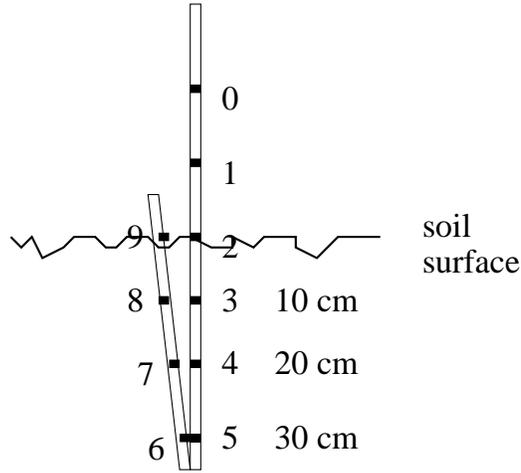
Figure 1: Thermometer positions above and below the surface. The thermometers, spaced by  $100 \pm 3$  mm, are rigidly attached to a stick. The stick was broken and folded between sensors 5 and 6, so the relative depths of the sensor pairs are only accurate to  $\pm 1$  cm, which is about the absolute accuracy of the sensor depths.
