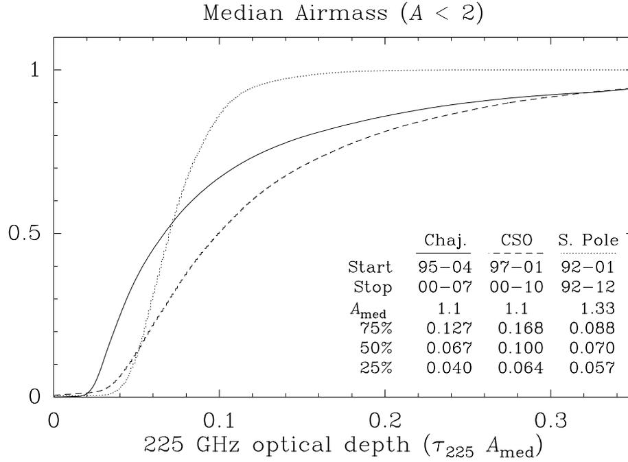
Figure 4: Cumulative distributions for Chajnantor, the CSO, and the South Pole of the 225 GHz optical depth at the median airmass ( $\tau_{225} A_{\text{med}}$ ) for observations near meridian transit and  $z < 60^\circ$  ( $A < 2$ ).
