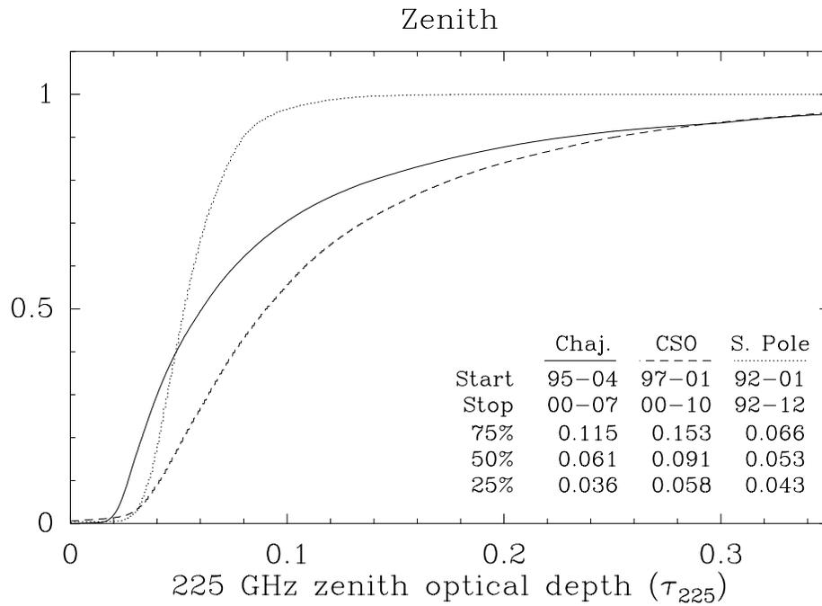
Figure 3: Cumulative distributions of the 225 GHz zenith optical depth ( $\tau_{225}$ ) measured at Chajnantor, at the CSO, and at the South Pole.
