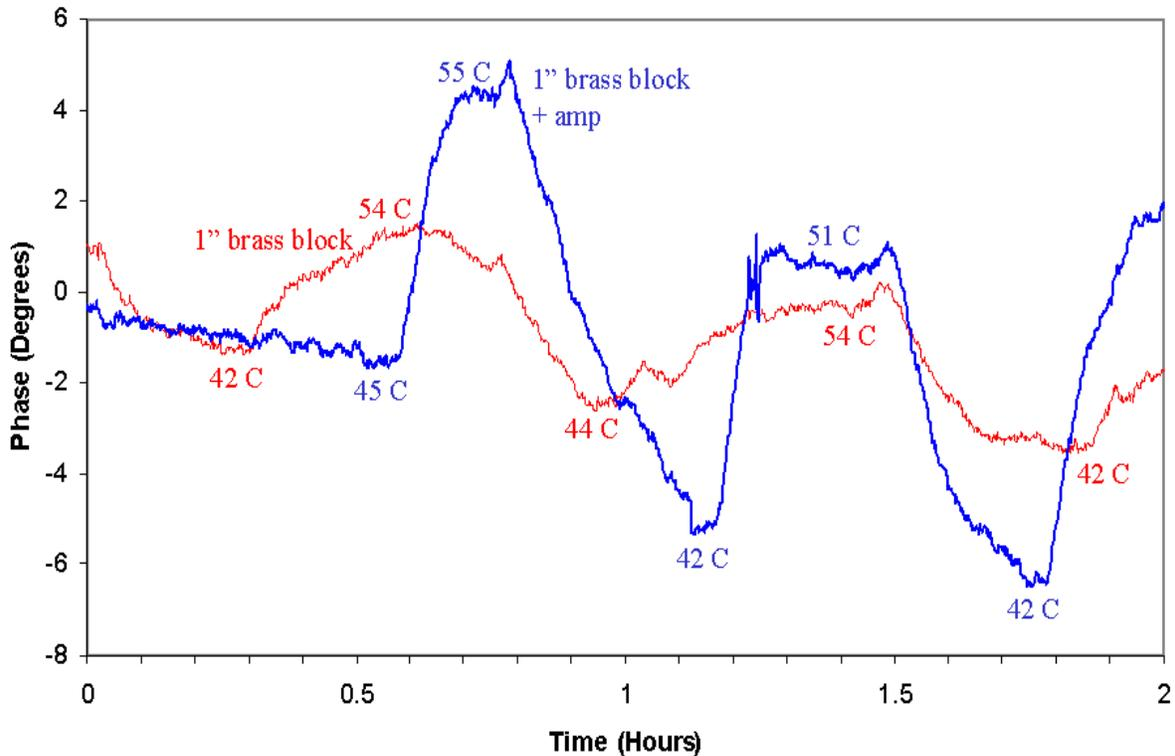
**Figure 5** Phase of Amplifier #4 for different temperatures ==> 0.4 degree phase/degree C at 108 GHz
