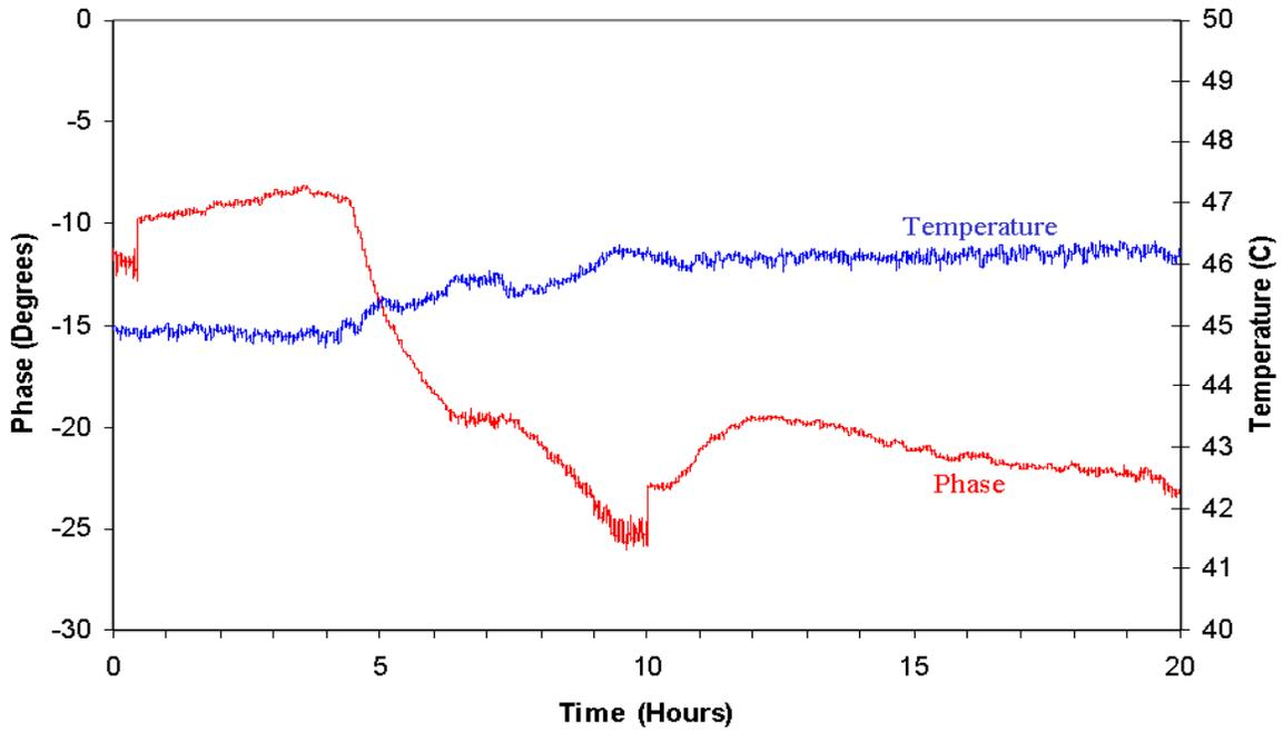
Figure 6 Raw phase data for 108 GHz Driver and Physical Temperature vs time in Hours
