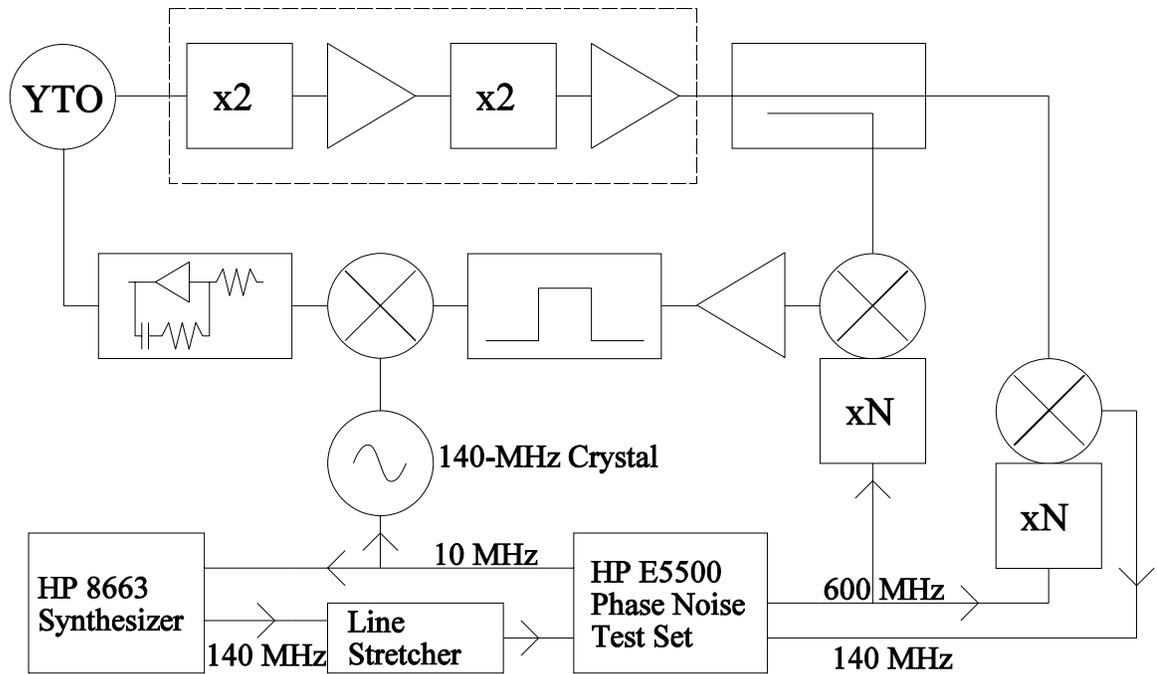
**Figure 1** Block Diagram of Phase Drift Test Set
