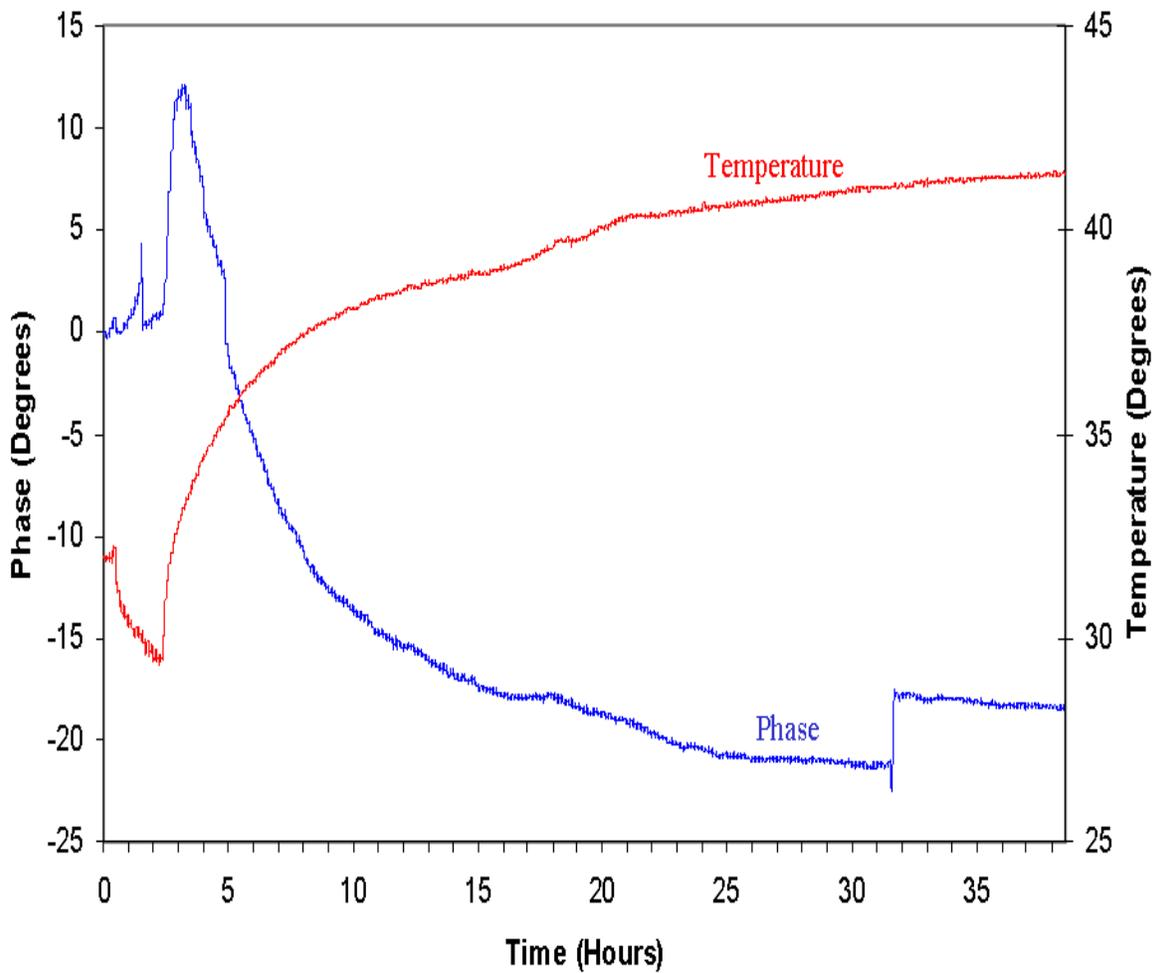
**Figure 2** Raw Data for 76 GHz Source Locked at 19 GHz
