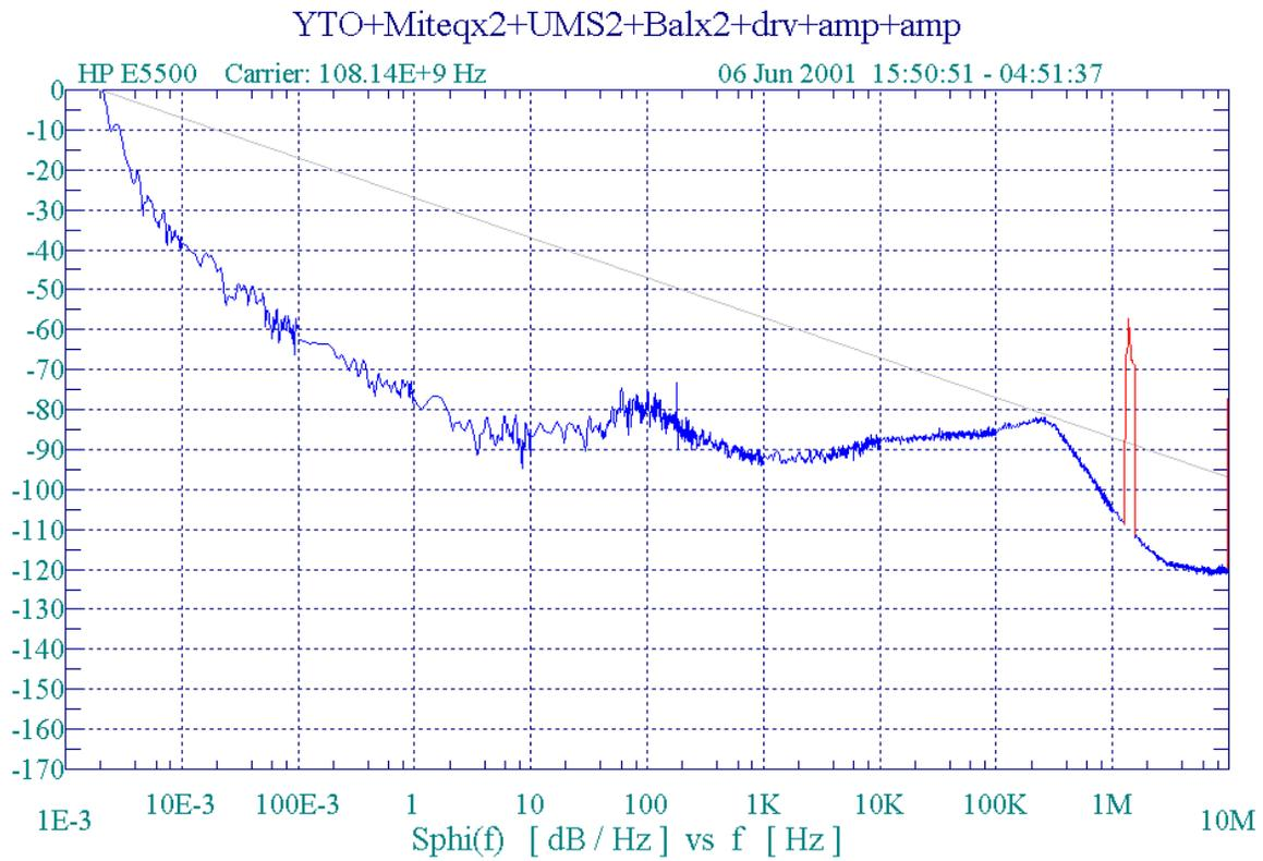
**Figure 4a** Phase Noise to 1 milliHz of System Phase Locked at 108.14 GHz with the final power amplifier outside the PLL
