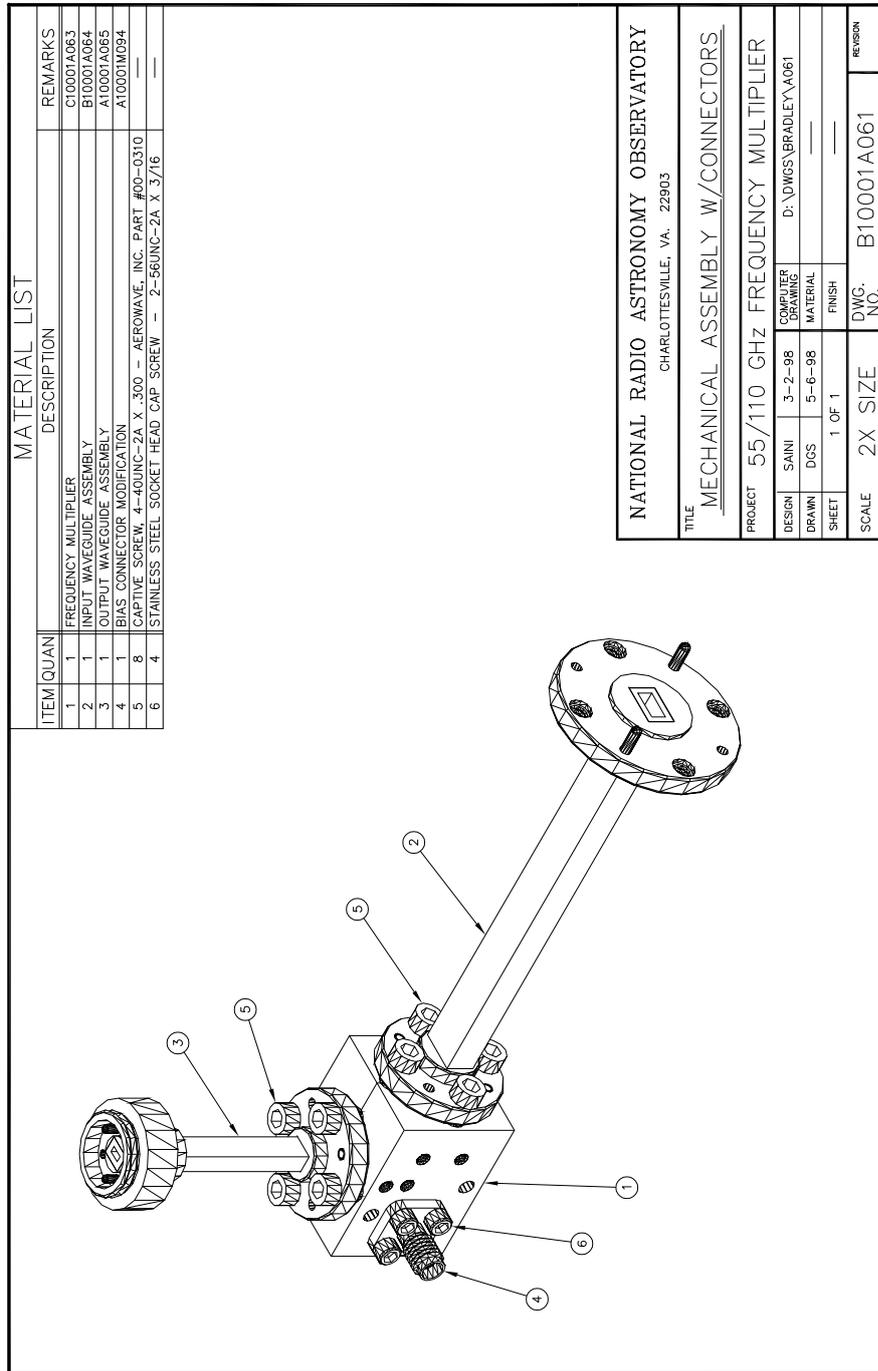
**Figure D.1:** 55/110 GHz frequency doubler: Mechanical assembly of the split block showing the DC bias connector and the waveguide flange adapters.
