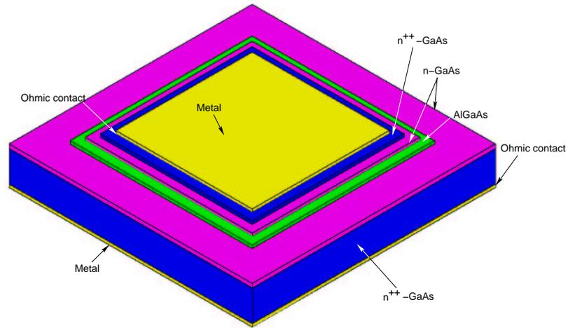
**Figure A.3:** Discrete hetero-junction barrier varactor diode.
