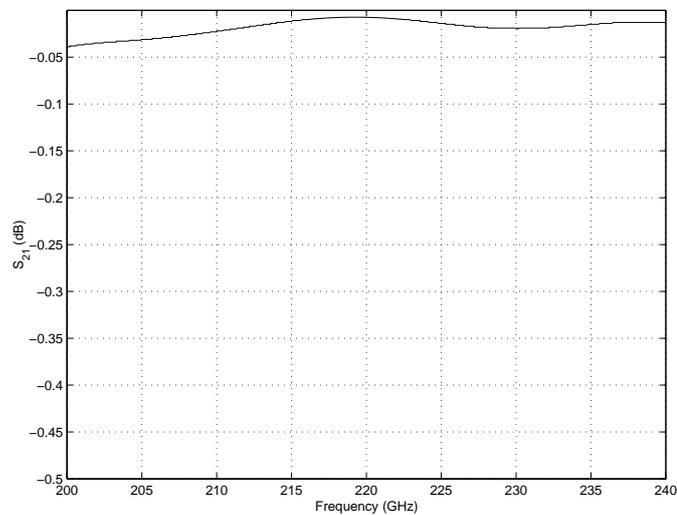
**Figure 2.38:** Plot of  $S_{21}$  for the complete output coupling arrangement, including the microstrip to one-fifth height waveguide probe, DC-bias filter and the one-fifth height to full height taper (simulated).
