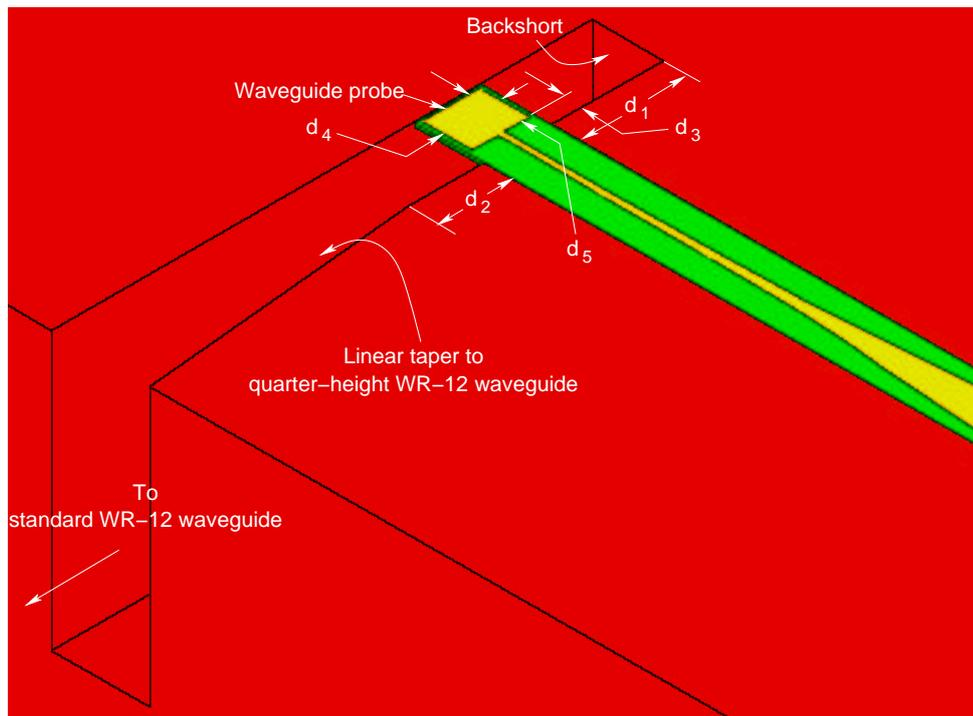
**Figure 4.14:** Design of the input coupler for the 80/240 GHz frequency tripler. Only bottom part of the mount that seats the quartz circuit is shown. The dimensions that were optimized to achieve a good coupling efficiency are marked.
