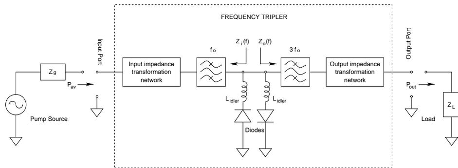
**Figure 4.3:** A practical frequency tripler circuit configuration based on anti-parallel arrangement of diodes.
