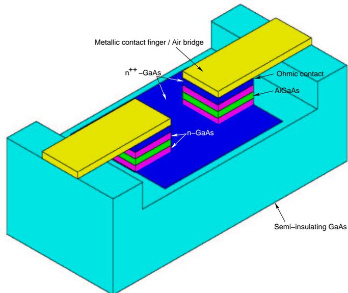
**Figure A.4:** Planarized hetero-junction barrier varactor diode.
