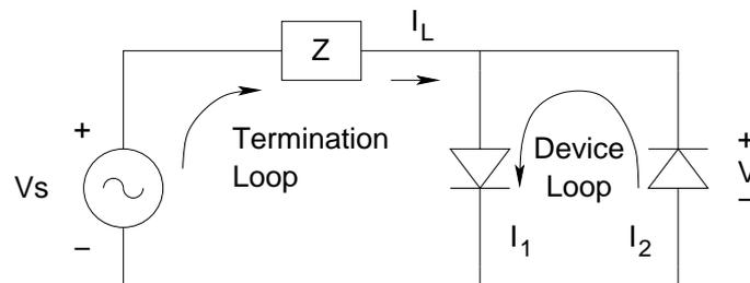
**Figure 4.2:** An alternate tripler circuit employing anti-parallel diode arrangement.
