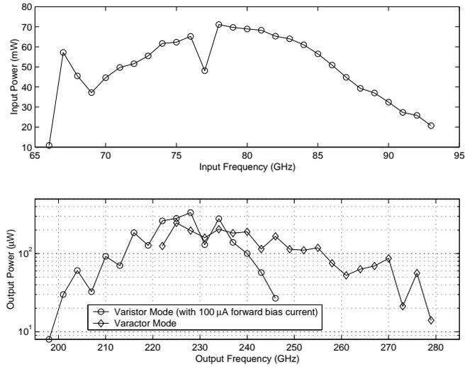
**Figure 4.33:** Measured performance of the 80/240 GHz frequency tripler, built using a diode chip having 6  $\mu\text{m}$  diameter anodes.
