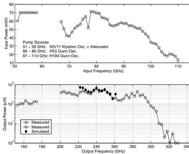
**Figure 4.38:** Performance of the modified 80/240 GHz frequency tripler built using a diode chip having  $6\ \mu\text{m}$  diameter anodes, with the DC bias bypass capacitor shorted to the ground pad with silver epoxy.
