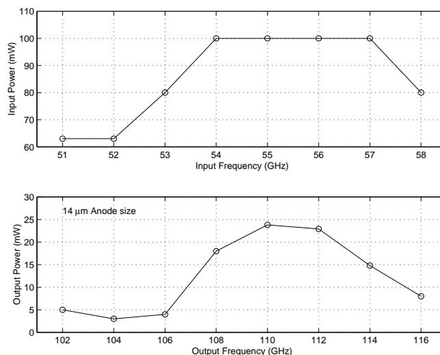
**Figure 2.29:** Plot of the measured output power versus frequency for the 55/110 GHz frequency doubler using a diode array with  $14 \mu m$  diameter anodes.
