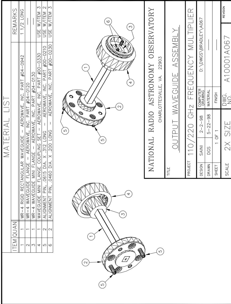
Figure D.19: 110/220 GHz frequency doubler: WR-4 output waveguide flange adapter assembly.
