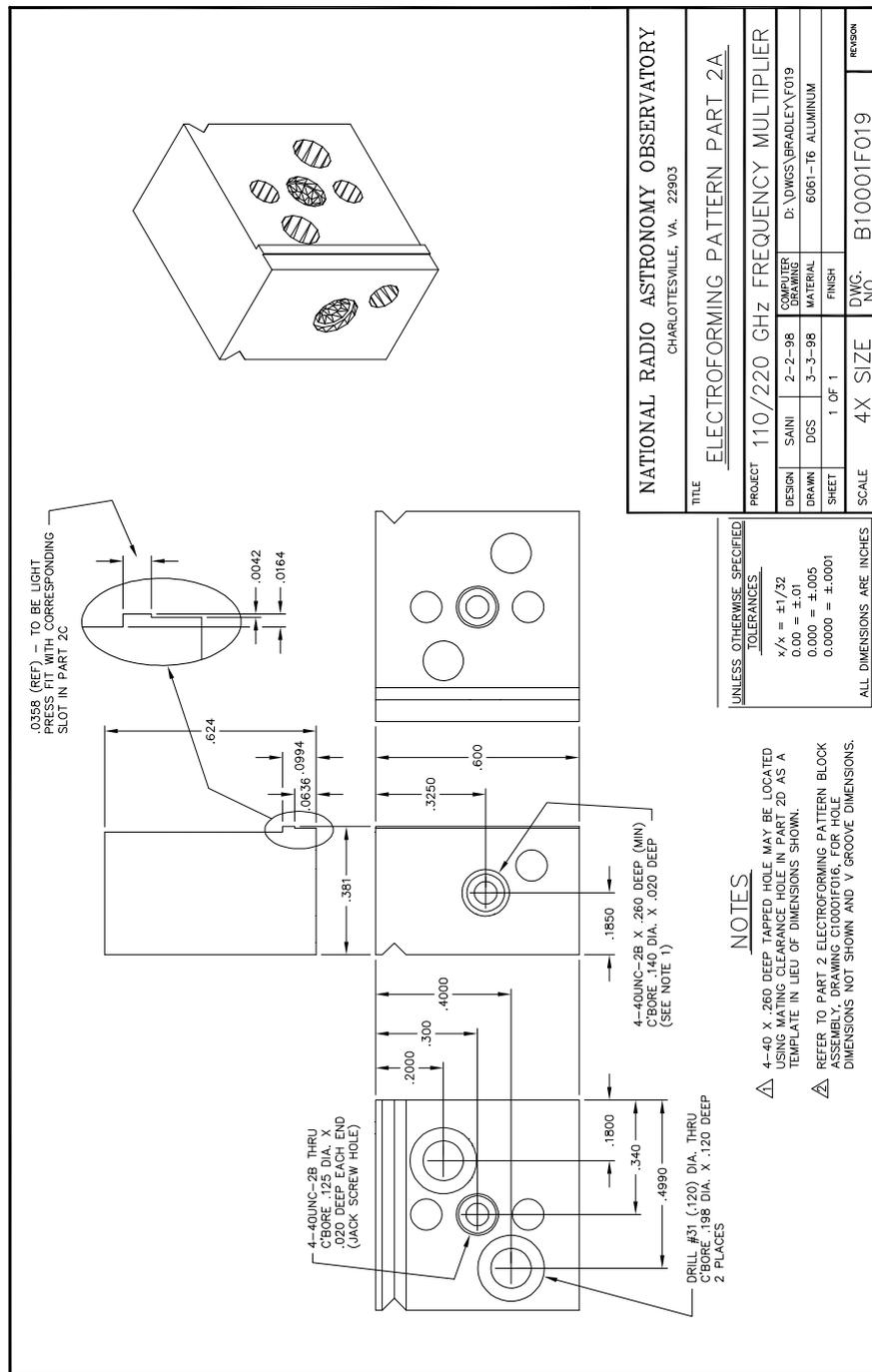
Figure D.26: 110/220 GHz frequency doubler: Mechanical details of the mandrel part 2A.
