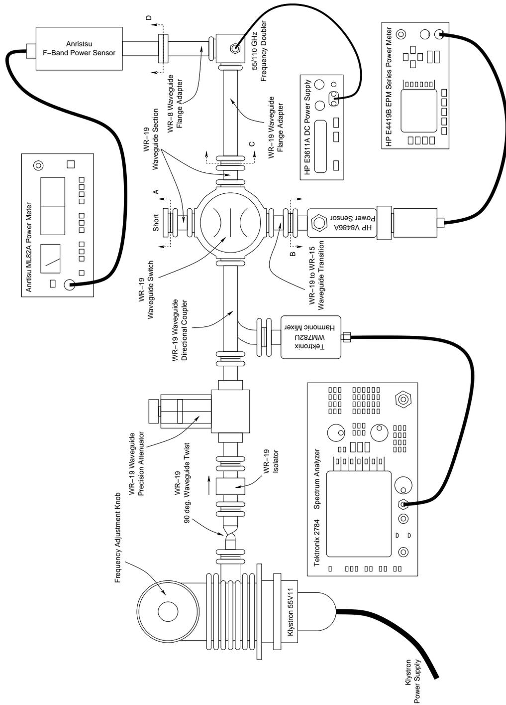
Figure 2.25: Experimental setup for evaluation of the 55/110 GHz frequency doubler.
