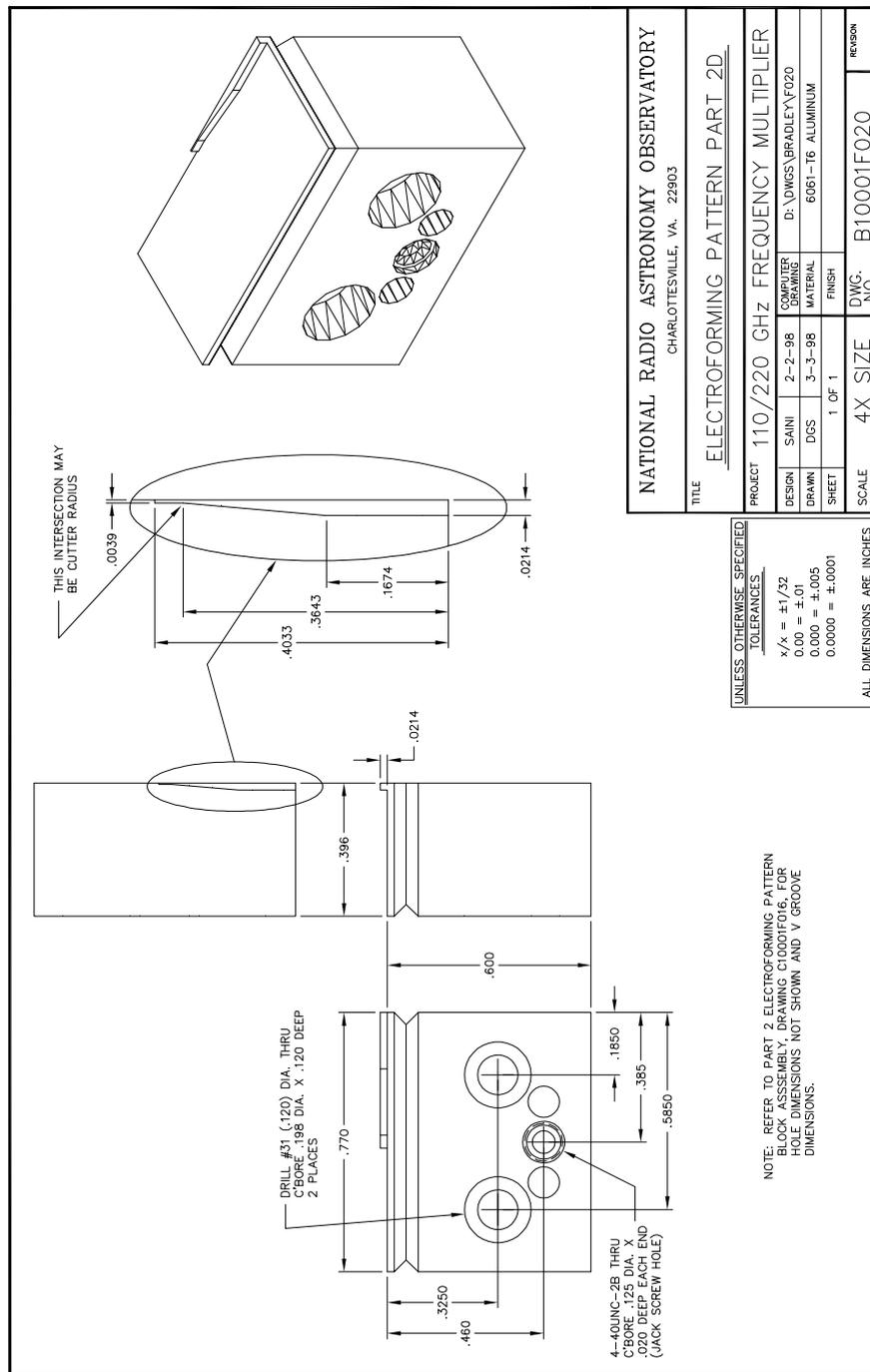
Figure D.29: 110/220 GHz frequency doubler: Mechanical details of the mandrel part 2D.
