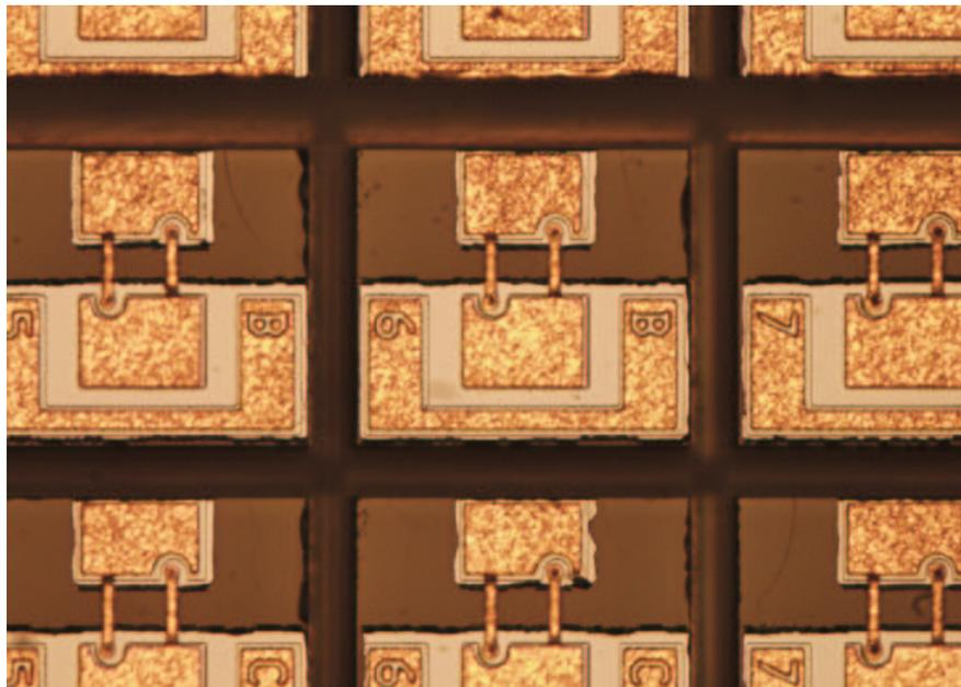
**Figure 3.2:** Photograph of the diced wafer prior to backside lapping to achieve chip separation. Photograph courtesy Gerhard S. Schoenthal, University of Virginia, Semiconductor Development Laboratory.
