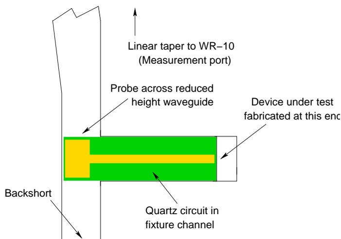
**Figure 3.8:** Cut away view of the test fixture, showing the placement of quartz circuit with the device under test inside.
