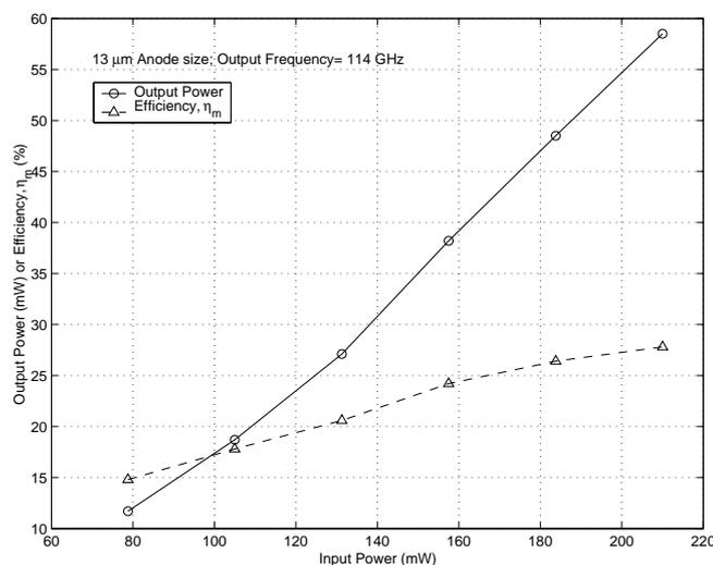
**Figure 2.28:** Measured output power and efficiency versus input pump power for an output frequency of 114 GHz.
