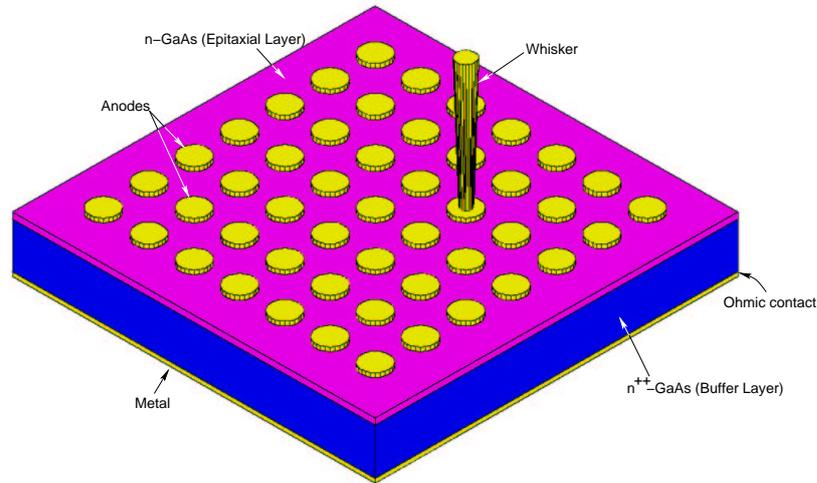
**Figure A.1:** Whisker contacted abrupt junction Schottky diode.
