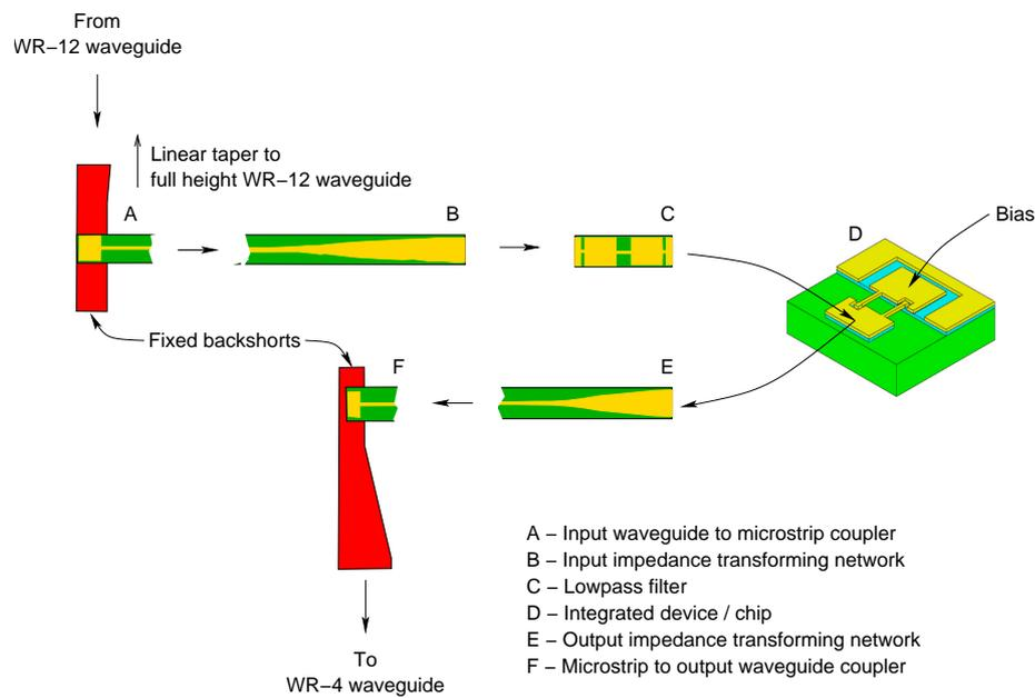
**Figure 4.4:** Relative placement of various components used in the 80/240 GHz frequency tripler.
