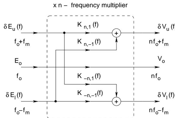
**Figure 5.1:** Transmission of sideband noise through a frequency multiplier, considered as a linear frequency converter.
