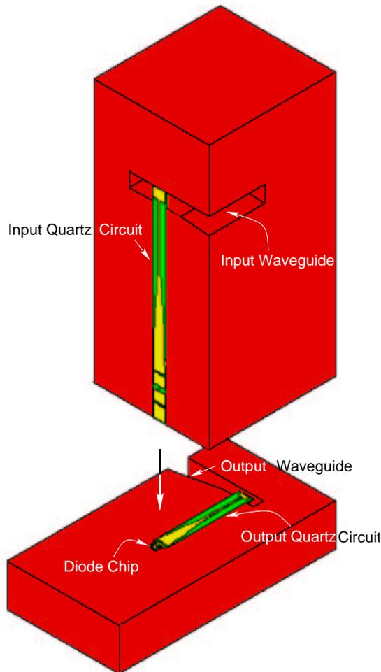
**Figure E.5:** Cut away view of the relevant pieces of the metal housing showing the relative placement of the diode chip, the input quartz circuit and the output quartz circuit. The DC bias arrangement located adjacent to the diode chip is not shown.
