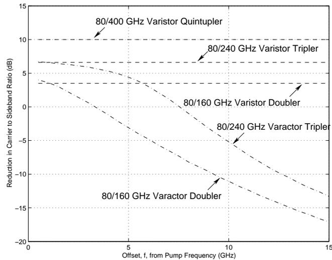
**Figure 5.4:** Plot of the degradation in carrier-to-sideband ratio for various frequency multipliers.
