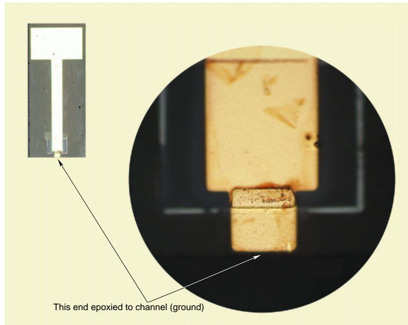
**Figure 3.7:** Photograph of 2 mil thick quartz circuit showing the test capacitor at one end of the microstrip transmission line. The waveguide probe is visible as a “flag” structure on the other end of the microstrip.
