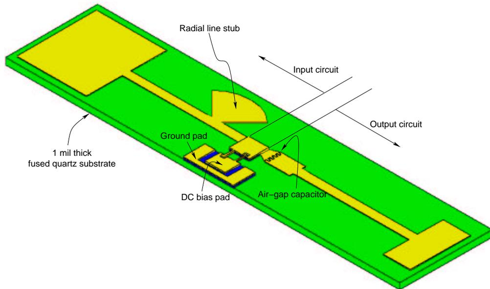
**Figure 4.39:** Layout of the 80/240 GHz frequency tripler as a MMIC chip. The embedding circuits may be fabricated integrally as shown on the extended GaAs-membrane-on-quartz substrate after the removal of GaAs from appropriate regions.
