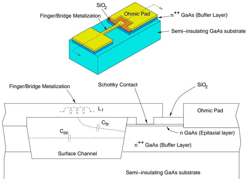
**Figure 2.4:** Details of a planar Schottky varactor.
