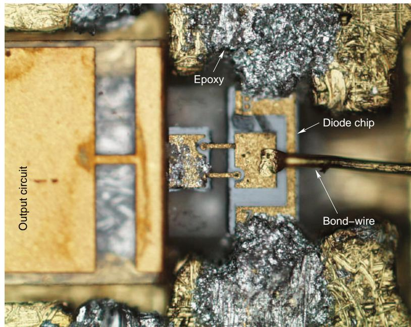
**Figure E.6:** Photo of the metal block showing the diode chip and the output circuit. A portion of the bond wire used for supplying the DC bias to the chip can be seen. The location of silver epoxy used to ground the chip pads is marked.
