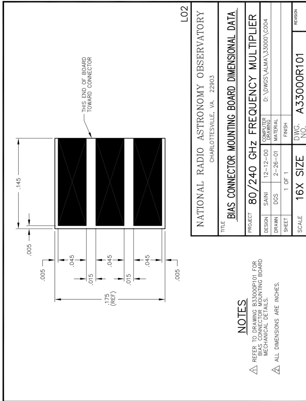
**Figure B.9:** Dimensional details of the artwork representing the metalization pattern on an individual DC bias board used in the 80/240 GHz frequency tripler.
