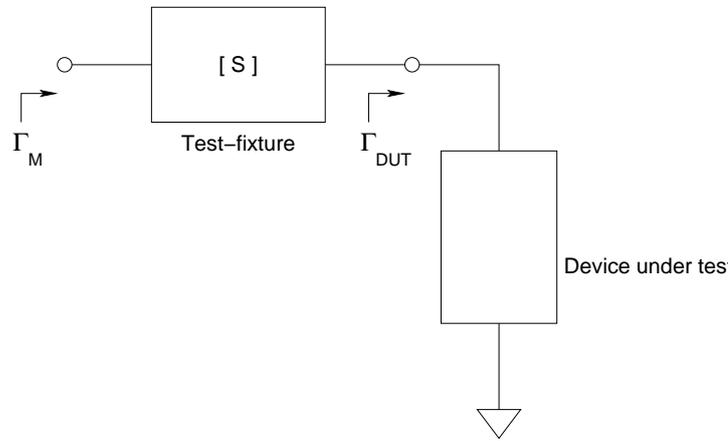
**Figure 3.9:** Block diagram of the experimental setup.
