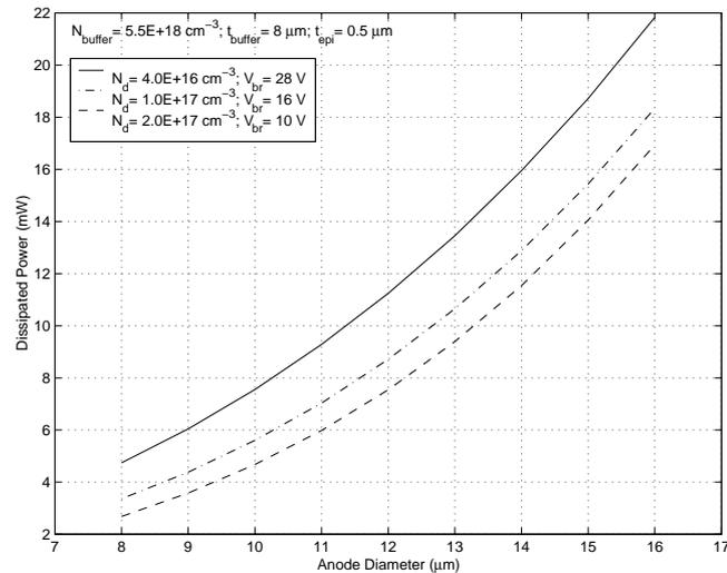
**Figure 2.11:** Power dissipated (per diode) under conditions of optimum operation for different anode sizes and epitaxial layer doping level.
