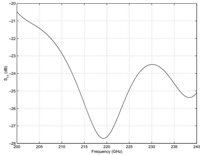
**Figure 2.37:** Plot of  $S_{11}$  for the complete output coupling arrangement, including the microstrip to one-fifth height waveguide probe, DC-bias filter and the one-fifth height to full height taper (simulated).
