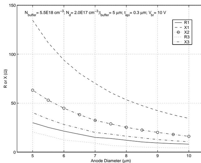
**Figure 4.9:** Optimum embedding impedances as a function of anode size.
