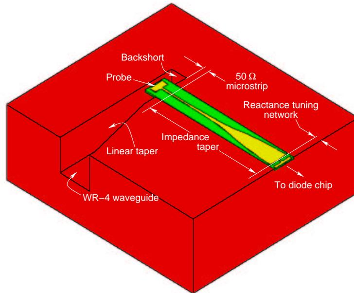
**Figure 4.22:** The output embedding circuit consisting of a microstrip impedance taper and a microstrip to waveguide transition. Only the bottom part of the mount that seats the quartz circuit is shown.
