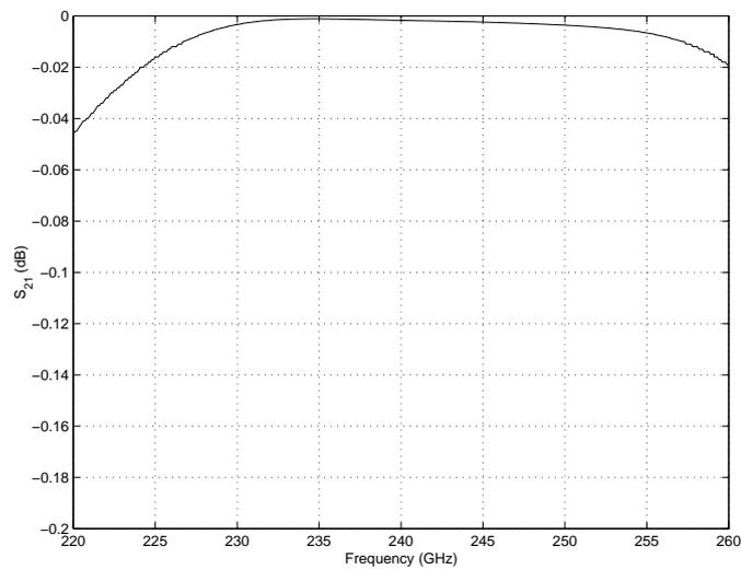
**Figure 4.29:** Plot of  $S_{21}$  for the complete 80/240 GHz frequency tripler output circuit (simulated).
