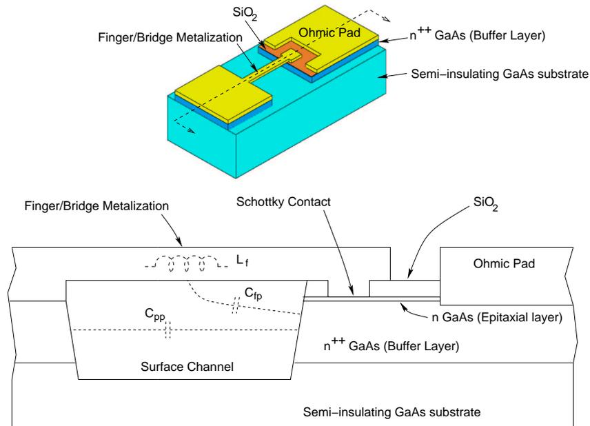
**Figure A.2:** Planarized abrupt junction Schottky diode.
