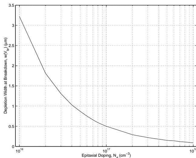
**Figure 2.12:** Variation of the width of the depleted region in the epitaxial layer at before breakdown as a function of epitaxial doping level.
