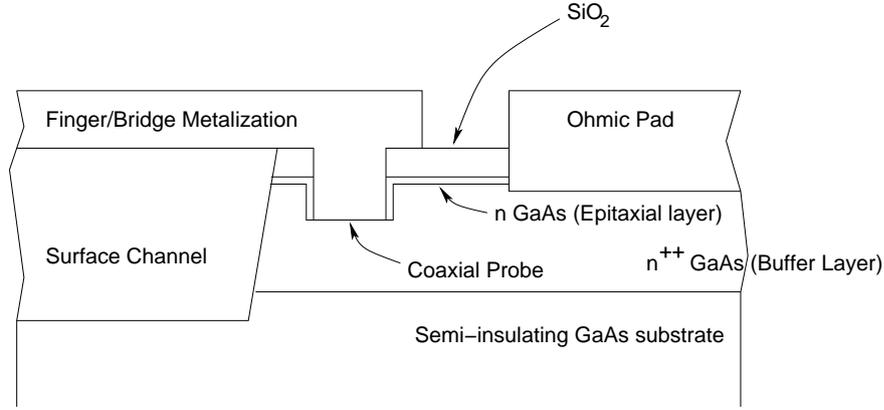
**Figure 2.16:** The coaxial probe geometry employed to calculate the impedance at the location of the Schottky junctions.
