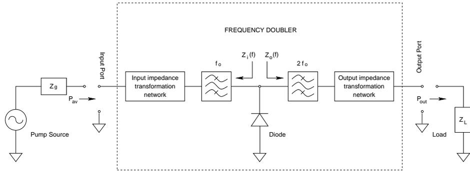
**Figure 2.1:** A single diode based frequency doubler.
