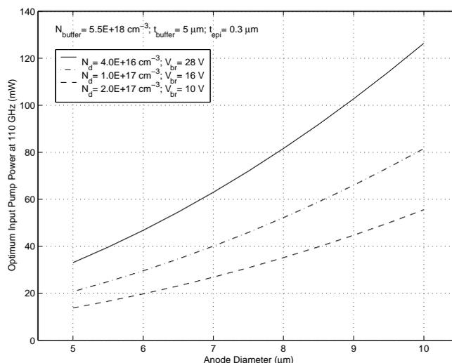
**Figure 2.30:** Input power (per diode) to obtain maximum conversion efficiency, for different anode sizes and epitaxial layer doping level.
