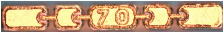
**Figure 2.34:** A Photograph of the UVA SB7T7 discrete planar Schottky varactor array used for the 110/220 GHz frequency doubler design.
