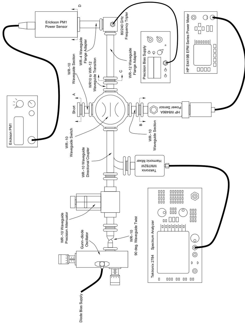
**Figure 4.32:** Experimental setup for evaluation of the 80/240 GHz frequency tripler.
