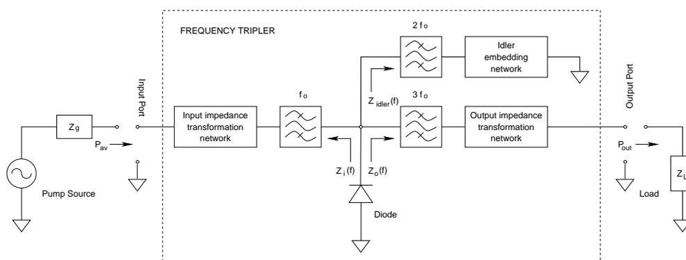
**Figure 4.1:** A single diode based frequency tripler.
