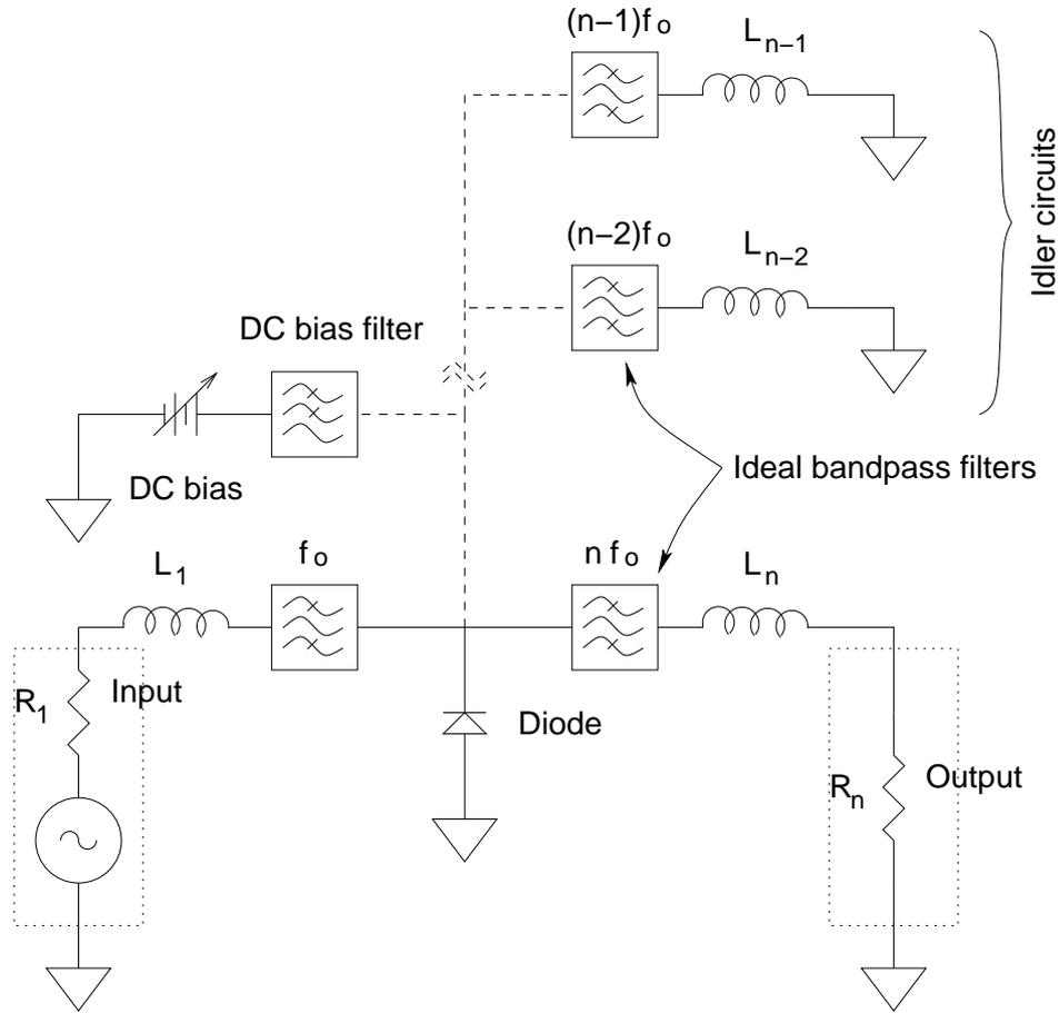
**Figure 5.3:** Generalized configuration of the circuit used in two-tone harmonic balance simulations to evaluate the up-conversion of amplitude-noise sidebands in  $\times n$  single-diode frequency multipliers. The idler and bias circuits were used, as appropriate, for setting up various frequency multiplier simulations.
