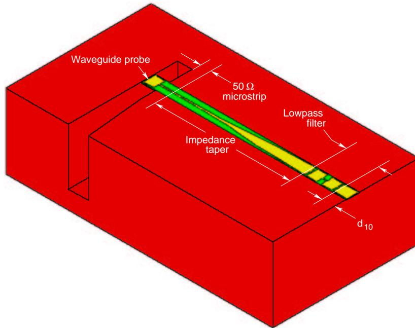
**Figure 4.19:** The complete input embedding circuit consisting of a waveguide to microstrip transition, a microstrip impedance taper and a lowpass filter. Only the bottom part of the mount that seats the quartz circuit is shown. The length of the section marked  $d_{10}$  was optimized such that the impedance presented to the diode chip was close to an open circuit at the output frequency of 240 GHz.
