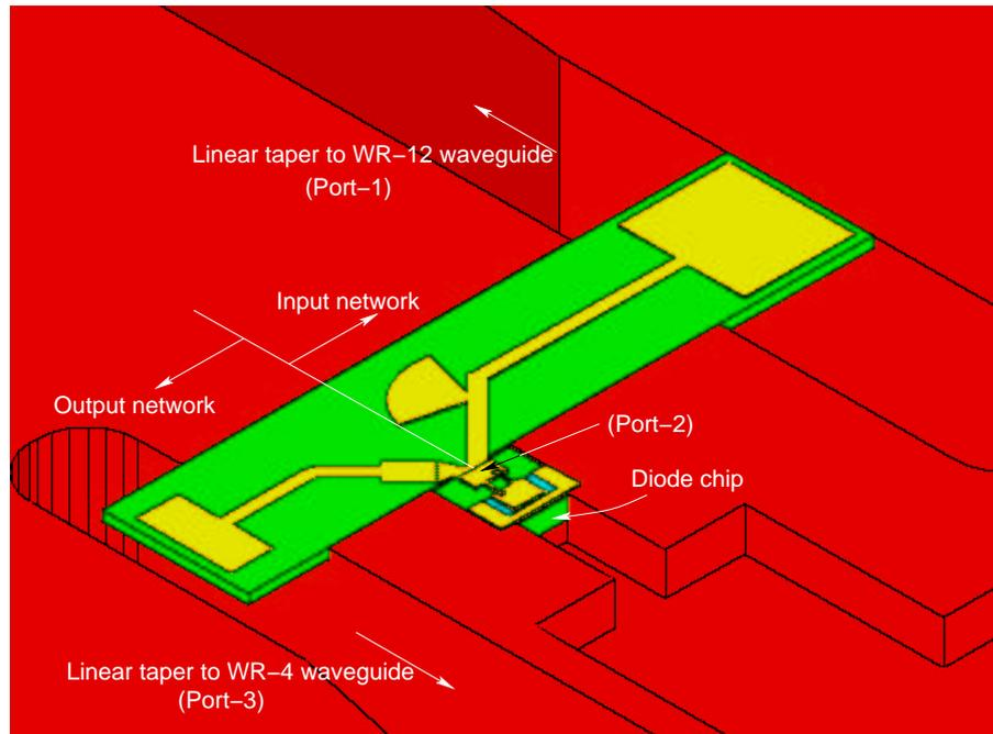
**Figure 4.35:** Layout of the input and output embedding circuits, integrated onto a single quartz substrate. Also illustrated is the placement of the quartz circuit relative to important features on the metal block as well as the diode chip. Only bottom half of the mount that seats the circuits is shown.
