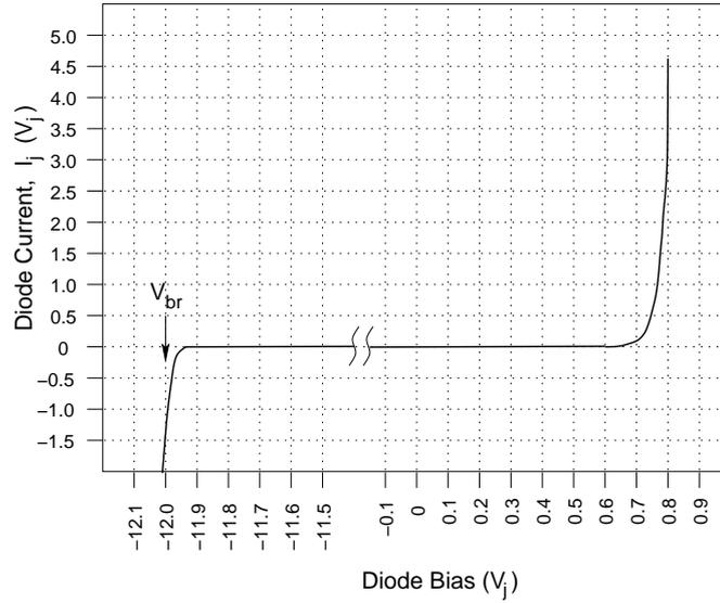
**Figure 2.5:** Typical Current-Voltage relationship for a Schottky varactor.
