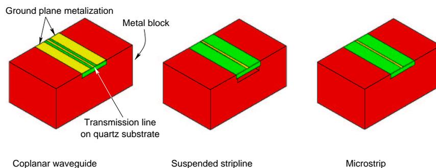
**Figure 3.3:** Planar transmission line structures.
