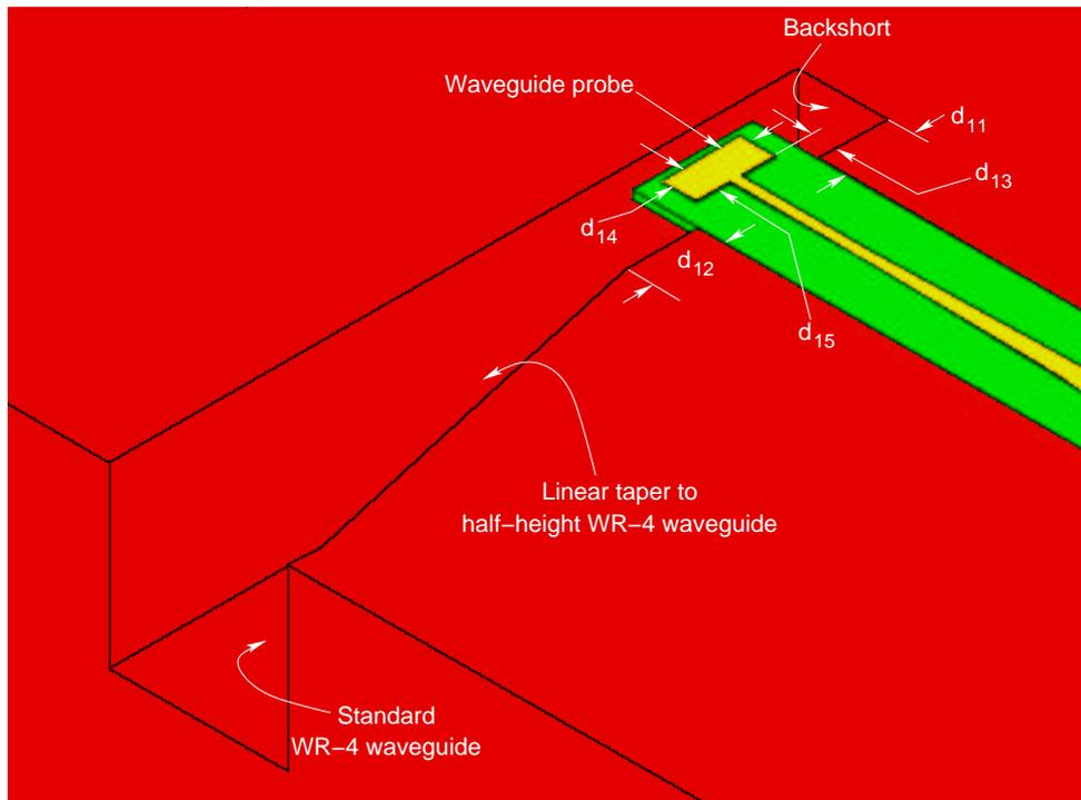
**Figure 4.24:** Design of the output coupler for the 80/240 GHz frequency tripler. Only bottom part of the mount that seats the quartz circuit is shown. The dimensions that were optimized to achieve a good coupling efficiency are marked.
