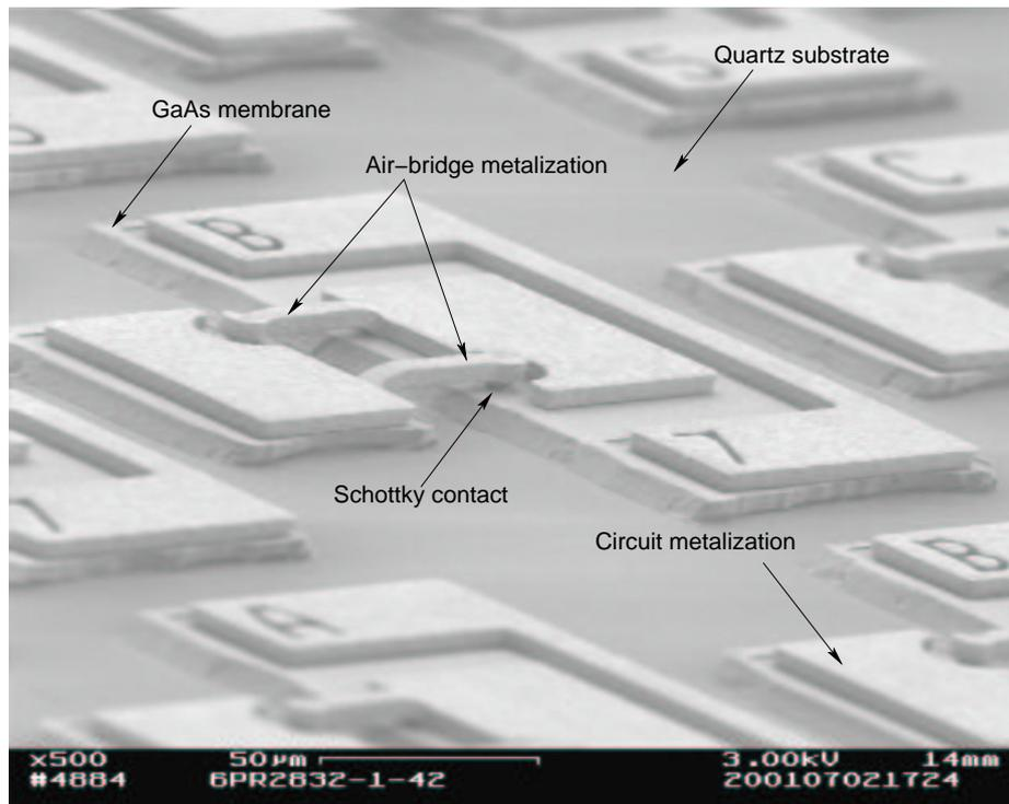
**Figure 3.1:** A Scanning Electron Micrograph of an undiced wafer fabricated based on the composite GaAs-membrane-on-quartz approach. Photograph courtesy Gerhard S. Schoenthal, University of Virginia, Semiconductor Development Laboratory.
