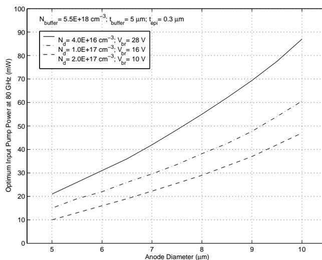
**Figure 4.7:** Input power (per diode) to obtain maximum conversion efficiency, for different anode sizes and epitaxial layer doping level.
