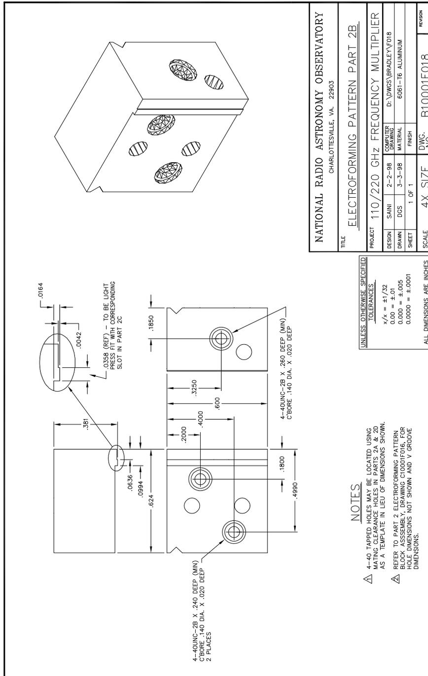
Figure D.27: 110/220 GHz frequency doubler: Mechanical details of the mandrel part 2B.
