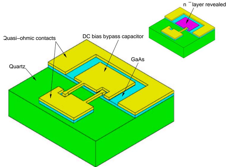
**Figure 4.5:** Layout of the quartz based integrated device, consisting of two Schottky diodes in an anti-parallel configuration and a large capacitor to accommodate the DC bias arrangement. The smaller inset is a view with the top metalization of capacitor removed to reveal the  $n^-$  layer underneath.
