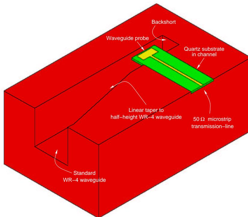
**Figure 3.4:** The microstrip to WR-4 waveguide transition. Figure shows a cut-away view of the arrangement. Only the bottom half of the block is illustrated, revealing the placement of the quartz circuit in the metal housing.
