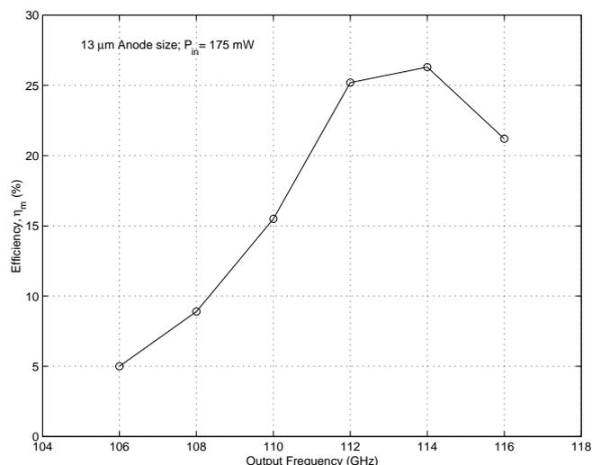
**Figure 2.26:** Measured conversion efficiency of the 55/110 GHz frequency doubler using a diode array with  $13 \mu m$  diameter anodes.
