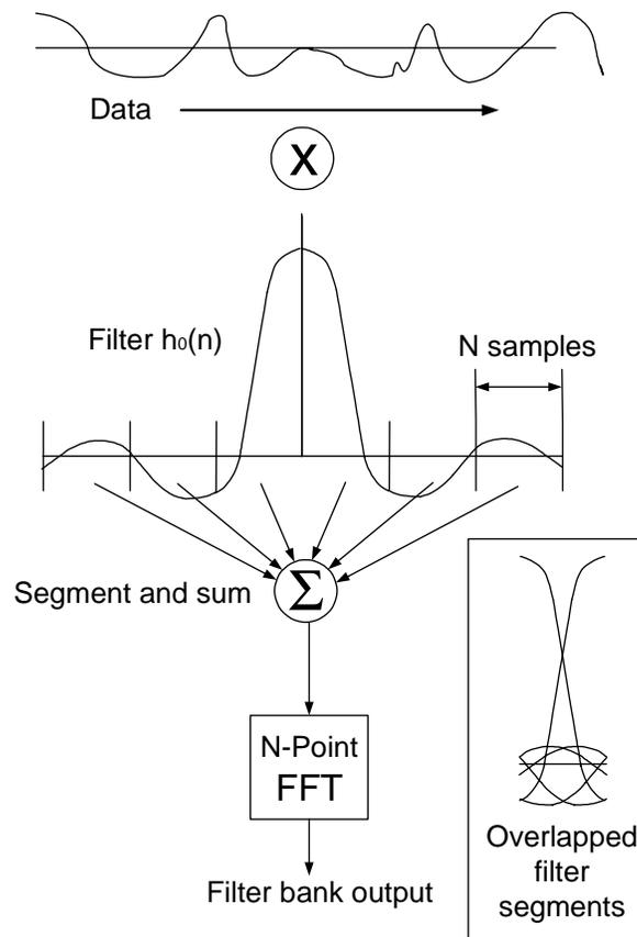
**Figure 4 Diagrammatic representation of the operation performed by the system shown in Figure 3.**
