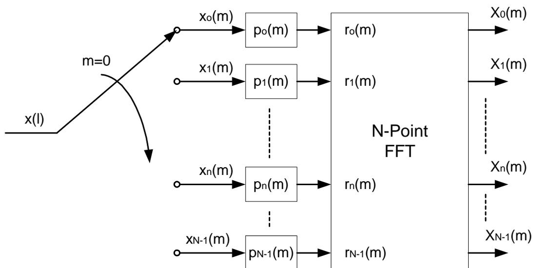
**Figure 2 DFT filterbank with arbitrary frequency response**
