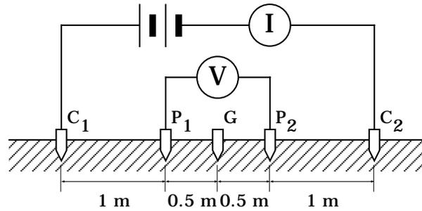
Figure 1: The Wenner electrode configuration. Current is injected into the ground through a pair of current electrodes ( $C_1$  and  $C_2$ ), and the potential difference is measured between a pair of potential electrodes ( $P_1$  and  $P_2$ ). Depth of the electrodes was set at about 10 cm.
