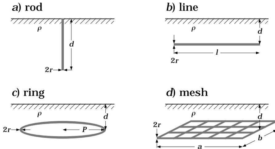
Figure 5: Configurations of prototypical grounding methods: (a) a rod, (b) a line, (c) a ring, and (d) a mesh (mesh number 15).
