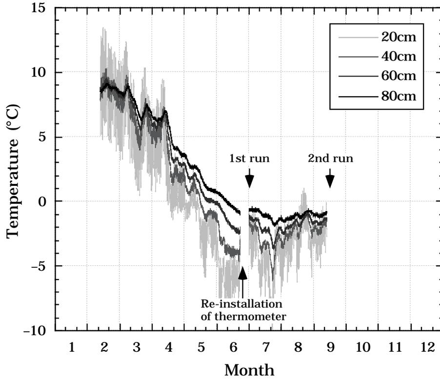
Figure 4: Subsurface temperature measured at Pampa La Bola (4800 m) during the year of 2000 as a function of depth [3]. Periods of our previous and present measurements are shown with arrows.
