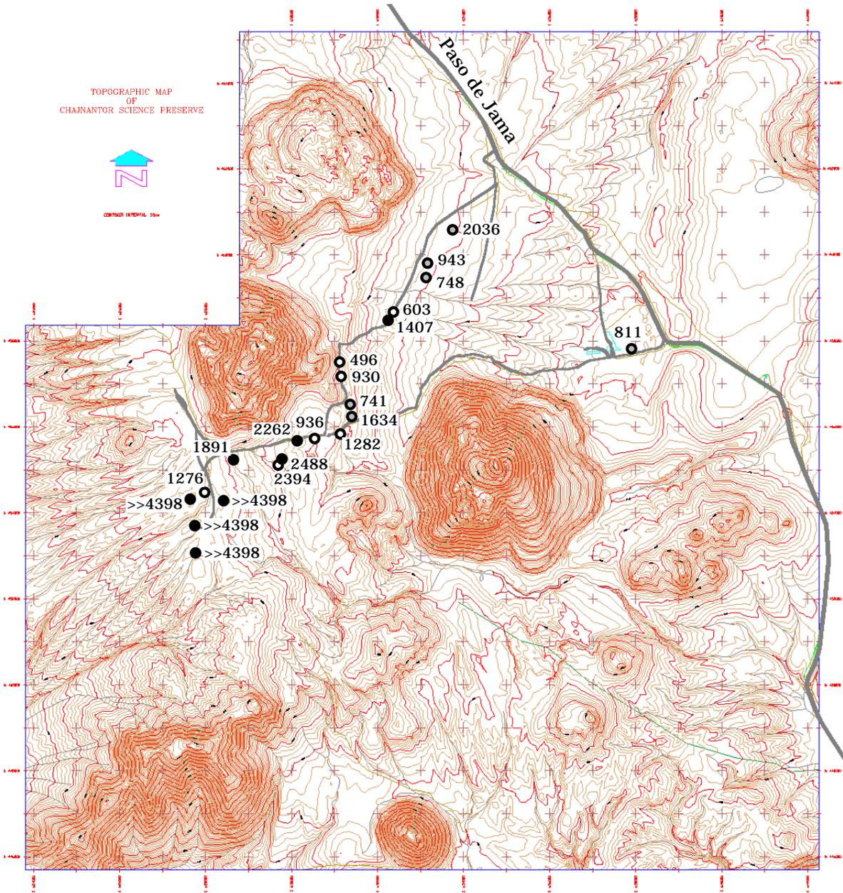
Figure 2: Apparent resistivity at the twenty-one locations measured with a fixed Wenner electrode spacing (2 m), overlaid on the topographic map of the Cerro Chascón science preserve area [2]. Filled circles, shaded circles, and open circles indicate that the topography of the corresponding location is ridge, flat, or valley, respectively. The absolute coordinates in this map may contain errors up to a few 100 m. Ticks are spaced by 1 km. Contour spacing is 10 m with thick contours every 50 m.
