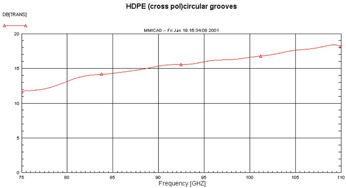
**Figure 21** Cross polar increase with circular rectangular grooves on both sides.
