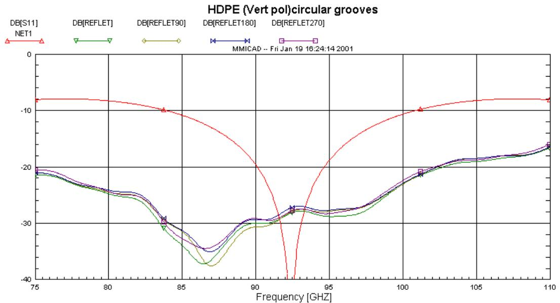
**Figure 16** Reflection of HDPE with circular rectangular grooves on both sides at rotation angles 0, 90, 180, and 270 degrees. NET1 (red line) is the theoretical curve for an unmatched layer.
