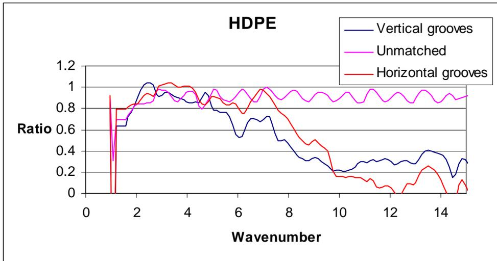
**Figure 24** FTS spectra of grooved (linear rectangular both sides) and un-grooved HDPE, resolution 7 GHz (1 wavenumber = 30 GHz).
