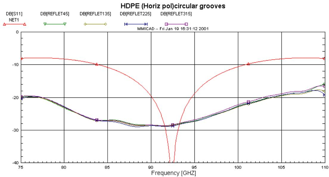
**Figure 20** Reflection of HDPE with circular rectangular grooves on both sides at rotation angles 45, 135, 225, and 315 degrees. NET1 (red line) is the theoretical curve for an unmatched layer.
