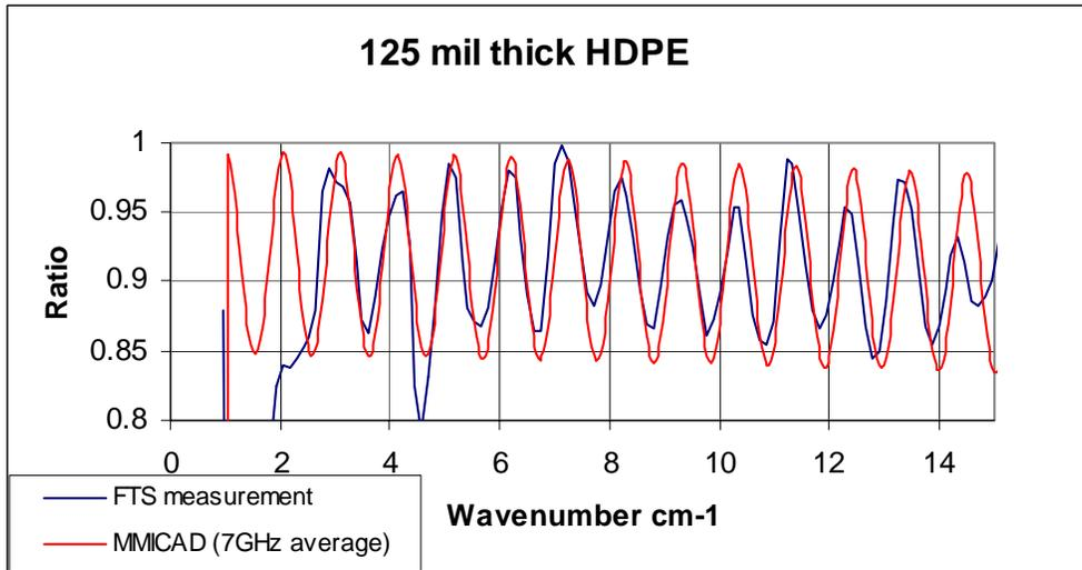
**Figure 23** FTS and MMICAD calculations (averaged over 7 GHz) including loss of a 125 mil thick piece of HDPE (1 wavenumber = 30 GHz).
