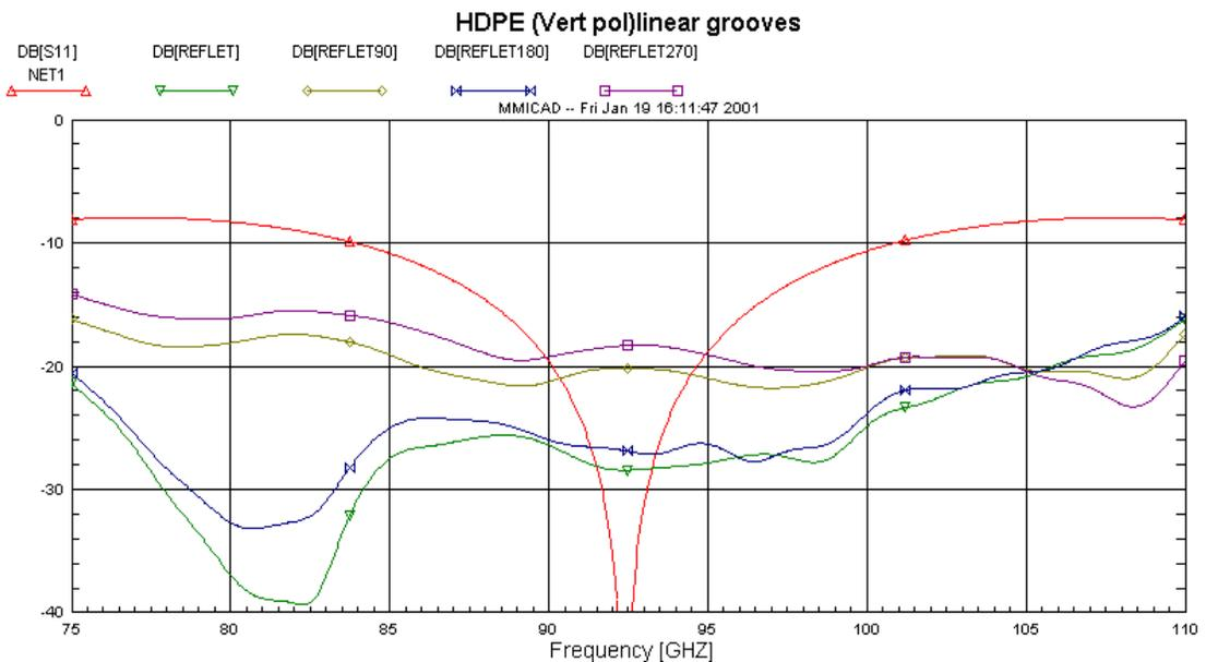
**Figure 10** Measured reflection of HDPE with linear rectangular grooves on both sides for various rotation angles for vertically polarized sources. NET1 (red line) is the theoretical curve for an unmatched layer.
