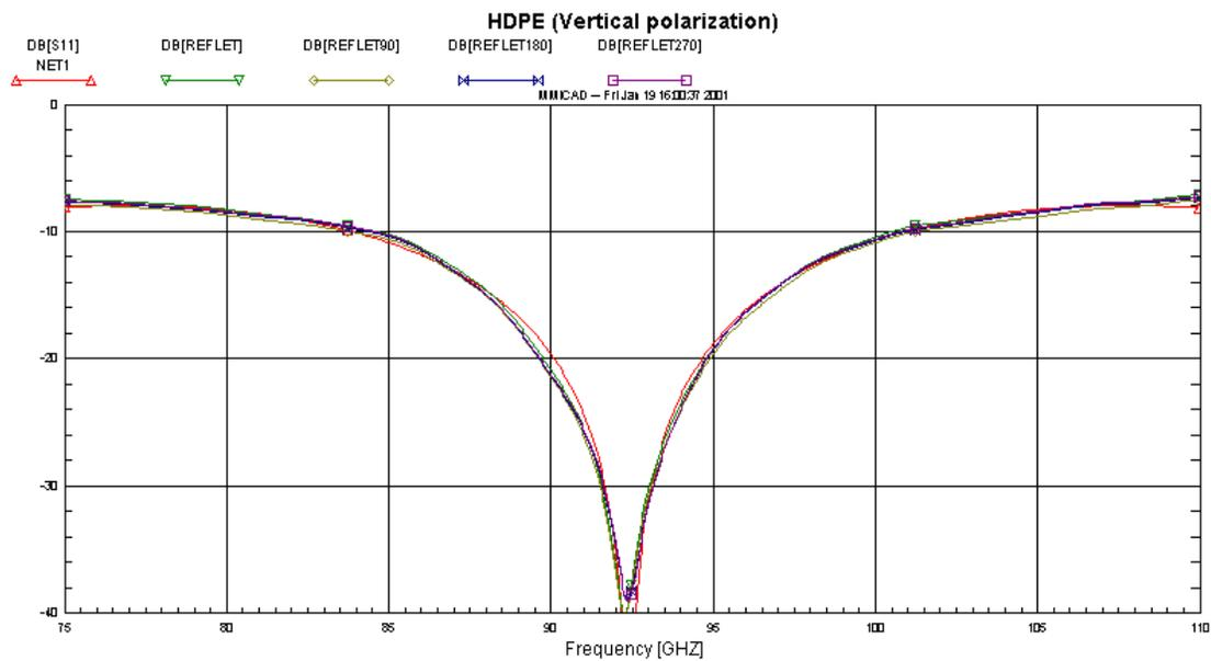
**Figure 2** Reflection of a 3.16 mm thick piece of HDPE for 4 rotation angles. Net1 (red) curve is the theoretical response.
