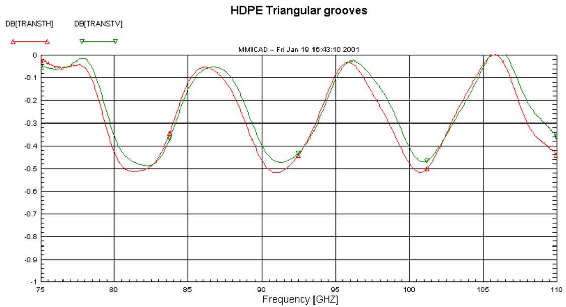
**Figure 27** Transmission of HDPE with triangular grooves on one face. Red line horizontal, green line vertical.
