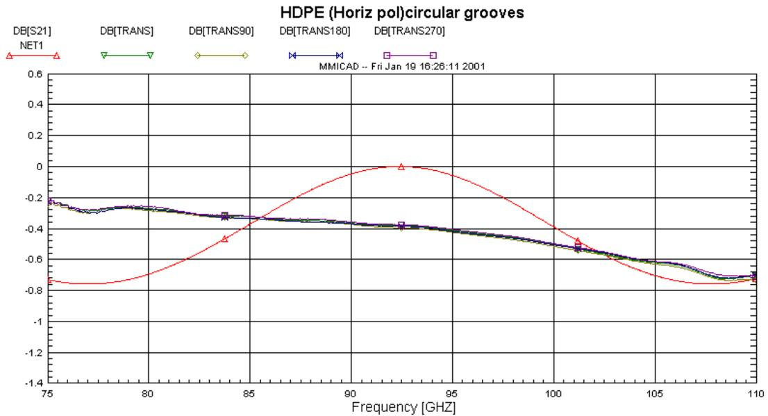
**Figure 17** Transmission of HDPE with circular rectangular grooves on both sides at rotation angles 0, 90, 180 and 270 degrees. NET1 (red line) is the theoretical curve for an unmatched layer.
