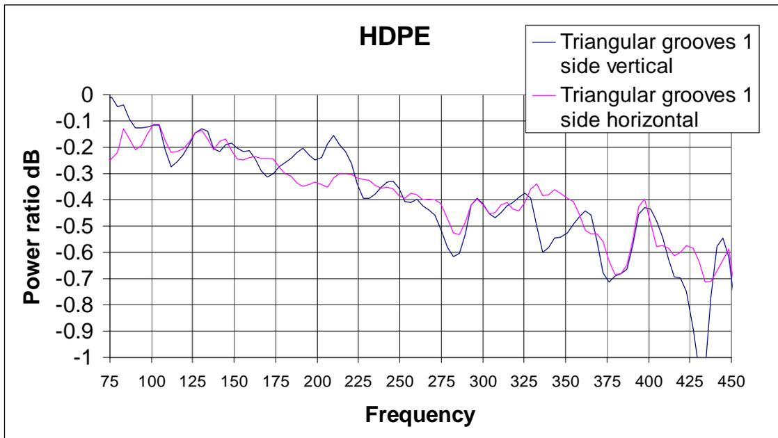
**Figure 26** FTS spectra of HDPE with triangular grooves on one face.
