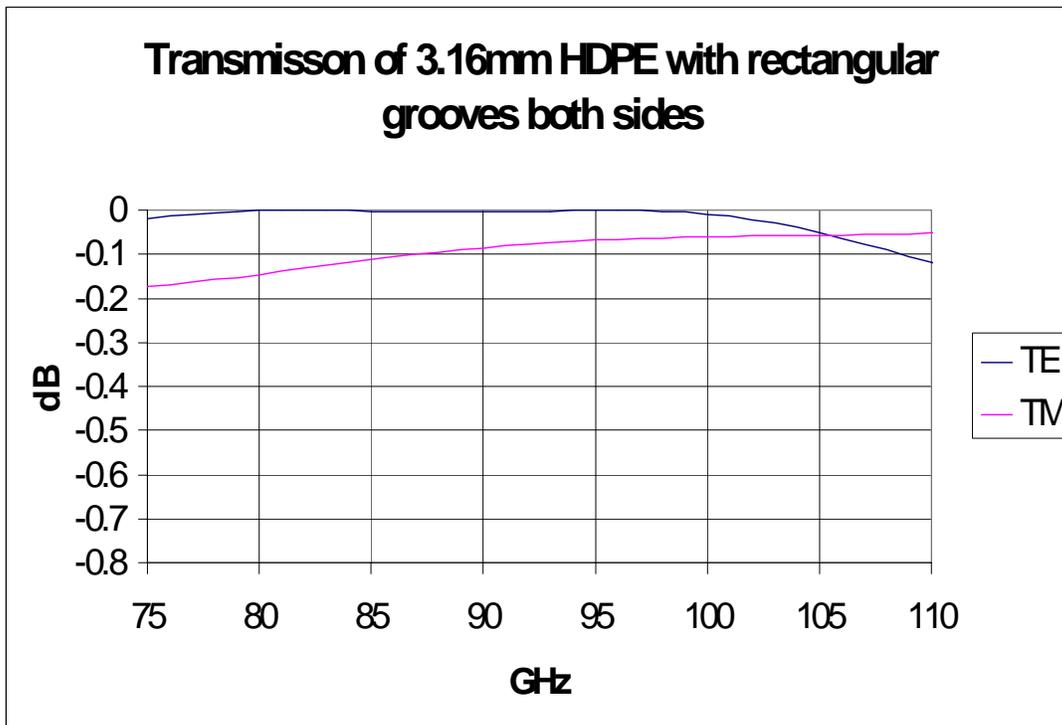
**Figure 7** Calculated transmission.
