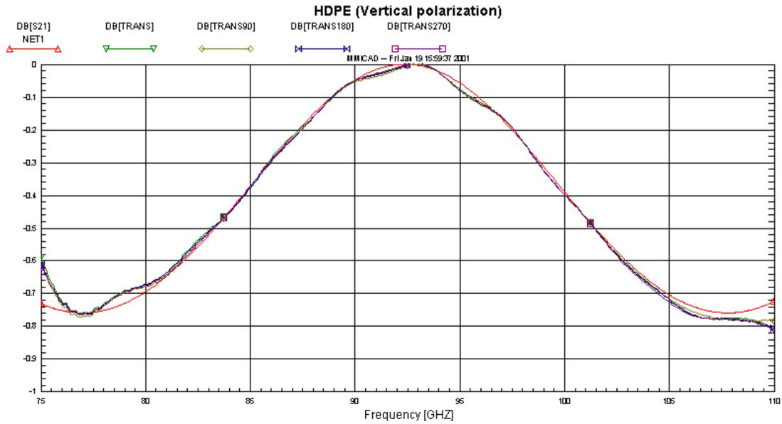
**Figure 1** Transmission of a 3.16mm thick piece of HDPE for 4 rotation angles. Net1 (red) is the theoretical response.
