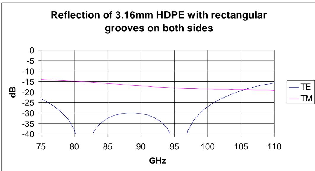
**Figure 8** Calculated reflection.
