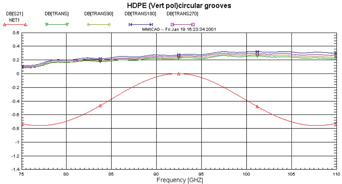
**Figure 15** Transmission of HDPE with circular rectangular grooves on both sides at rotation angles 0, 90, 180, and 270 degrees. NET1 (red line) is the theoretical curve for an unmatched layer.
