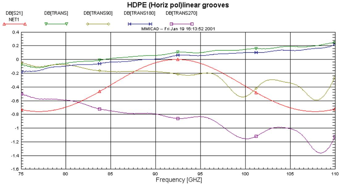
**Figure 11** Measured transmission of HDPE with linear rectangular grooves on both sides for various rotation angles for horizontally polarized sources. NET1 (red line) is the theoretical curve for an unmatched layer.
