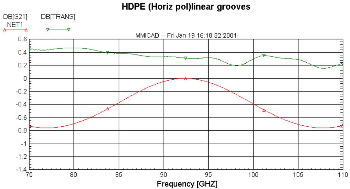
**Figure 13** “Optimized” transmission of HDPE with linear rectangular grooves on both sides. NET1 (red line) is the theoretical curve for an unmatched layer.
