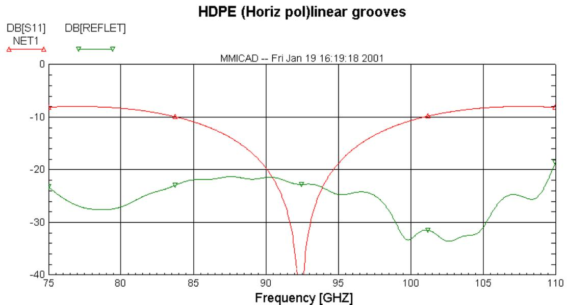
**Figure 14** “Optimized” reflection of HDPE with linear rectangular grooves on both sides. NET1 (red line) is the theoretical curve for an unmatched layer.
