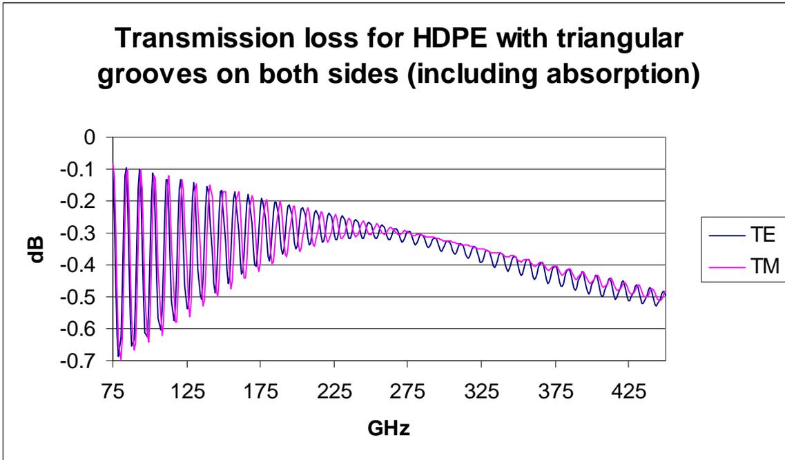
**Figure 25** Scatter calculation for the transmission loss of a 11mm thick piece of HDPE with triangular grooves on both sides (including absorption loss  $\tan\delta=0.0007$ , which over estimates loss at low frequency end [2]).
