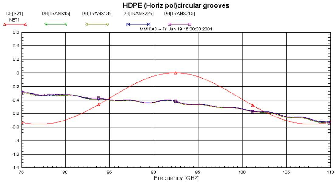
**Figure 19** Transmission of HDPE with circular rectangular grooves on both sides at rotation angles 45, 135, 225 and 315 degrees. NET1 (red line) is the theoretical curve for an unmatched layer.
