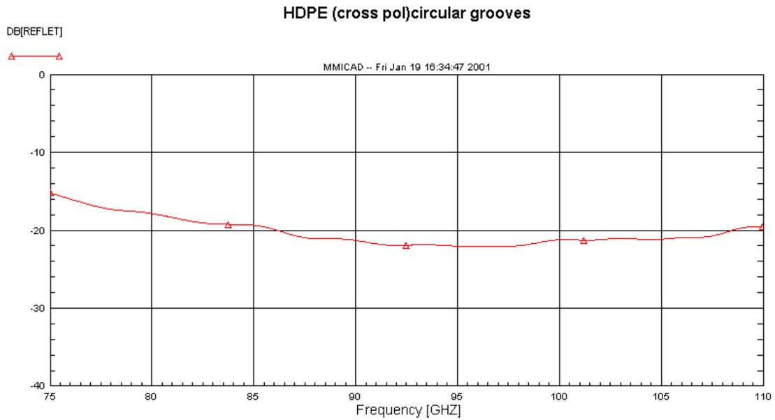
**Figure 22** Cross-polar reflection for circular rectangular grooves on both sides.
