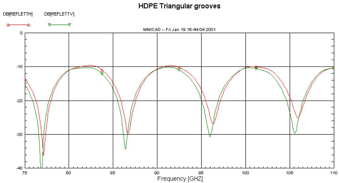
**Figure 28** Reflection of HDPE with triangular grooves on one face. Red line horizontal, green line vertical.
