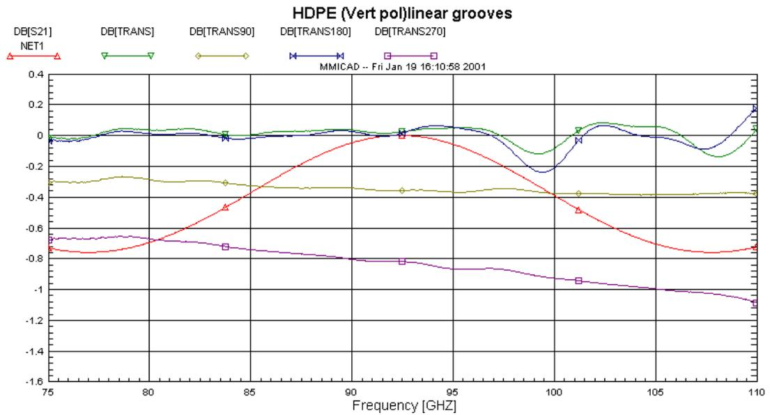
**Figure 9** Measured transmission of HDPE with linear rectangular grooves on both sides for various rotation angles for vertically polarized sources. NET1 (red line) is the theoretical curve for an unmatched layer.
