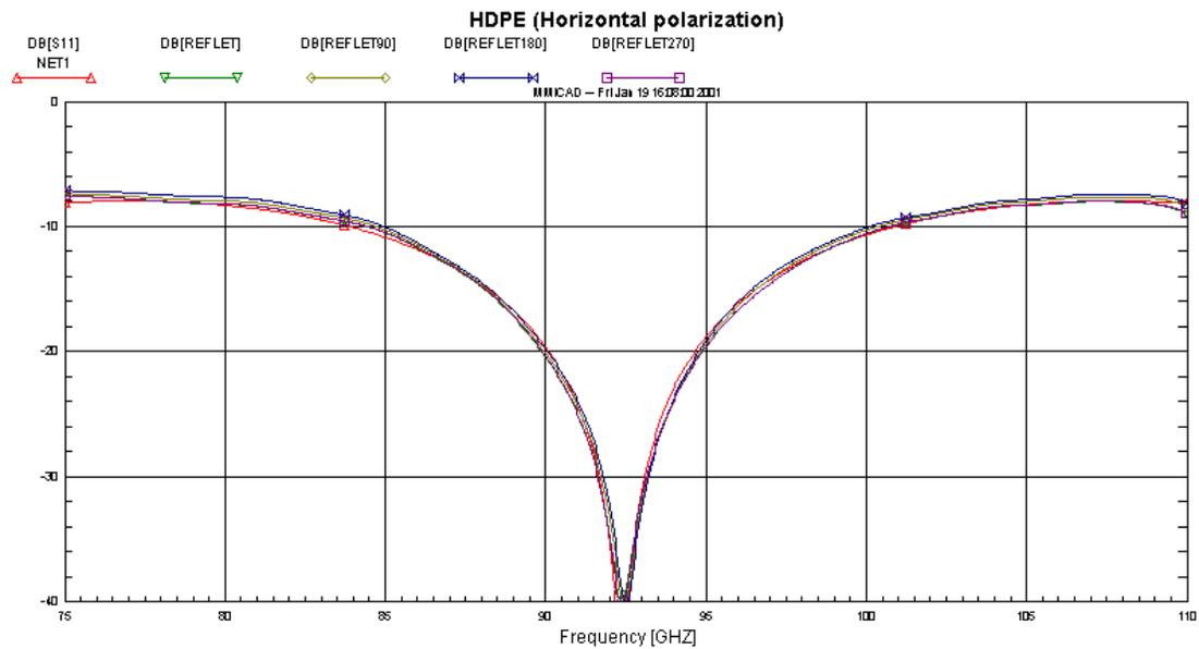
**Figure 4** Reflection of a 3.16 mm thick piece of HDPE for 4 rotation angles. NET1 (red) curve is the theoretical response.
