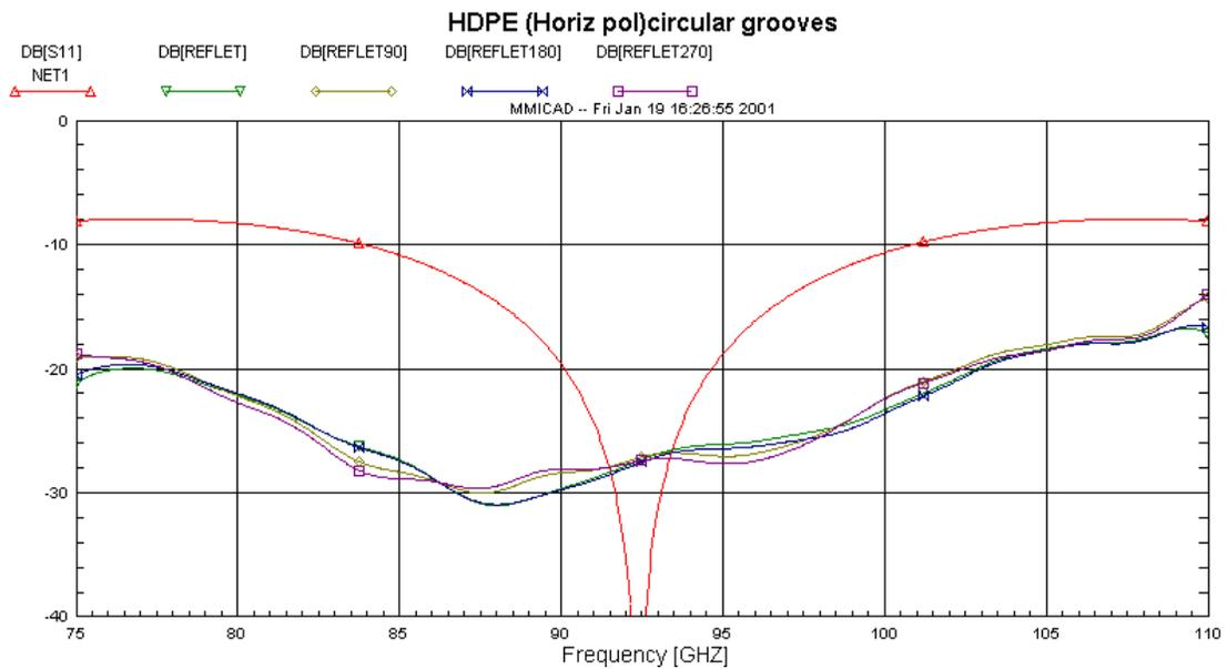
**Figure 18** Reflection of HDPE with circular rectangular grooves on both sides at rotation angles 0, 90, 180, and 270 degrees. NET1 (red line) is the theoretical curve for an unmatched layer.
