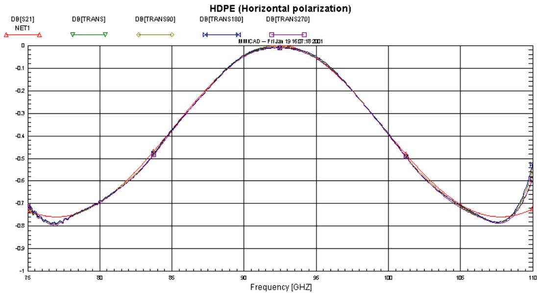
**Figure 3** Transmission of a 3.16 mm thick piece of HDPE for 4 rotation angles. NET1 (red) curve is the theoretical response.
