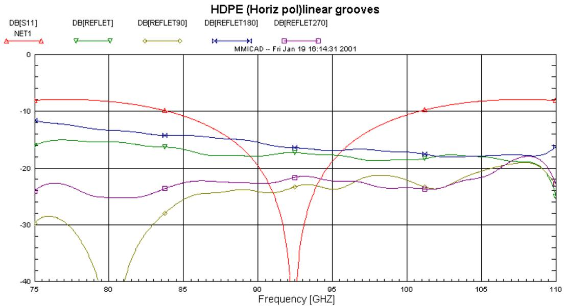
**Figure 12** Measured reflection of HDPE with linear rectangular grooves on both sides for various rotation angles for horizontally polarized sources. NET1 (red line) is the theoretical curve for an unmatched layer.
