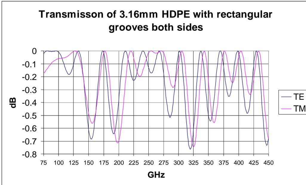
**Figure 5** Calculated transmission.
