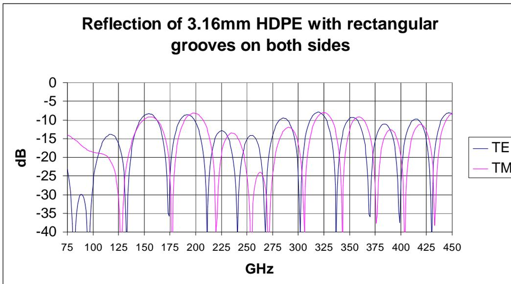
**Figure 6** Calculated reflection.
