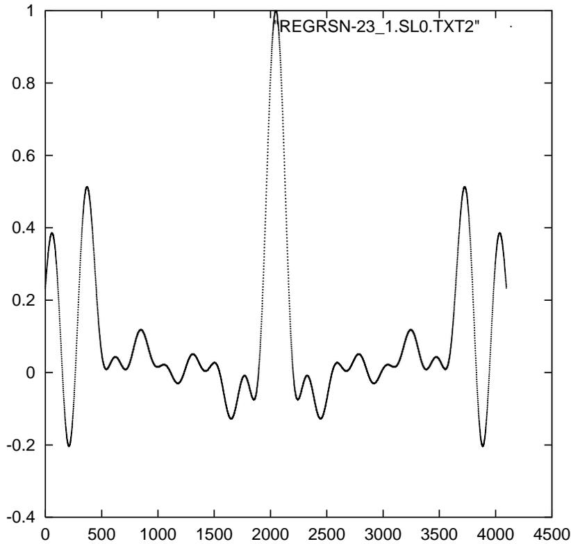
Figure 6: Cross sectional plot of slice at 0 degrees through synthetic beam of perturbed square array
