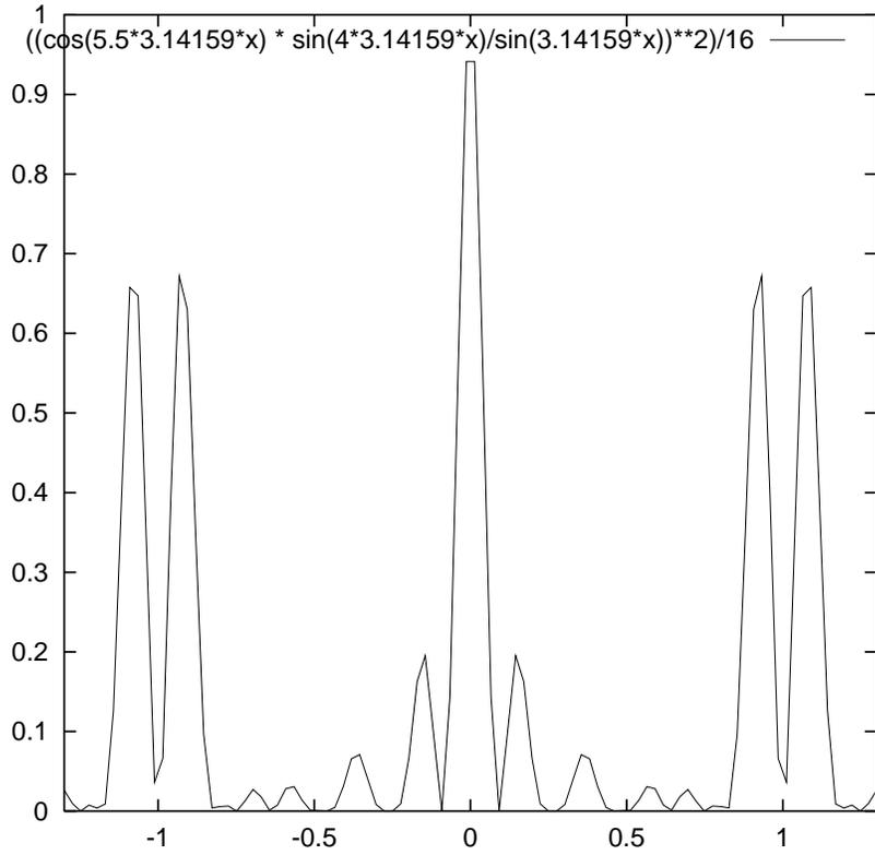
Figure 5: Cross sectional plot of model 1-d perturbed array's power spectrum
