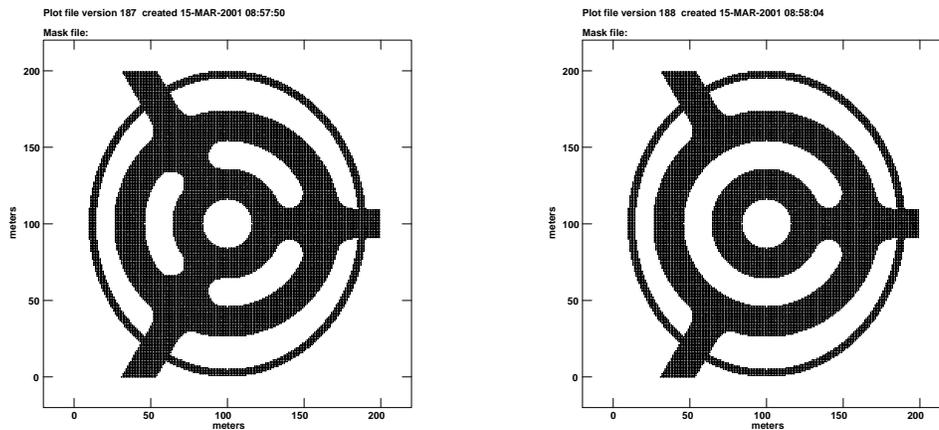
Figure 2: Examples of the roads with three radius. Only one radius goes to the inner circle at the right plot. That saves some room for antennas but complicates the driving. The width of the roads is 20m. The radius of the turns is 10m. The outside ellipse is not a road but a boundary that make antennas stay inside of the ellipse to make the configuration elongated at the N-S direction.
