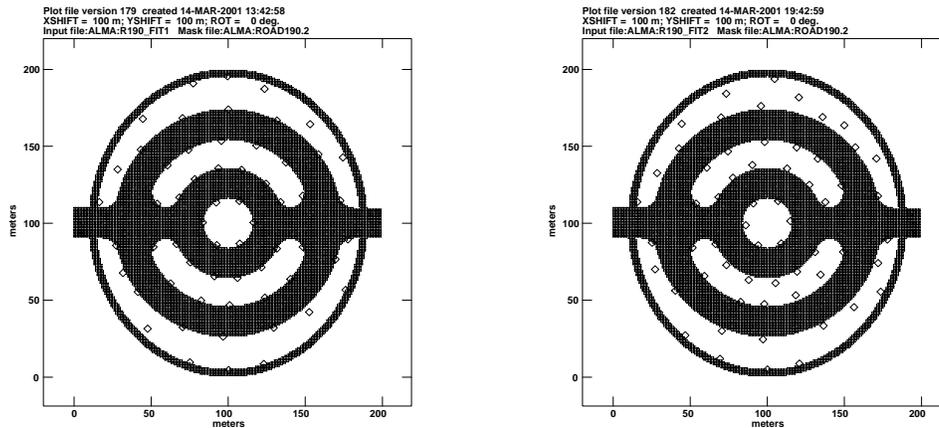
Figure 5: The configuration with the road width 20m. The maximum size of the configuration is 190m. The inner circle includes 6 antennas. Some antennas which the transporter passes by have to stop the observation. The configuration is 10%elongated at the N-S direction. The relevant optimization of the side lobe is carried out for the nearest side lobes (the left plots; side lobes  $\sim 0.01$ ) and for the total area of the primary beam (the right plot; side lobes  $\sim 0.052$ )
