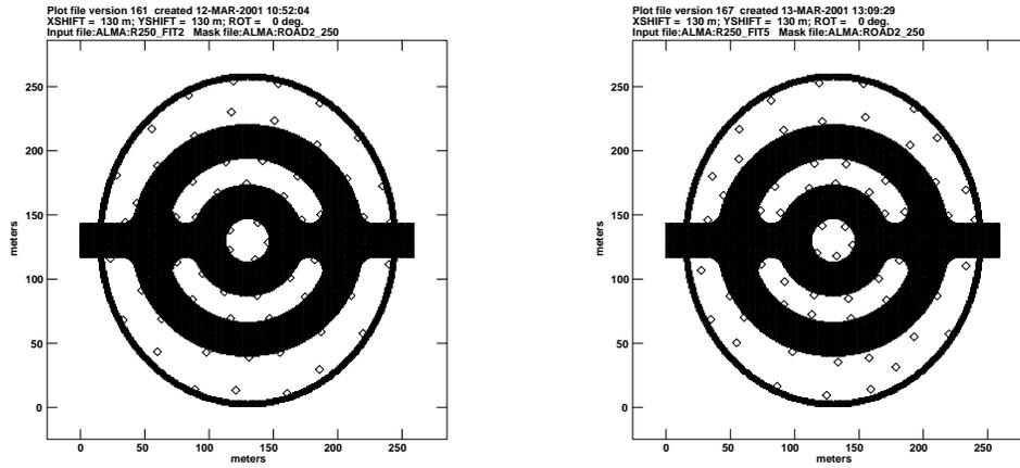
Figure 4: The configuration with the road width 27m. The maximum size of the configuration is 250m. The inner circle includes 5 antennas. All antennas can be reached by a transporter without stop of the observation. The configuration is 10%elongated at the N-S direction. The relevant optimization of the side lobe is carried out for the nearest side lobes (the left plots; side lobes  $\sim 0.009$ ) and for the total area of the primary beam (the right plot; side lobes  $\sim 0.048$ )
