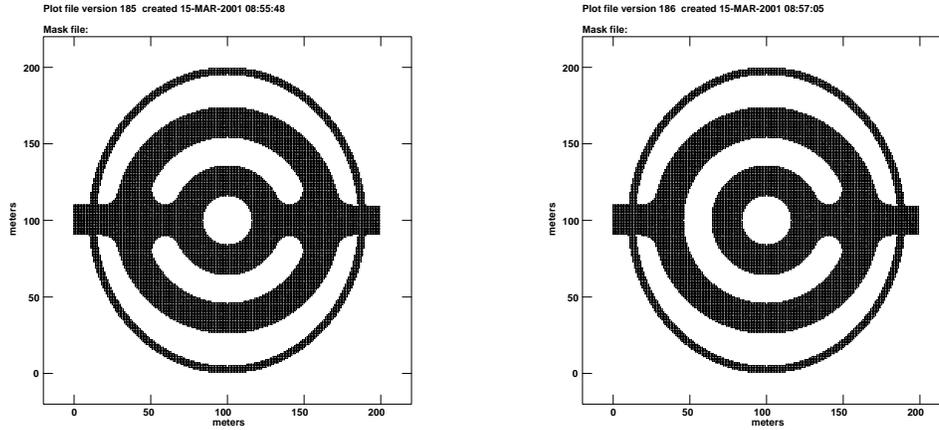
Figure 1: Examples of the roads with two radius. Only one radius goes to the inner circle at the right plot. That saves some room for antennas but complicates the driving. The width of the roads is 20m. The radius of the turns is 10m. The outside ellipse is not a road but a boundary that make antennas stay inside of the ellipse to make the configuration elongated at the N-S direction.
