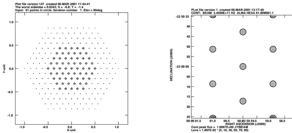
Figure 3: The hexagon tile configuration with 61 antennas at the left plot and its beam pattern at the right plot. The beam pattern shows 100% grating side lobes.
