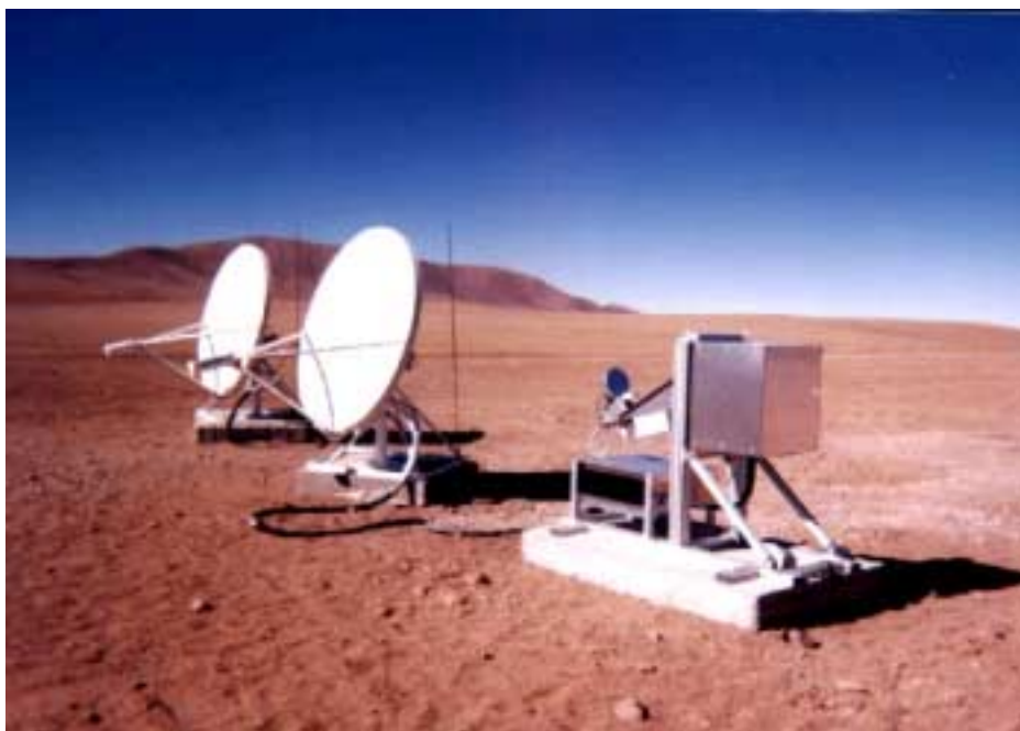
Fig 2.- The experimental setup at Chajnantor showing one end of the interferometer baseline. The 183 GHz radiometer is on the right, the ESO dish is at the centre and the NRAO dish on the left. The distance between the radiometer and the NRAO interferometer used for the experiment described here is of about 6 m.
