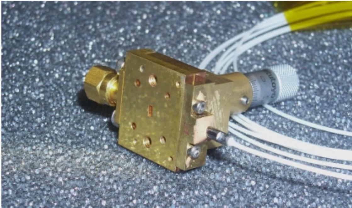
Fig. 2: Photograph of completed photonic sources showing the WR-10 output waveguide and the stainless steel fibre ferrule cemented to the block. The block base dimensions are 20 mm x 25 mm.
