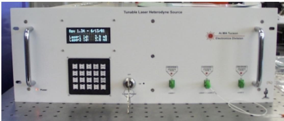
Fig. 3: Photograph of the front panel of the NRAO dual 1.55  $\mu\text{m}$  laser source. A keypad allows the user to set a difference frequency in the range from 1 GHz to 625 GHz
