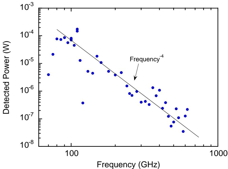
Fig. 5: Dependence of mm-wave power on frequency for a constant excitation power of +10 dBm. The line is a guide to the eye and indicates a frequency<sup>-4</sup> dependence
