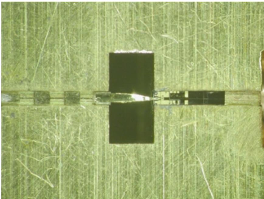
Fig. 1: Photograph of  $u^2t$  photodiode chip (right centre) incorporated in a photonic mixer block.
