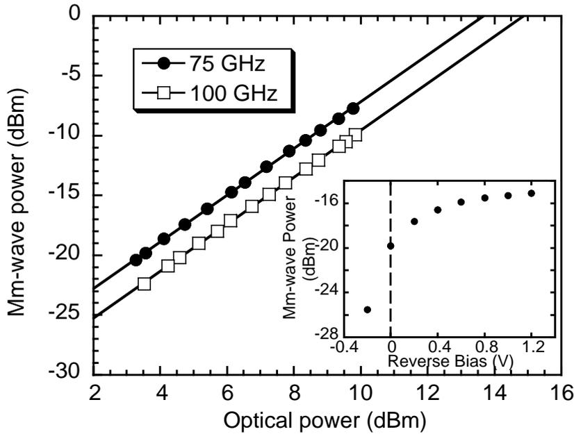
Fig. 4: Dependence of mm-wave power on optical power at frequencies of 75 GHz (solid circles) and 100 GHz (open squares) for a reverse bias of  $-1.2$  V. The lines indicate a slope of two. The inset shows the dependence of the mm-wave power on bias at a frequency of 100 GHz and an optical power of  $+7.8$  dBm.
