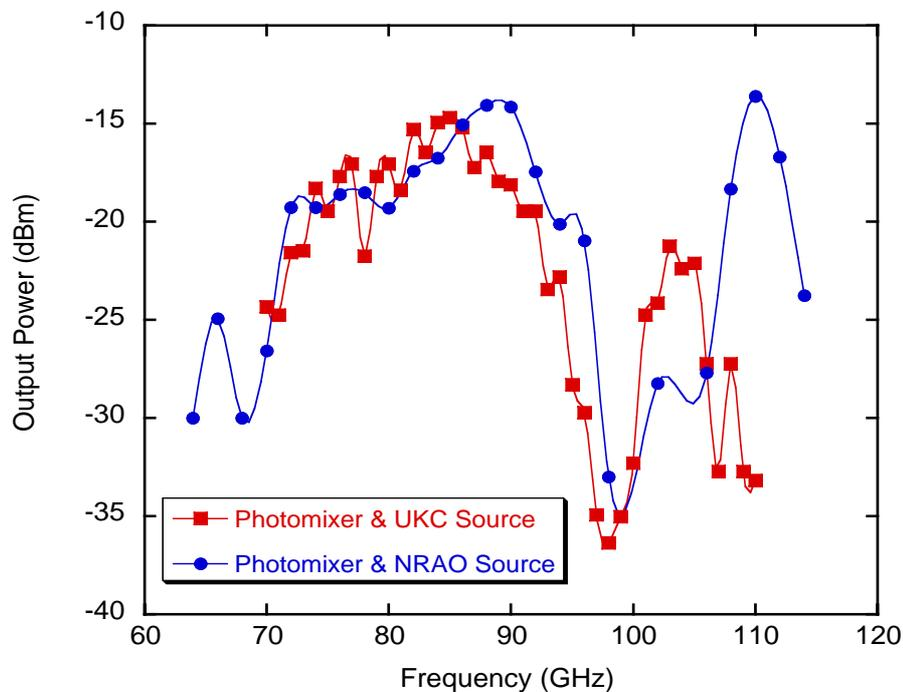
Fig. 6: Comparison of the W-band tuning of two photomixers, both of which were fixed tuned for optimum power at 90 GHz. For comparison purposes the red data points have been scaled by a few dB to better overlap the blue points. The curves are a guide to the eye.
