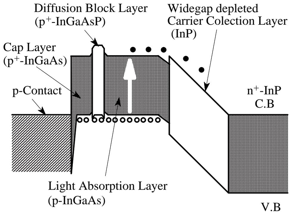
Fig. 1 Schematic energy band diagram of a UTC-PD.
