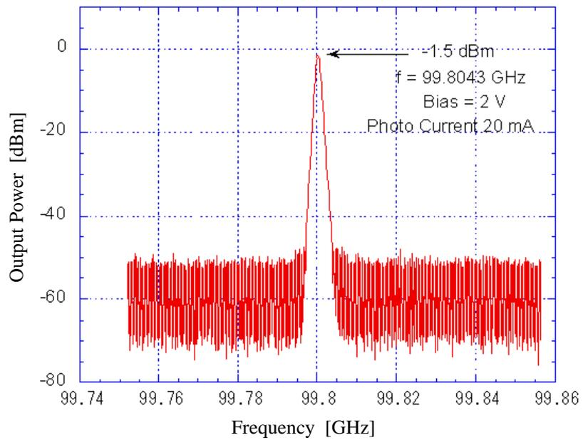
Fig. 8 Spectrum of photomixer output at  $\sim 100$  GHz.
