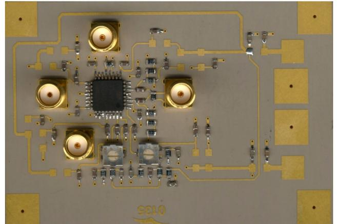
**Fig. 5.** Printed circuit board and 2-bit comparator ASIC used for laboratory tests
