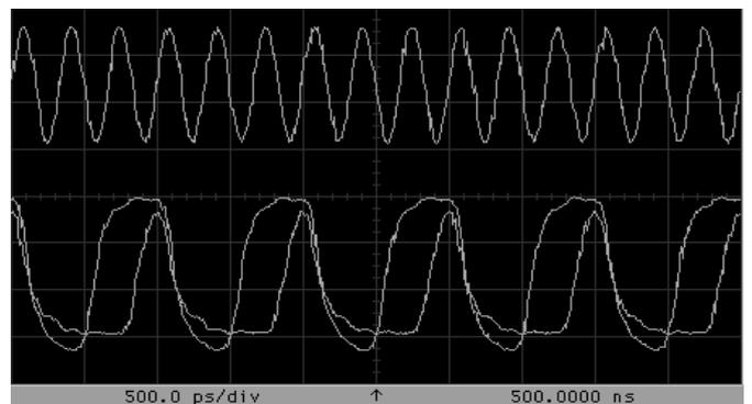
**Fig. 6.** Measured output waveform (lower plots) in response to 3 GHz input signal (upper plot) and 4 GHz clock
