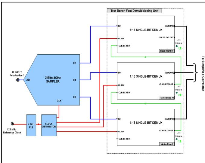
**Fig. 7.** Fast Demultiplexing Unit (FDU) block diagram for the digitizer test equipment
