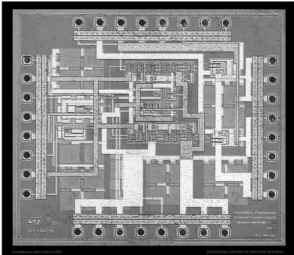
**Fig. 4.** Microphotograph of our first SiGe, 2-bit digitizer ASIC
