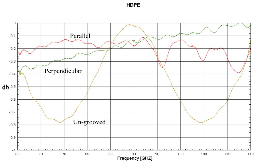
**Figure 9.** Transmission of un-grooved (yellow) and linearly-grooved HDPE (both 3.16 mm thick) parallel (red) and perpendicular (green) to the E-plane.
