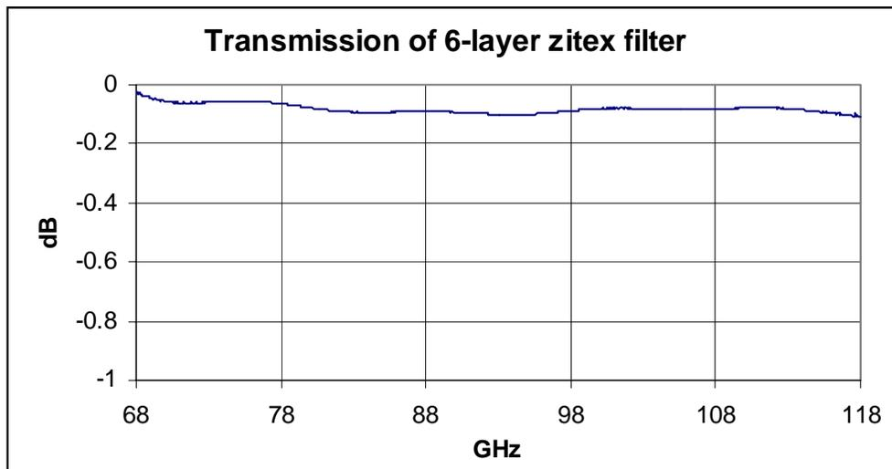
**Figure 5.** Measured transmission of 6-layer filter at room temperature.
