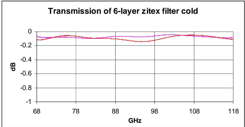
**Figure 6.** Measurement of transmission of 6-layer filter after repeated immersion in liquid nitrogen.
