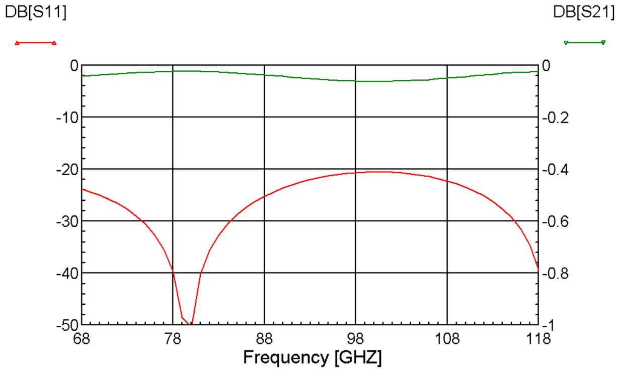
**Figure 4.** MMICAD calculation (transmission-green, reflection-red) for an optimized 6-layer IR filter. 203-micron thick Zitex G108 with 380-micron gaps, refractive index 1.2, loss 0.2 dB/cm.
