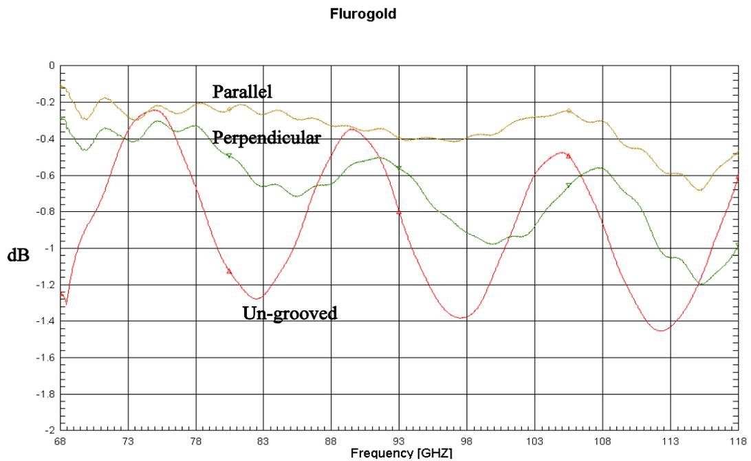
**Figure 8.** Transmission of linearly-grooved Flurogold (6.22 mm thick) for grooves parallel to the E-field (yellow) and perpendicular to the E-field (green). The red curve is for an un-grooved piece of Flurogold (6.22 mm thick).
