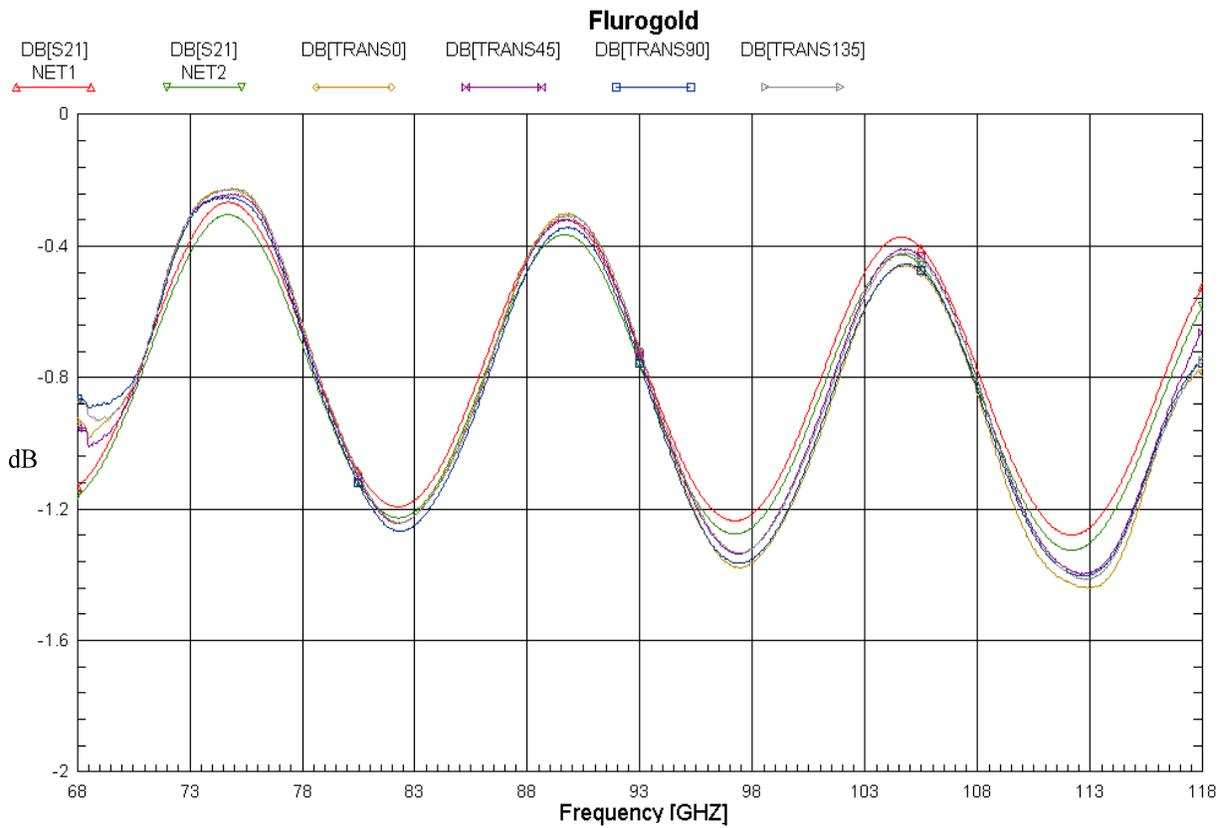
**Figure 7.** Transmission of a 6.22-mm thick piece of un-grooved Flurogold for rotation angles 0 (yellow), 45 (blue), 90 (purple), 135 (grey) degrees. Net1 (red) and Net2 (green) are MMICAD calculations for losses of 0.46 and 0.53 dB/cm, respectively.
