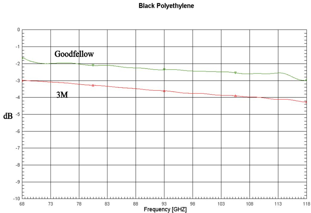
**Figure 1.** Transmission of 90-micron thick 3M (red) and Goodfellow (green) black polyethylene.
