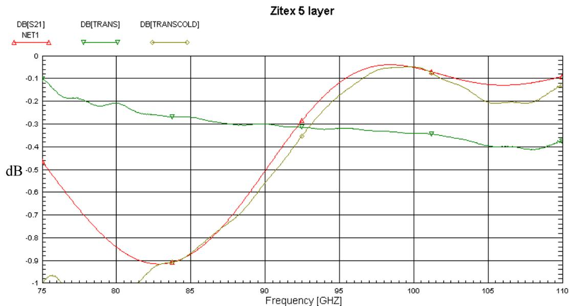
**Figure 3.** Measured transmission of a 5-layer Zitex IR filter (254-micron thick Zitex G110 with 1.575-mm gaps) at 300 K (green) and 77 K (yellow). Net1 (red curve) is the MMICAD prediction for the 5-layer filter of the same dimensions and loss of 0.2 dB/cm. The difference between the measured and the calculated performance below 83 GHz is probably an alignment problem.
