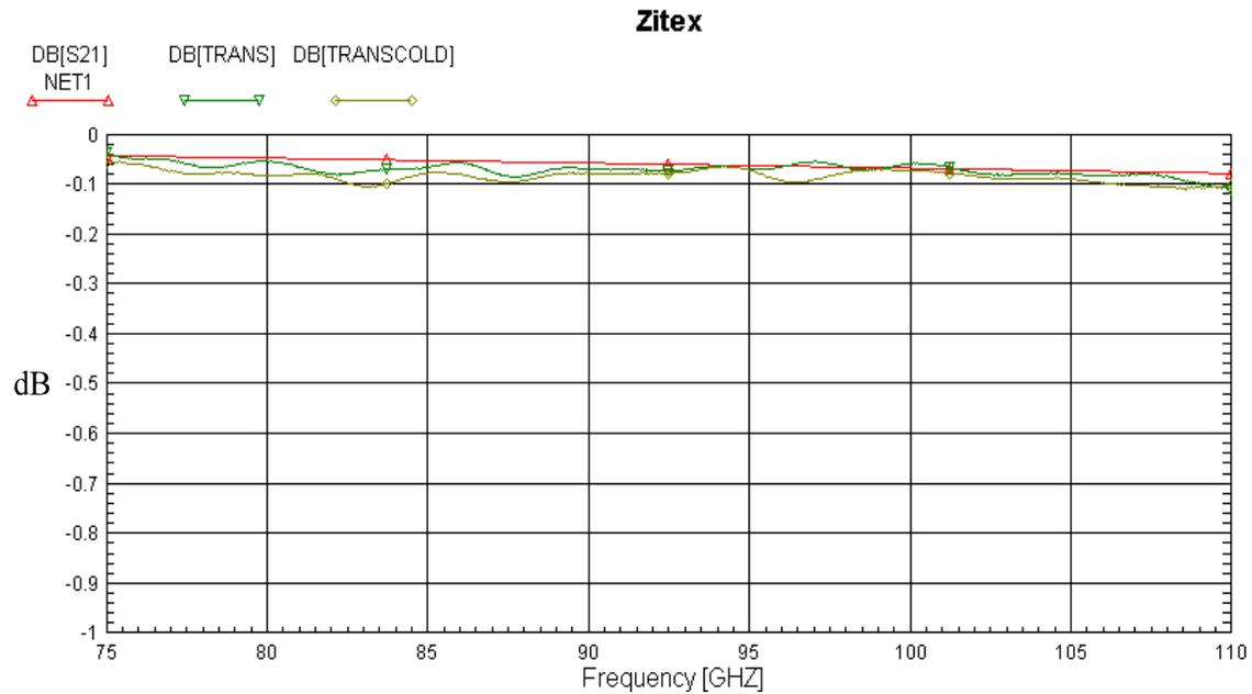
**Figure 2.** Transmission of free-standing Zitex G110 (254-microns thick) at 300 K (green) and 77 K (yellow). Net1 (red line) is the MMICAD curve for a material of the same thickness and refractive index.
