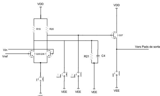
Fig. 7. Schematic of the output buffer
