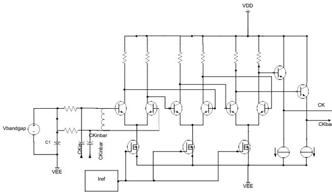
Fig. 10. Schematic of clock amplifier
