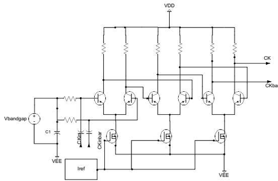
Fig. 6. Schematic of clock distributor circuit
