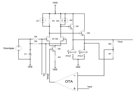
Fig. 2. Schematic of the input adapter amplifier
