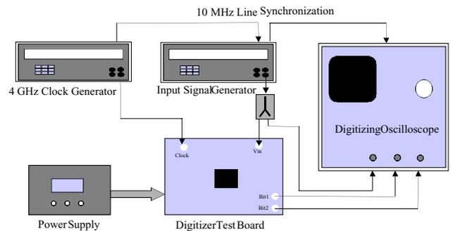
Fig. 12. Two-bit digitizer test bench
