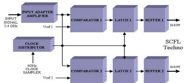
Fig. 1. Two-bit digitizer circuit configuration
