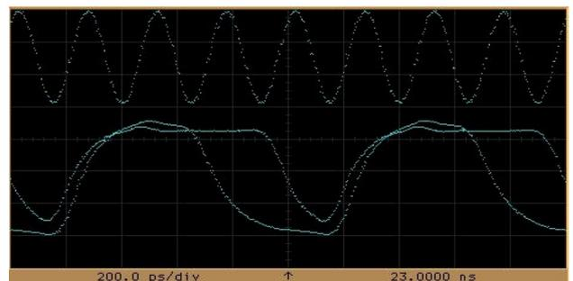
Fig. 15. Measured output waveforms (lower plots) in response to 3 GHz input signal for a 4 GHz sampling clock
