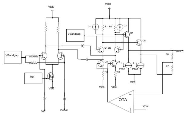
Fig. 9. Schematic of the input adapter amplifier
