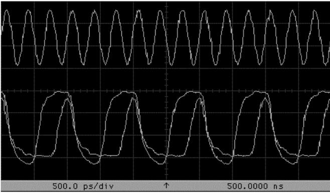
Fig. 13. Measured output waveforms (lower plots) in response to a 3 GHz input signal (upper plot); the digitizer clock is at 4 GHz
