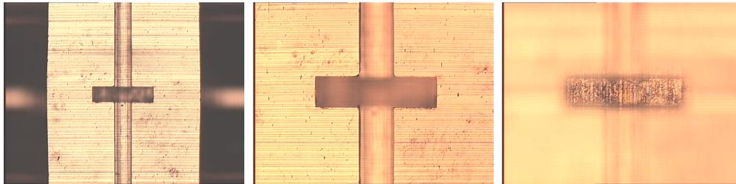
*Figure 9: The small series of backpieces and photographs demonstrating the cavity quality. The middle and the right photographs at the bottom series are focused on the top and bottom of the cavity, respectively.*
