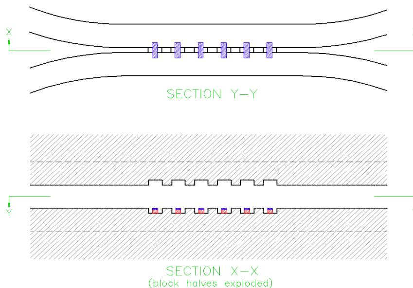
**Fig. 1.** Diagram of the split-block coupler with six coupling probes (blue) on quartz standoffs (red). In the lower view, the two block halves are shown separated for clarity.
