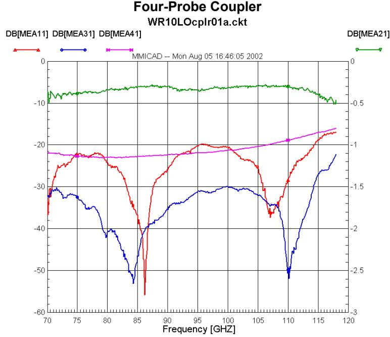
**Fig. 3. Measured S-parameters of the WR-10 directional coupler with four probes. Left scale: — S11 dB, — S31 dB, — S41 dB. Right scale: — S21 dB. (The WR-10 band is indicated by the markers at 75 and 110 GHz.)**
