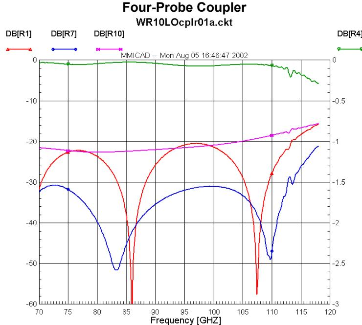
**Fig. 4. Results of the QuickWave simulation of the four-probe coupler. Left scale: — S11 dB, — S31 dB, — S41 dB. Right scale: — S21 dB. (The WR-10 band is indicated by the markers at 75 and 110 GHz.)**
