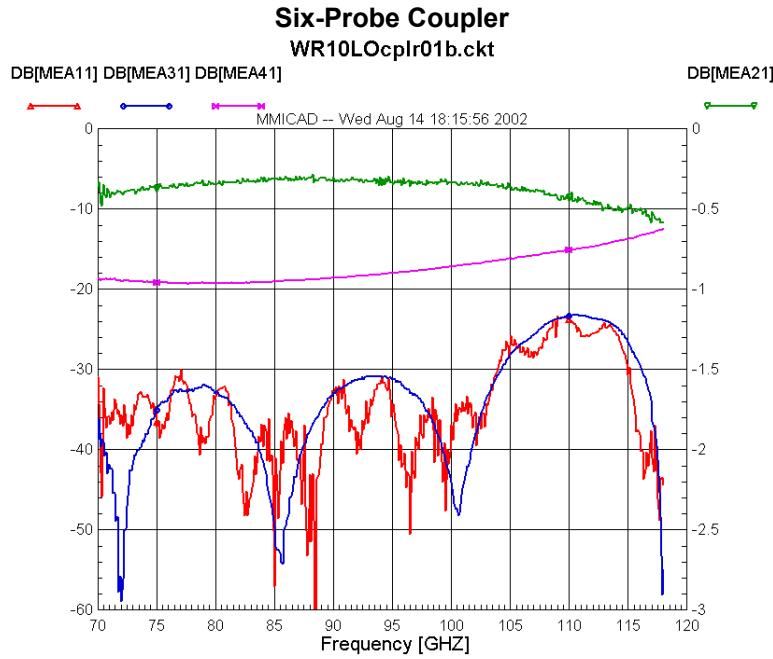
**Fig. 5.** Measured S-parameters of the WR-10 directional coupler with six probes. Left scale: — S11 dB, — S31 dB, — S41 dB. Right scale: — S21 dB. (The WR-10 band is indicated by the markers at 75 and 110 GHz.)
