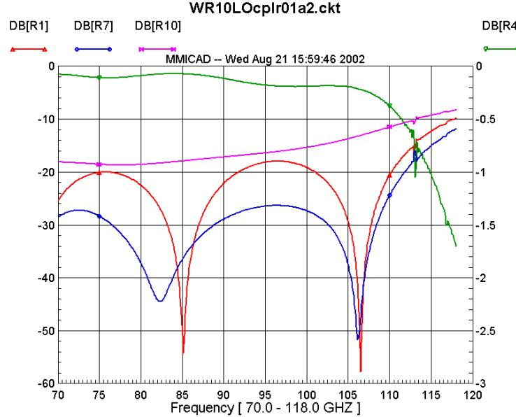
**Fig. 8. Results of the QuickWave simulation of the four-probe coupler with all probes increased in length by 0.004". (Compare with Fig. 4.)** Left scale: — S11 dB, — S31 dB, — S41 dB. Right scale: — S21 dB. (The WR-10 band is indicated by the markers at 75 and 110 GHz.)
