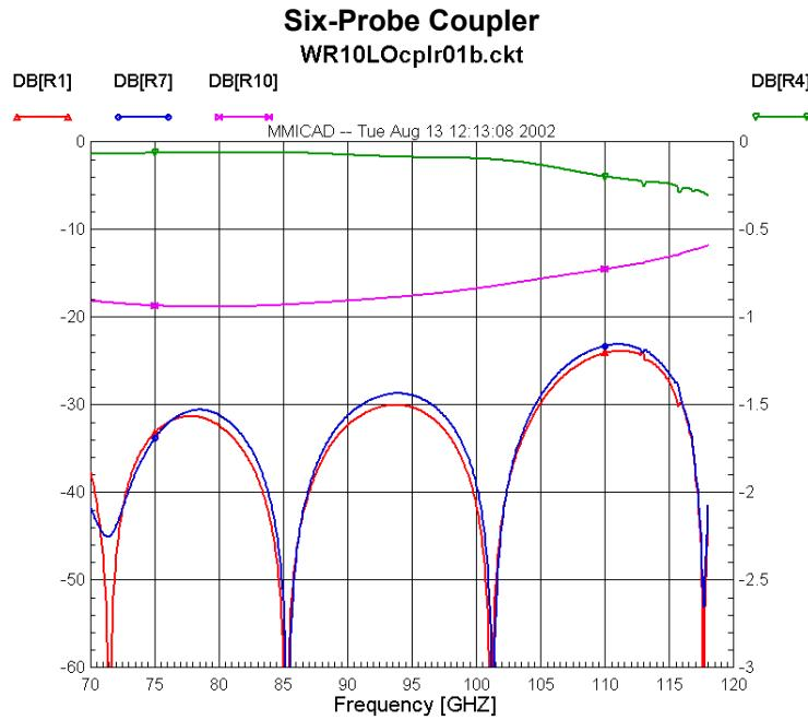
**Fig. 6.** Results of the QuickWave simulation of the six-probe coupler. Left scale: — S11 dB, — S31 dB, — S41 dB. Right scale: — S21 dB. (The WR-10 band is indicated by the markers at 75 and 110 GHz.)
