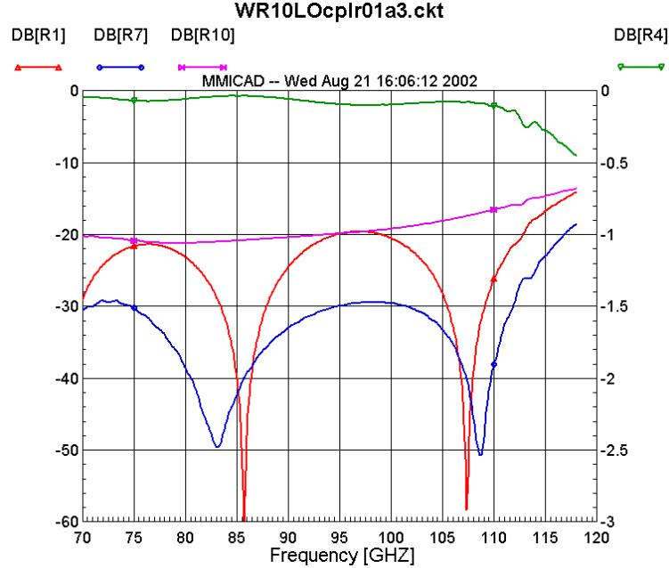
**Fig. 9. Results of the QuickWave simulation of the four-probe coupler with the thickness of all probes increased from 0.0016" to 0.0032". (Compare with Fig. 4.) Left scale: — S11 dB, — S31 dB, — S41 dB. Right scale: — S21 dB. (The WR-10 band is indicated by the markers at 75 and 110 GHz.)**
