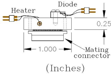
Figure 4. A test block to evaluate the thermal performance of the heat sinks.
