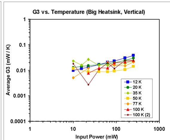
Figure 11. G3 for the big heat sink mounted vertically.
