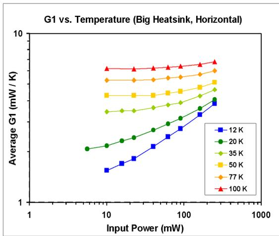
Figure 6. G1 for the big heat sink mounted horizontally.
