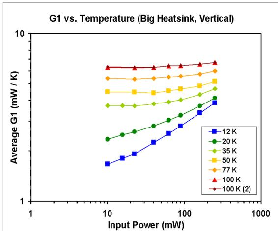
Figure 10. G1 for the big heat sink mounted vertically.
