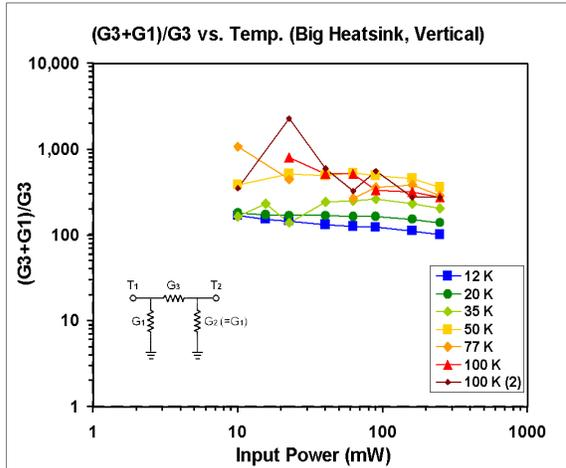
Figure 12. “Figure of merit” for the big heat sink mounted vertically.
