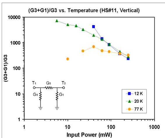
Figure B11. "Figure of merit" for heat sink #11 mounted vertically.
