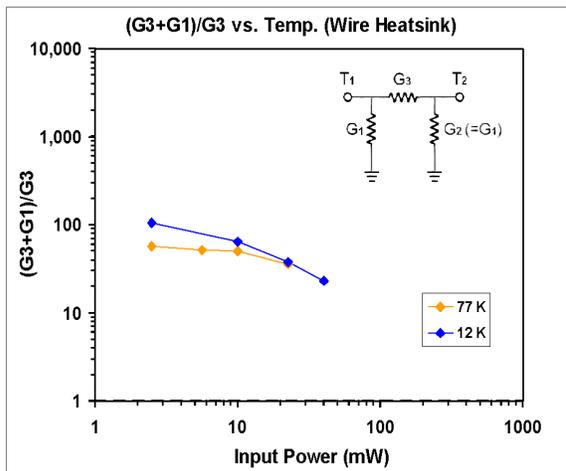
Figure B16. "Figure of merit" for the wire heat sink.
