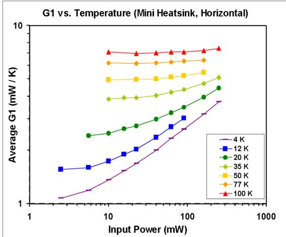
Figure 14. G1 for the mini heat sink mounted horizontally.
