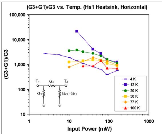
Figure B3. "Figure of merit" for the original heat sink mounted horizontally.
