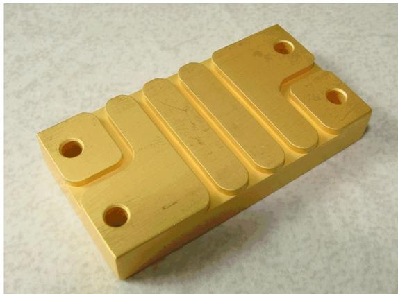
Figure B13. A heat sink block used to clamp down 12 pairs of phosphor bronze wire with Apiezon N high-conductivity vacuum grease<sup>1</sup>.
