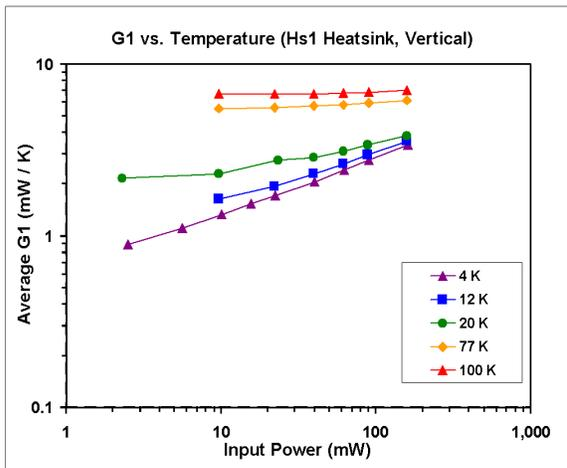
Figure B5. "Figure of merit" for the original heat sink mounted vertically.
