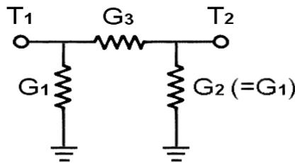
Figure 5. A two-port thermal model for the heat sink.
