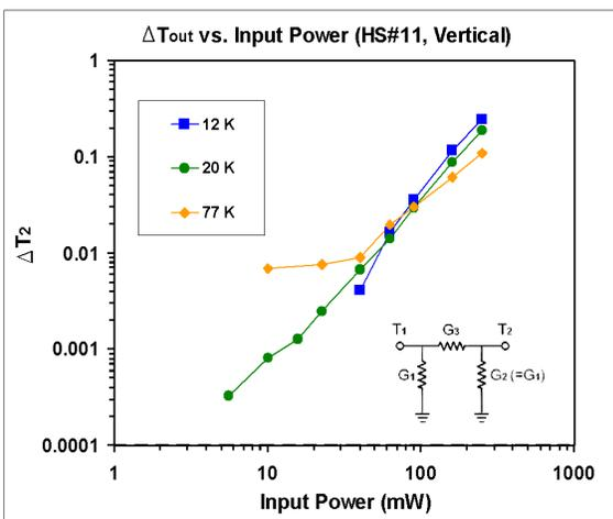
Figure B12. Output temperature rise vs. input power for heat sink #11 mounted vertically.
