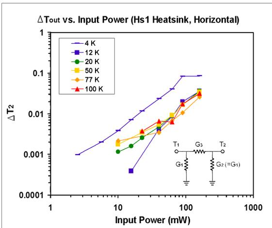
Figure B4. Output temperature rise vs. input power for the original heat sink, horizontal.
