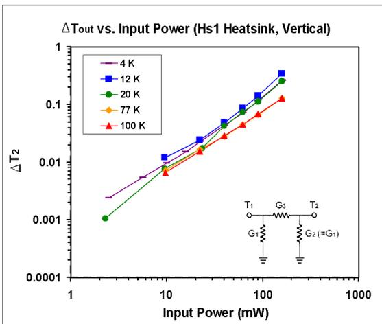
Figure B8. Output temperature rise vs. input power for the original heat sink, vertical.
