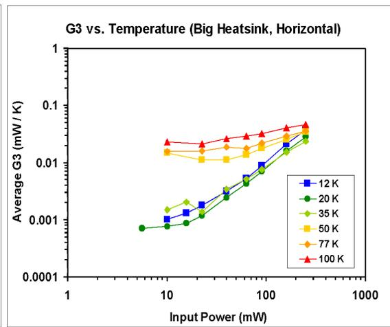
Figure 7. G3 for the big heat sink mounted horizontally.
