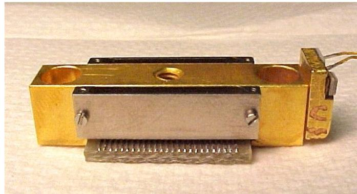
Figure 3. A miniature version of the larger heat sink.
