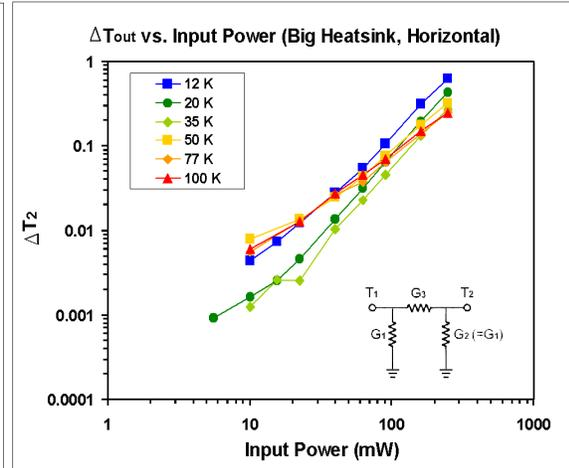
Figure 9. Output temperature rise vs. input power for the big heat sink, horizontal.
