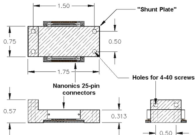
Figure 1. Design of a modular heat sink with Nanonics connectors. Dimensions are in inches.
