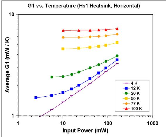
Figure B1. G1 for the original heat sink, horizontal.
