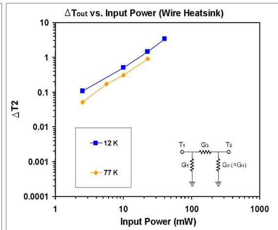
Figure B17. Output temperature rise vs. input power for the wire heat sink.
