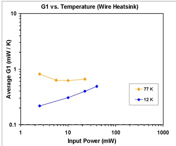
Figure B14. G1 for the wire heat sink.
