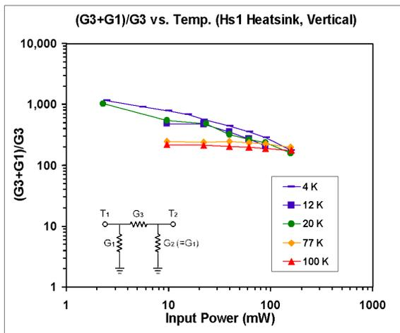
Figure B7. G3 for the original heat sink, vertical.
