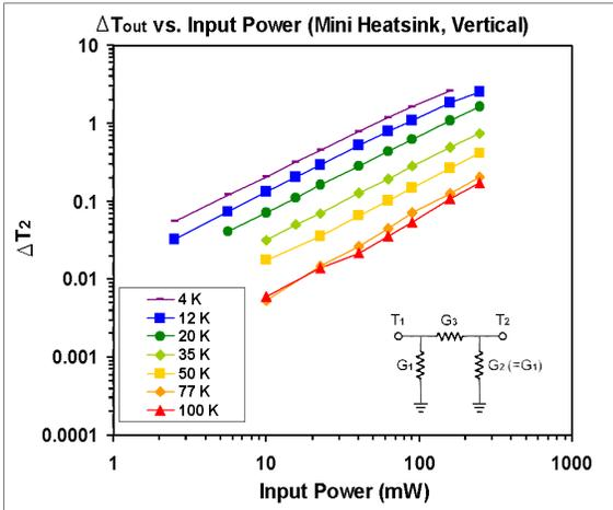
Figure 21. Output temperature rise vs. input power for the mini heat sink, vertical.
