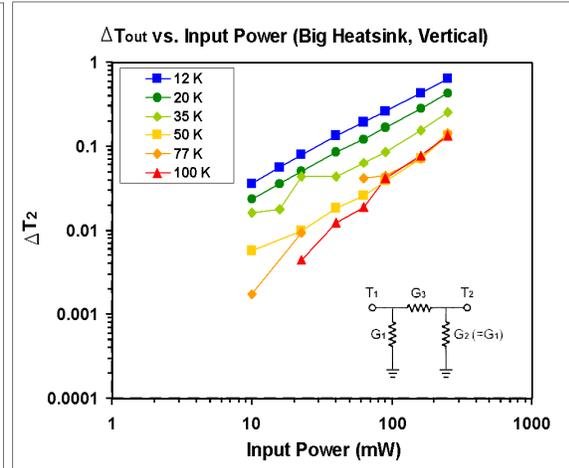
Figure 13. Output temperature rise vs. input power for the big heat sink, vertical.
