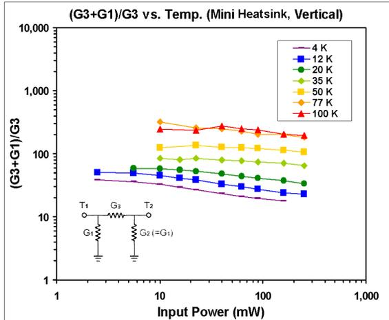
Figure 20. “Figure of merit” for the mini heat sink mounted vertically.
