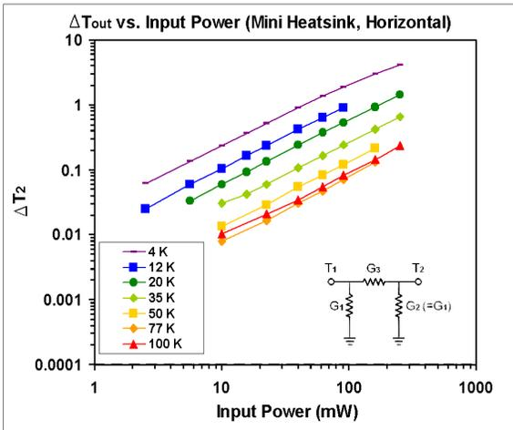
Figure 17. Output temperature rise vs. input power for the mini heat sink, horizontal.
