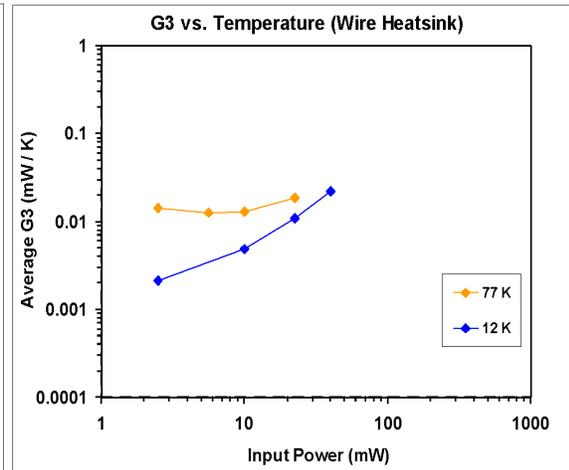
Figure B15. G3 for the wire heat sink.
