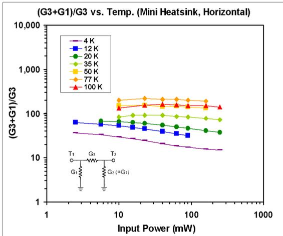
Figure 16. “Figure of merit” for the mini heat sink mounted horizontally.
