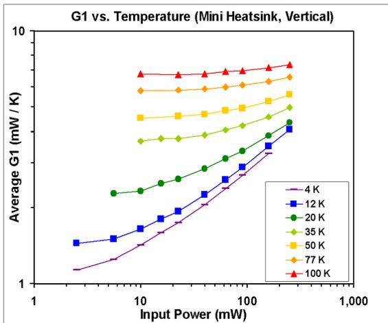
Figure 18. G1 for the mini heat sink mounted vertically.
