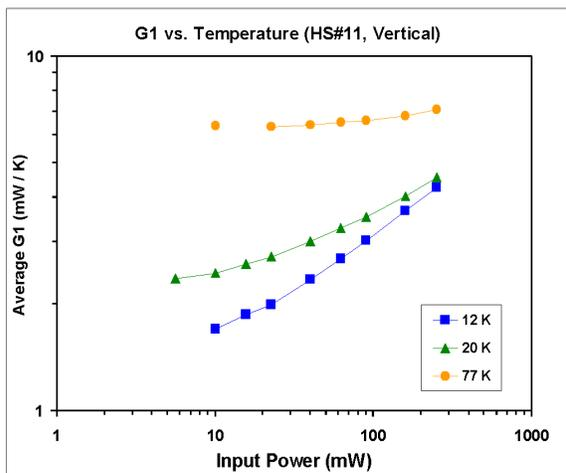
Figure B9. G1 for heat sink #11, vertical.
