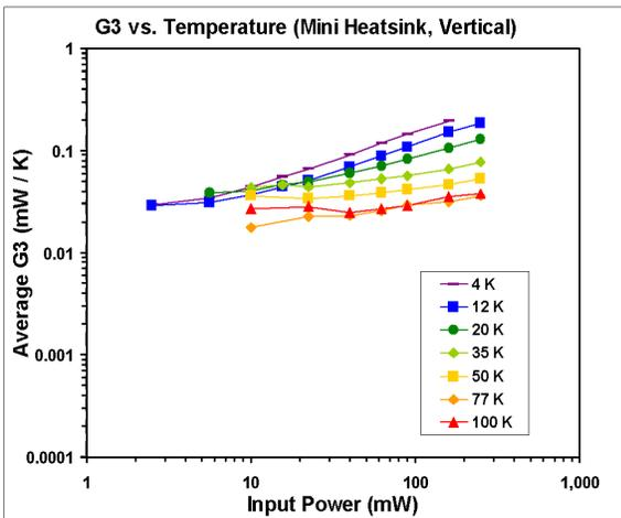
Figure 19. G3 for the mini heat sink mounted vertically.
