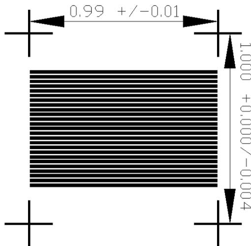
Figure A1. Printed circuit board layout for the large heat sink. Dimensions are in inches.
