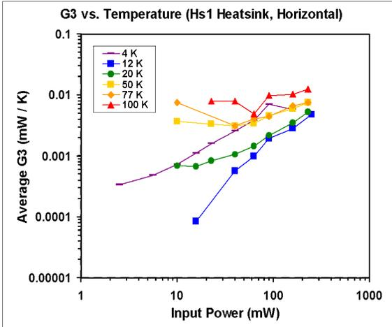
Figure B2. G3 for the original heat sink, horizontal.
