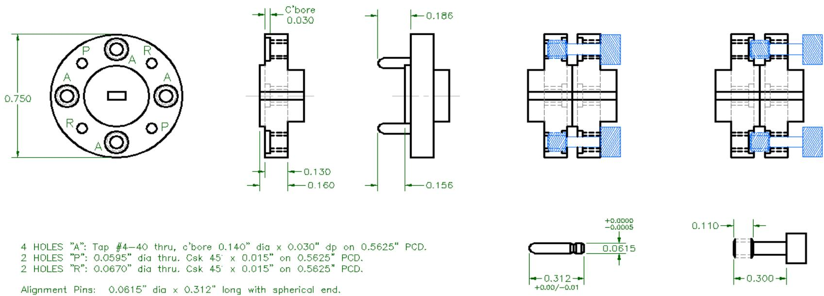
Fig. 1 The standard Mil-F-3922/67B flange with its raised central boss. The right hand diagrams show a pair of flanges engaged with the screws inserted and withdrawn.
