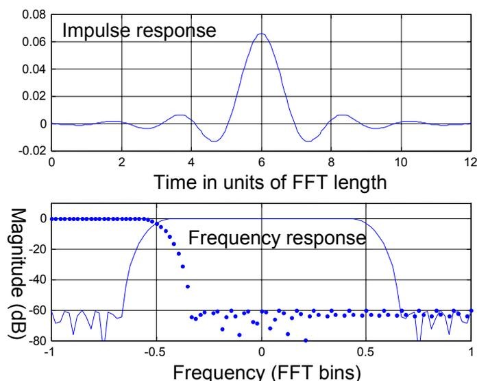
**Figure 2 Example of a prototype filter impulse response and the resulting channel response for a polyphase filterbank. Also shown in the lower plot is the channel response of an adjacent channel (dotted) for a polyphase filterbank implemented with the topology shown in Figure 1.**
