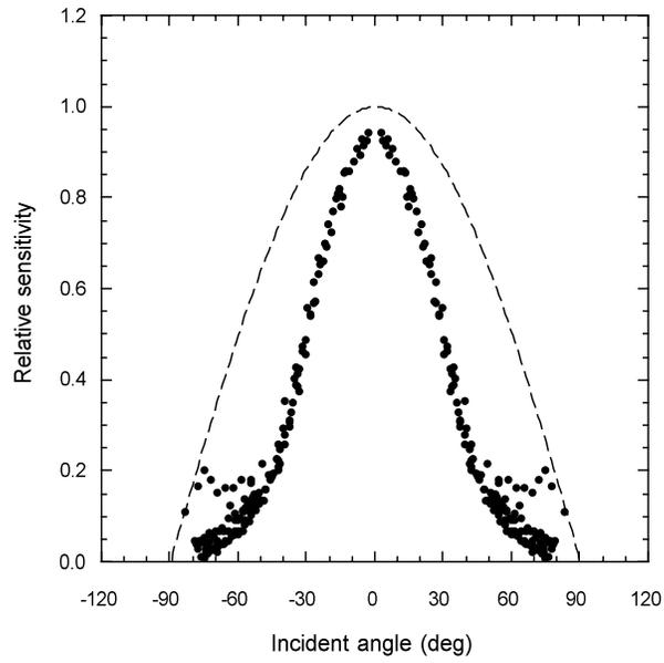
Figure 5: Incident angle dependence of the UVD-365PD sensor measured toward the Sun. Dashed line corresponds to the cosine response.
