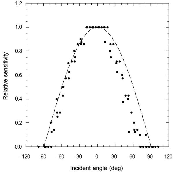
Figure 8: Measured incident angle dependence of SafeSun. Dashed line corresponds to the cosine response. Incident angle is positive toward the foreside of the observer.
