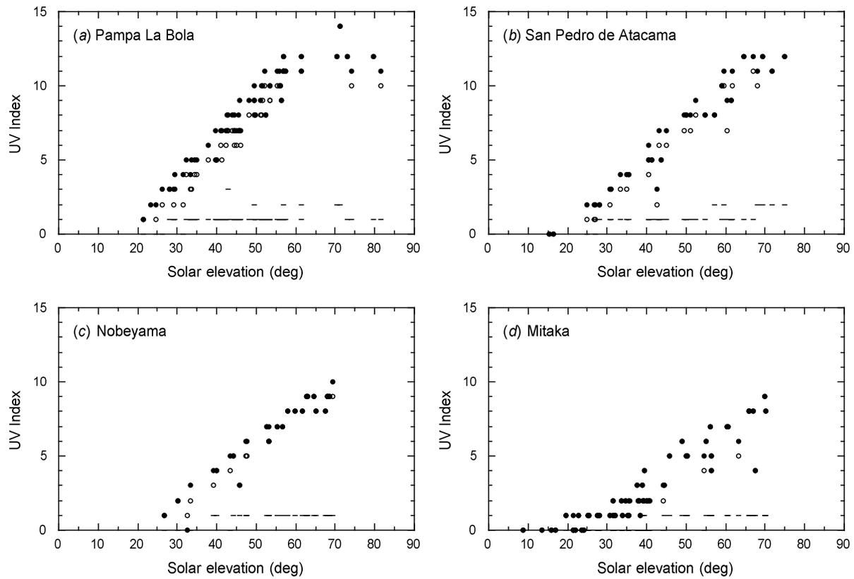
Figure 7: Solar elevation dependence of UV Index, which chiefly reflects UVB intensity, toward three positions of the sky — toward the Sun ( $I_{\text{sun}}^+$ ; *filled circles*), toward the zenith ( $I_{\text{zen}}^+$ ; *open circles*), and toward the horizon in the opposite direction to the Sun ( $I_{\text{hor}}^+$ ; *dashes*) — measured at (a) Pampa La Bola, (b) San Pedro de Atacama, (c) Nobeyama, and (d) Mitaka.
