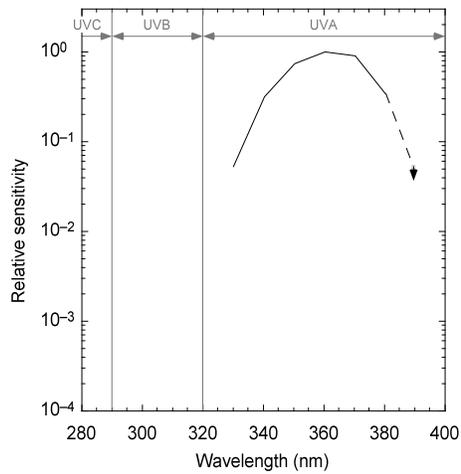
Figure 1: Typical relative spectral sensitivity of Ushio UVD-365PD sensor (Ushio Inc. 2001, private communication).
