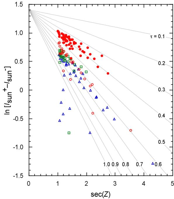
Figure 6: Airmass dependence of the UVA intensity toward the Sun, measured at Pampa La Bola (*red filled circles*), San Pedro de Atacama (*red open circles*), Socorro AOC (*blue filled squares*), Nobeyama (*green open squares*), and Mitaka (*blue open triangles*), subtracted for uniform component. Thin lines indicate extinction curves with an intersection at  $\ln(I_{\text{sun}}^+ - I_{\text{sun}}^-) = 1.4$ .
