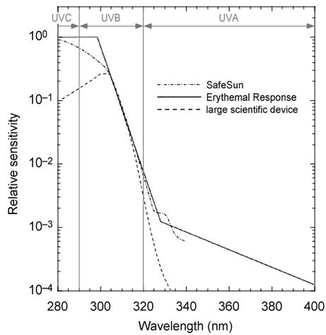
Figure 2: Relative spectral sensitivities (normalized at 310 nm) of SafeSun Classic personal UV radiometer (*dot-dash line*) and a large scientific device widely used for laboratory/meteorological measurements (*dashed line*) overlaid on the Erythral Response Spectrum pattern (*solid line*) [6].
