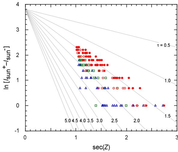
Figure 9: Airmass dependence of the UV Index, which chiefly reflects UVB intensity, toward the Sun, measured at Pampa La Bola (*red filled circles*), San Pedro de Atacama (*red open circles*), Nobeyama (*green open squares*), and Mitaka (*blue open triangles*), subtracted for uniform component. Thin lines indicate extinction curves with an intersection at  $\ln(I_{\text{sun}}^+ - I_{\text{sun}}^-) = 3.8$ .
